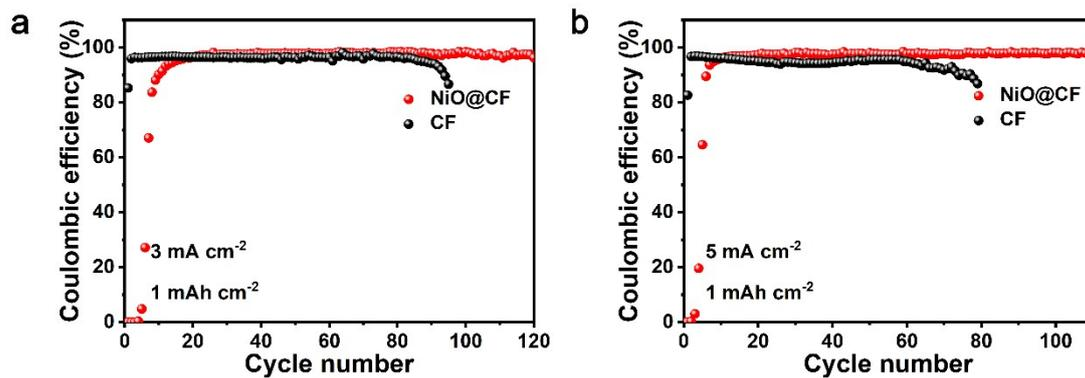
**Fig. S8** Coulombic efficiencies comparison of Li || CF and Li || NiO@CF cells tested at a constant deposition capacity of 1 mAh cm<sup>-2</sup> with different current densities, (a) 3 mA cm<sup>-2</sup>, (b) 5 mA cm<sup>-2</sup>
