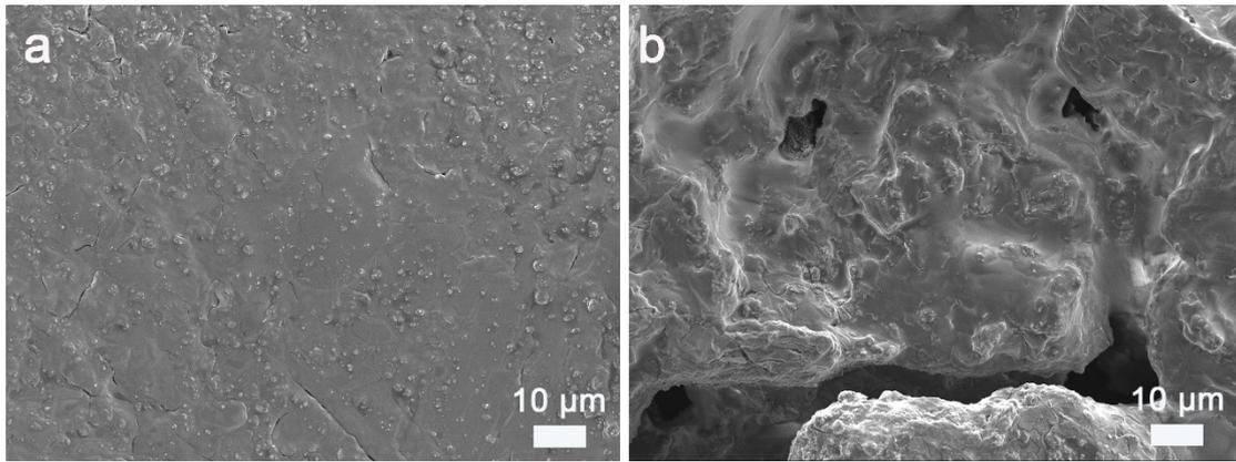
**Fig. S11** SEM images of (a) Li/NiO@CF || LFP and (b) Li/CF || LFP full batteries at the anode after cycling 200<sup>th</sup> at 3 C
