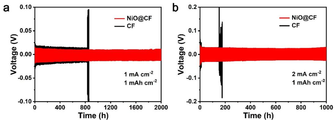
**Fig. S9** Electrochemical performance of Li || NiO@CF || Li and bare Li || CF || Li cells tested at different current densities (a) 1 mA cm<sup>-2</sup>, (b) 2 mA cm<sup>-2</sup> with a constant areal capacity of 1 mAh cm<sup>-2</sup>
