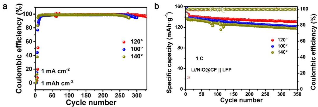
**Fig. S7** (a) The coulombic efficiencies of Li || NiO@CF cells, (b) cycling performance of Li/NiO@CF || LFP full battery for NiO@CF electrodes derived from different hydrothermal temperatures
