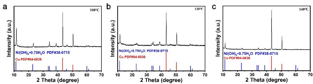
**Fig. S5** XRD patterns of Ni(OH)<sub>2</sub>·0.75H<sub>2</sub>O/Cu foam composites prepared at different hydrothermal temperatures, (a) 100 °C, (b) 120 °C, (c) 140 °C
