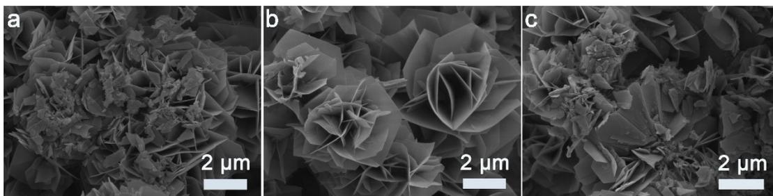
**Fig. S6** SEM images of  $\text{Ni(OH)}_2 \cdot 0.75\text{H}_2\text{O}$  prepared at different hydrothermal temperatures, (a) 100 °C, (b) 120 °C, (c) 140 °C
