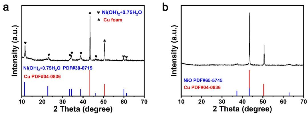
**Fig. S2** XRD patterns of (a) Ni(OH)<sub>2</sub>·0.75H<sub>2</sub>O@CF, (b) NiO@CF
