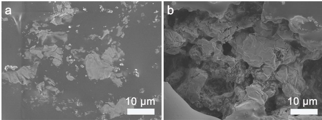
**Fig. S10** SEM images of symmetric cells based on NiO@CF and CF anode after cycling 300 h at current density of  $10 \text{ mA cm}^{-2}$ , with depositing capacity of  $10 \text{ mAh cm}^{-2}$ , respectively. (a) NiO@CF electrode, (b) CF electrode
