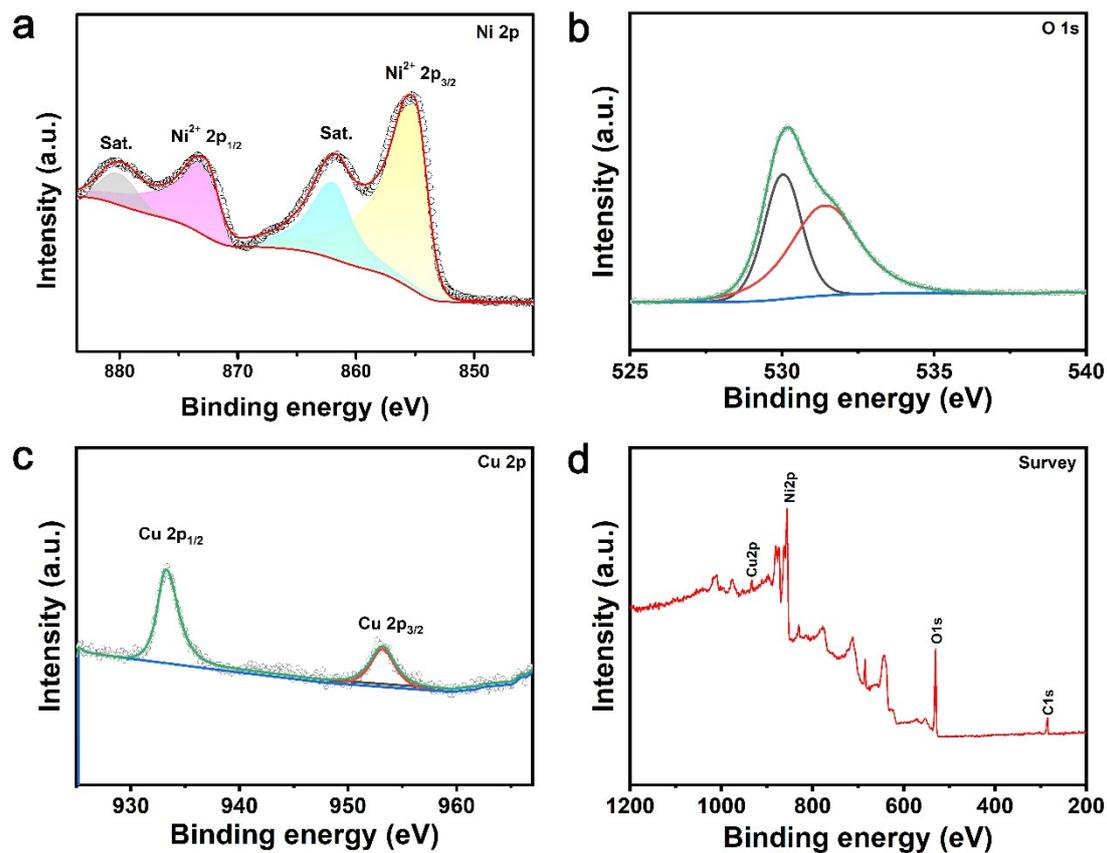
**Fig. S4** XPS spectra of NiO@CF. The high-resolution XPS spectrum of (a) Ni 2p, (b) O 1s, (c) Cu 2p, (d) XPS survey spectrum
