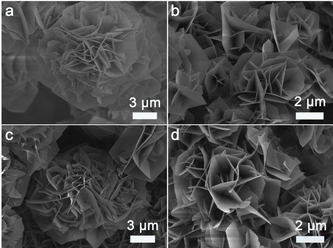
**Fig. S1** SEM images after hydrothermal treatment, (a) low magnification, (b) high magnification; SEM images after annealing treatment, (c) low magnification, (d) high magnification
