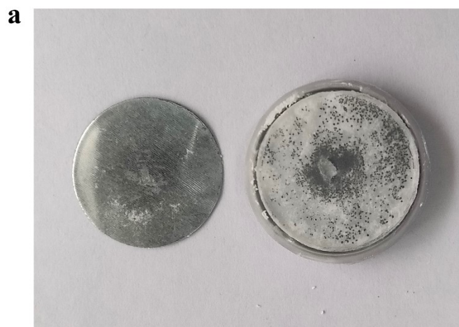
Figure S9. Photographs of (a) bare Zn and (b) \delta\text{-MnO}_2\text{/Zn} electrodes after 10 cycles at 3\text{ mA cm}^{-2} and 1.5\text{ mAh cm}^{-2} .
