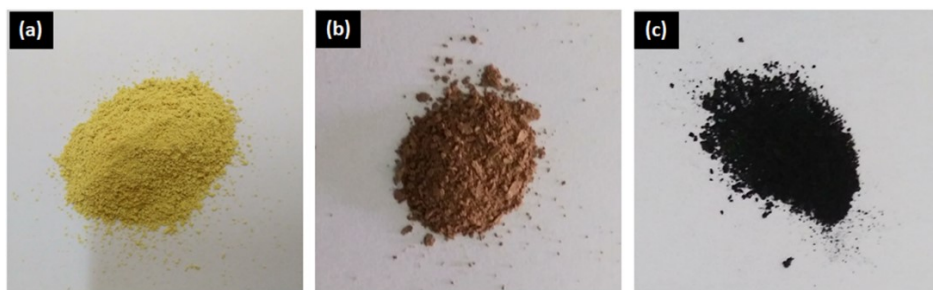
Figure S1. Photographic images of (a) SgCN, (b) CF/SgCN and (c) SeCF-MMO/ SgCN:MX powder.
