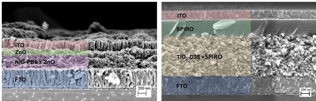
**Figure S5:** SEM cross-section pictures of (left) n-ssDSC and (right) p-ssDSC.
