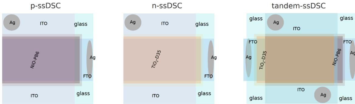
**Figure S1:** Device structure of p-ssDSC, n-ssDSC and resulting tandem device.
