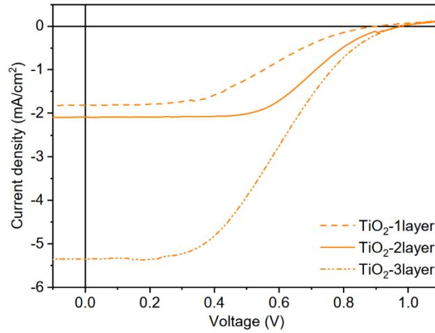
**Figure S3:** *J-V* curves of n-ssDSCs fabricated with 1, 2 and 3 layers of TiO<sub>2</sub>, illuminated from the ITO, without PB6 cover.
