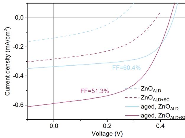
**Figure S2:** *J-V* curves of p-ssDSC with just an ALD layer of ZnO and an extra layer of solution processed ZnO from Zn(acac)<sub>2</sub> solution, both directly after fabrication and after aging for 8 weeks.
