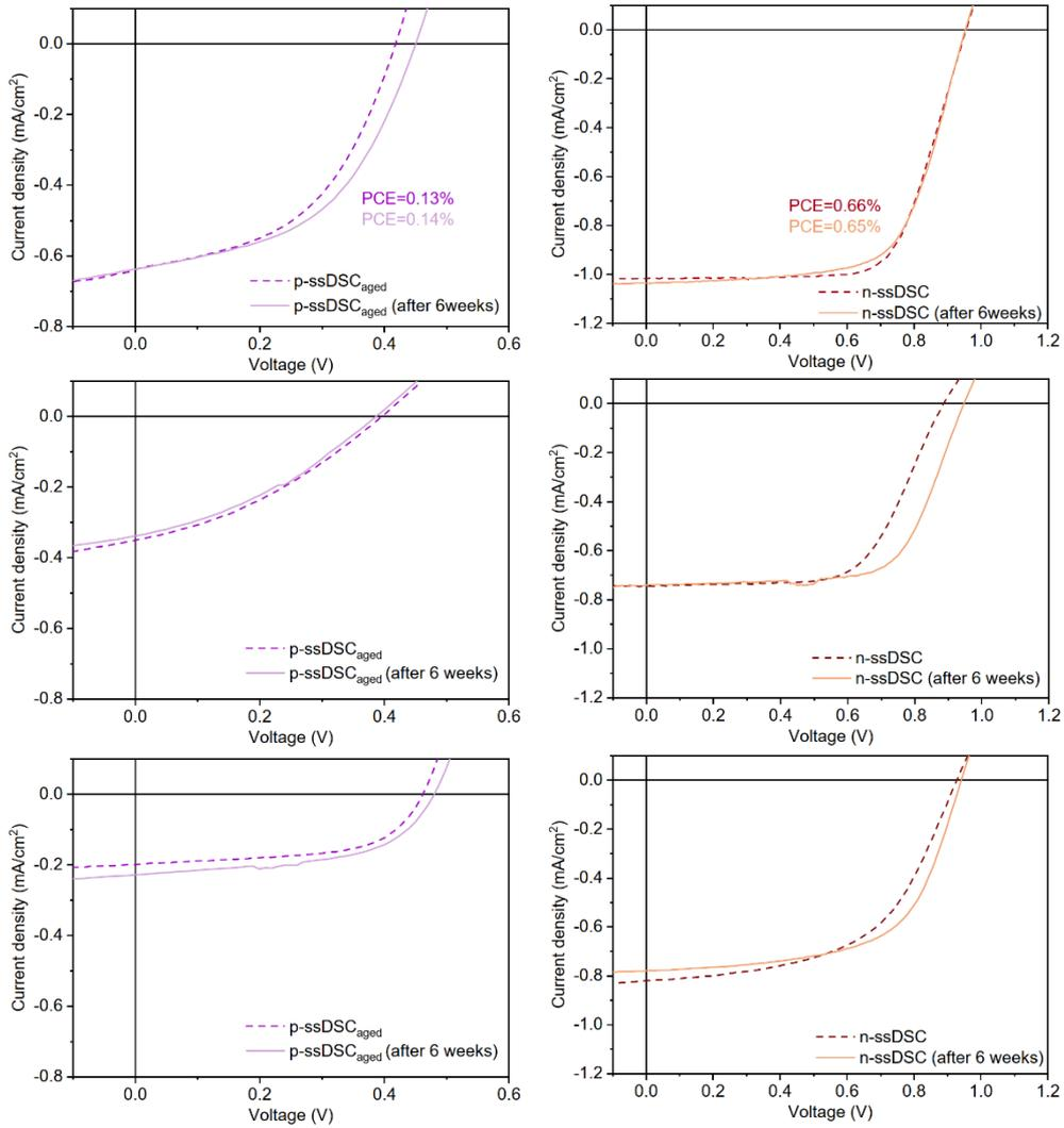
**Figure S8:** J-V curves of three p-ssDSC (left) and p-ssDSC films (right) from Fig. 5 in the main text after storage in ambient conditions for 6 weeks. Note that the p-ssDSC is already aged at the starting point and that p-ssDSC is measured by illumination from the FTO side and that the n-ssDSC was shaded by a p-ssDSC during the measurement.
