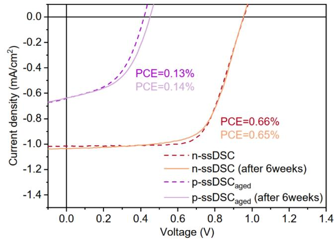
**Figure S7:** *J-V* curves of two ss-DSCs from Fig. 5 in the main text after storage in ambient conditions for 6 weeks. Note that the p-ssDSC is already aged at the starting point and that p-ssDSC is measured by illumination from the FTO side and that the n-ssDSC was shaded by a p-ssDSC during the measurement.
