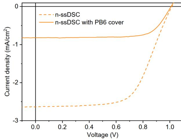
**Figure S4:** *J-V* curves of n-ssDSCs fabricated with 2 layers of TiO<sub>2</sub>, illuminated from the ITO side, with and without PB6 cover.
