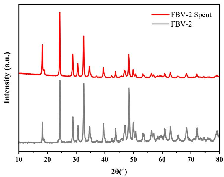
**Figure S2:** XRD of Fresh and spent FBV-2 for comparison
