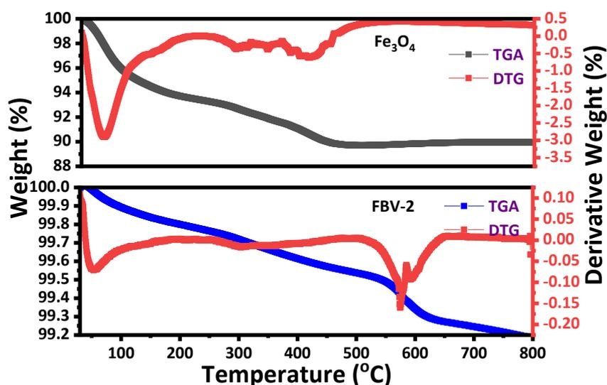
Figure S1: TG/DTA of photocatalyst  $\text{Fe}_3\text{O}_4$  and FBV-2
