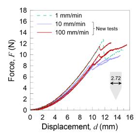
Finally, to further explore the repeatability of results for penetration tests, the test for ED8 with 2R = 2.72 mm is performed three times at the penetration velocity of 1 mm/min. The plot reported below clearly shows a good consistency in the results.
