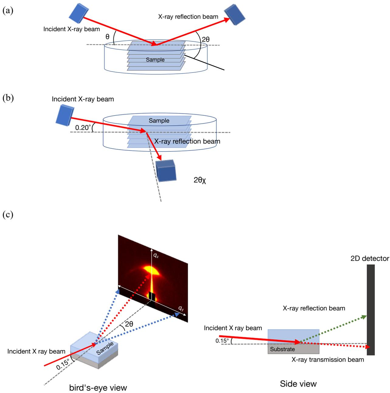
**Figure S4** Experimental geometry for (a) out-of-plane XRD, (b) in-plane XRD and (c) 2D GI-XRD.<sup>2</sup>
