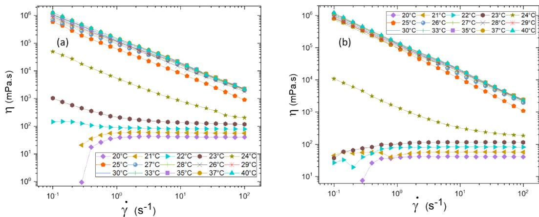
**Figure S8:** (a) and (b) are the flow curve with viscosity as a function for shear rate for 20%PF127 and composite systems with 0.1% nanorods. The sol-gel transition can be observed at 23°C for 20% PF127 and 24°C for the composite system with 0.1% nanorods. Solid lines are guided to the eyes.
