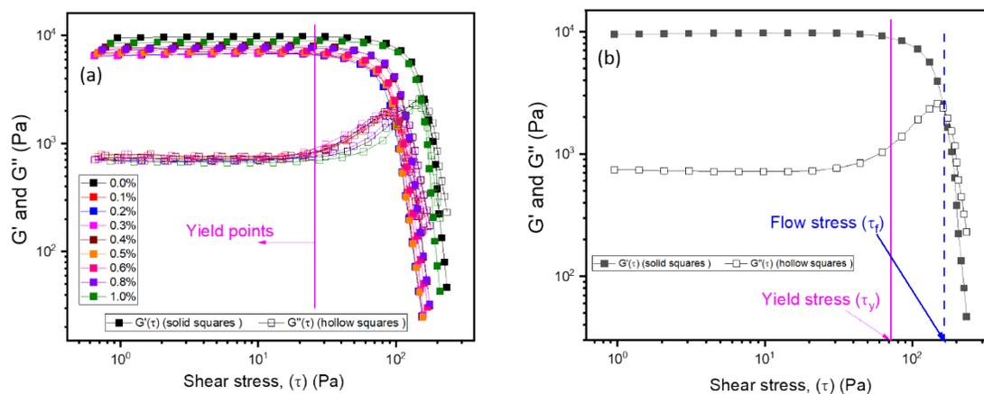
**Figure S11:** (a) Amplitude sweep data with storage modulus ( $G'$ ) and loss modulus ( $G''$ ) as a function of shear stress ( $\tau$ ) at a constant angular frequency ( $\omega = 10$  rad/s) for different concentrations at 30 °C for 20 % PF127 and for composites with different concentration of  $\beta$  - FeOOH nanorods (b) we defined yield stress ( $\tau_y$ ), flow stress ( $\tau_f$ ). Solid lines in both figures (a) and (b) are guided to the eye.
