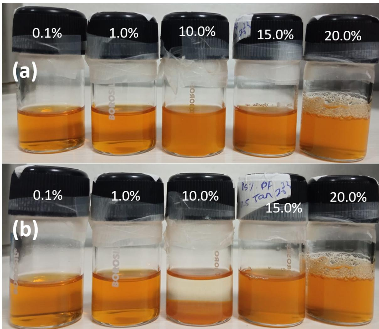
**Figure S6:** Visual observation of adsorption of PF127 on nanorods surface by observing sedimentation in the composite system for 0.1% (w/v) nanorods and with different concentration of PF127 (a) initial images and (b) is images taken after 25 minutes. The experiment is done at 25°C.
