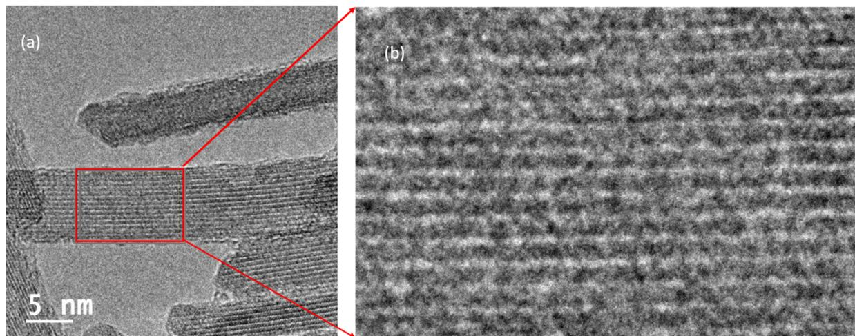
**Figure S1:** (a) Original HR-TEM image of nanorods with selected is highlighted the region in a red square where the d-spacing is supposed to be calculated (b) cropped area of figure (a)
