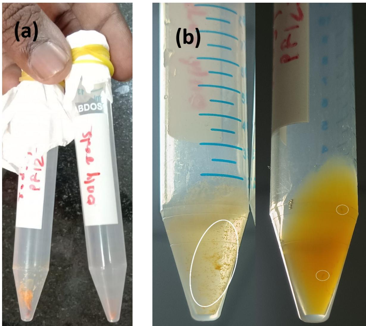
**Figure S5:** (a) Freeze-dried powder of 0.1% NRs and its composite with PF127 (PF127-NRs) and (b) Re-dispersion of NRs and PF127-NRs in DI water. It can be noted that for both NRs and PF127-NRs composite system cannot redisperse in DI water due to strong hydrophilic interaction and the particle forms aggregates (white circle) seen in Figure b. This can be indication of PF127 get adsorbed on surface of  $\beta$ -FeOOH NRs.
