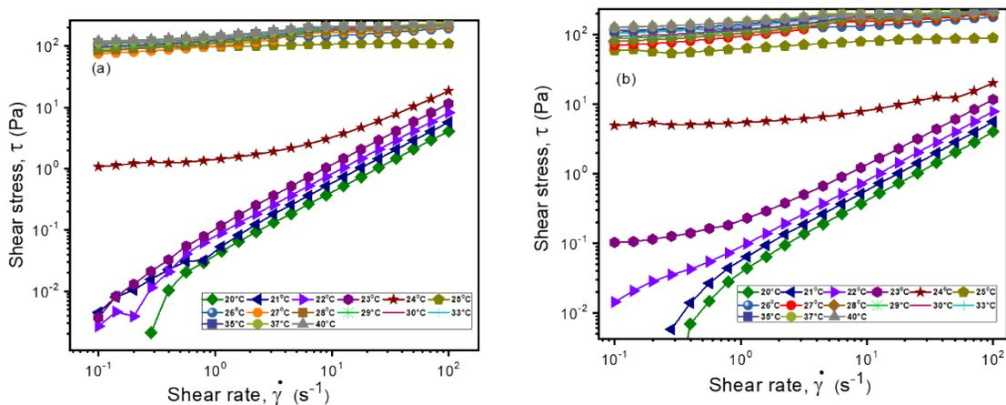
**Figure S7:** (a) and (b) are the flow curve with shear stress as a function of shear rate for 20%PF127 and composite systems with 0.1% nanorods. Both figures show the clear transition from liquid phase to a gel-like state. Solid lines are guided to the eyes.
