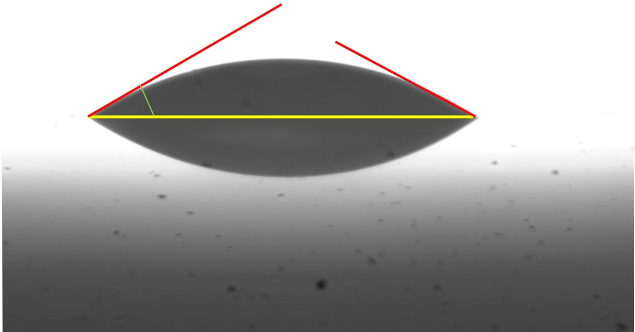
**Figure S4:** The contact angle measurement is done by placing a water droplet on a  $\beta$ -FeOOH NRs film. The left side and right side angle values are 36.03 ° and 34.65 °, which represents the hydrophilic nature of the  $\beta$ -FeOOH NRs film.
