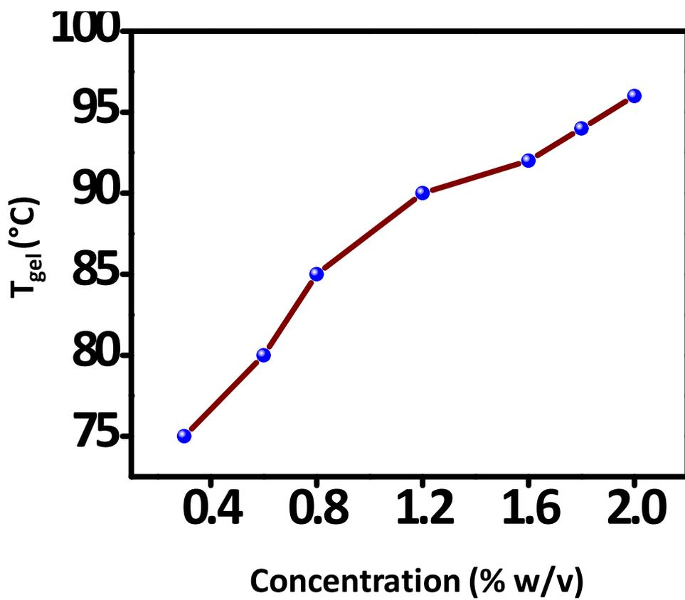
**Fig. S5.** Variation of  $T_{gel}$  with increasing concentration of the gelators **A** and **B** for 1:1 hydrogel.
