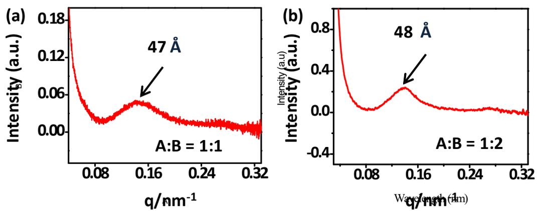
Fig. S7. SAXS data obtained from the (a)1:1 and (b)1:2 hydrogels.
