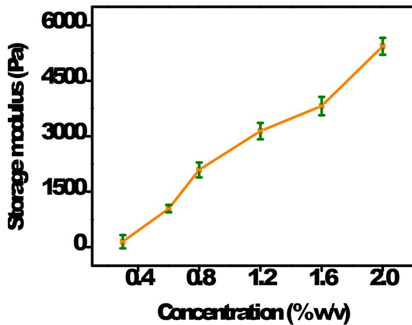
**Fig. S4.** Variation of storage modulus with increasing concentration of the gelators A and B for 1:1 hydrogel.
