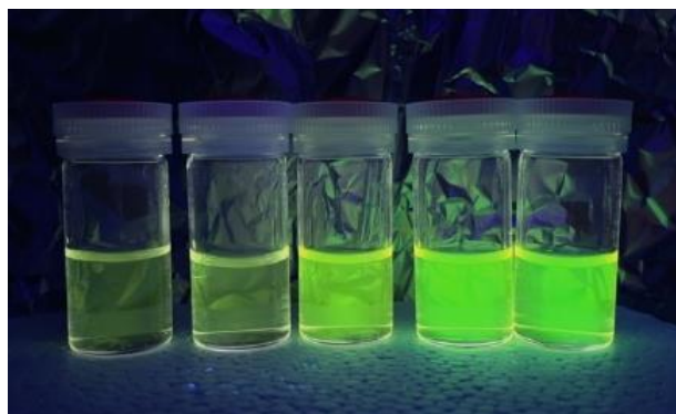
Figure S3. Photographs of fluorescence of FL in buffer solutions. (From left to right, pH 2.0, pH 3.0, pH 5.8, pH 7.4, pH 8.0)
