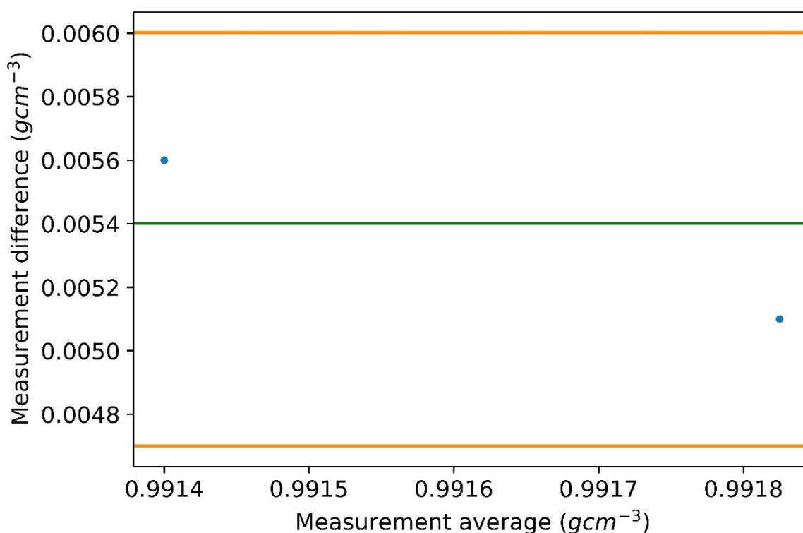
**Figure S14.** The means of the literature value and measured value are plotted against the difference between the two values (blue points). The orange lines denote the upper and lower bounds of two
