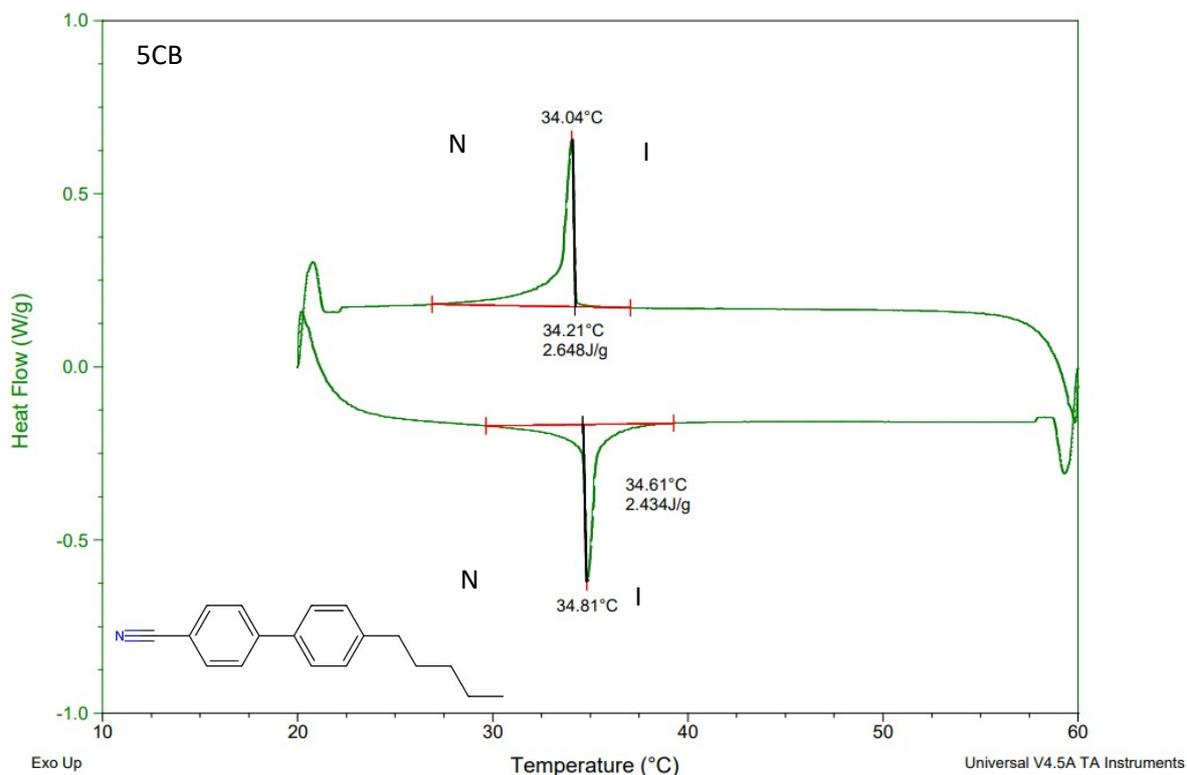
**Figure S1:** DSC Thermogram (endo up, exo down) for 5CB recorded at (10 dC min<sup>-1</sup>). The phase state of liquid crystal through the measurement run is labelled.
