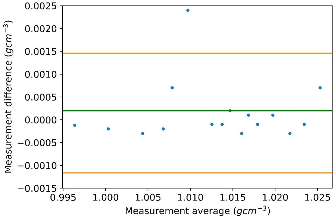
**Figure S10.** The means of the literature value and measured value are plotted against the difference between the two values (blue points). The orange lines denote the upper and lower bounds of two standard deviations. The green line gives the mean difference between literature and measured values.
