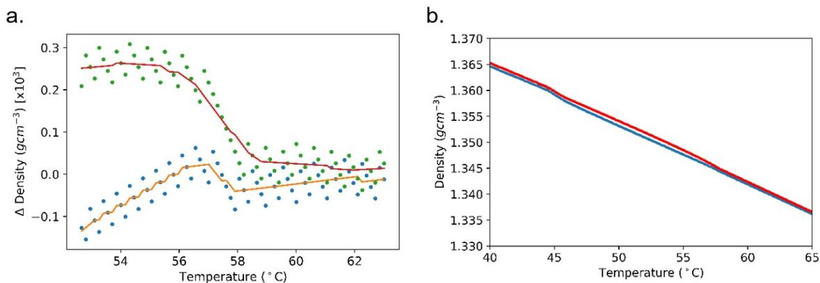
**Figure S8.** These figures show discounting viscosity corrections for M5 can affect the density values over the (a) N-N<sub>x</sub> transition and (b) a temperature range containing N-N<sub>x</sub>-N<sub>F</sub> phases. In (a) the density data without viscosity corrections are shown as the green dots with the red visual guideline. (b) gives the data without viscosity corrections as the red points.
