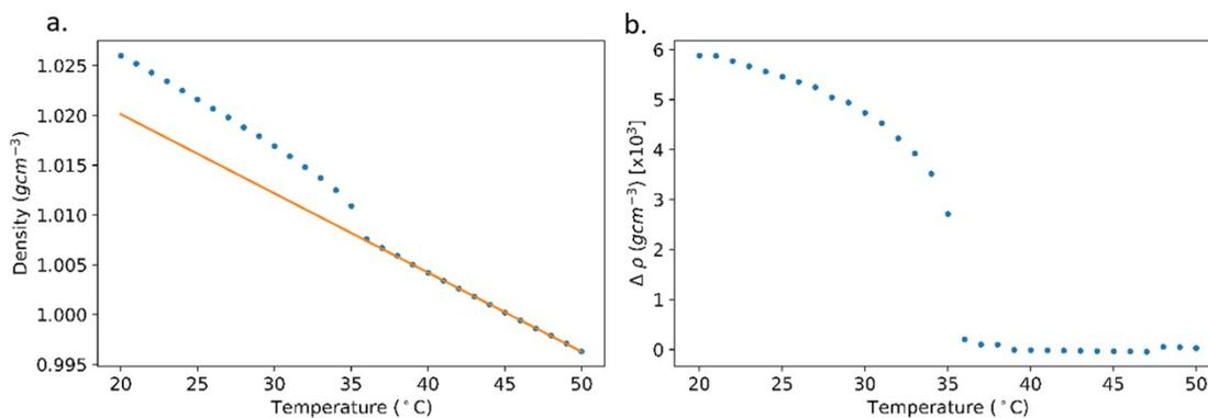
**Figure S6.** An example to illustrate how the deviation of the density at a transition,  $\Delta\rho(T)$  is examined. Densities from a measurement run of 5CB are given in (a) where a linear fit of the density values in the higher temperature phase,  $\rho^{\text{high}T}(T)$  is also shown. The resulting deviation  $\Delta\rho(T) = \rho(T) - \rho^{\text{high}T}$  is then shown in (b).
