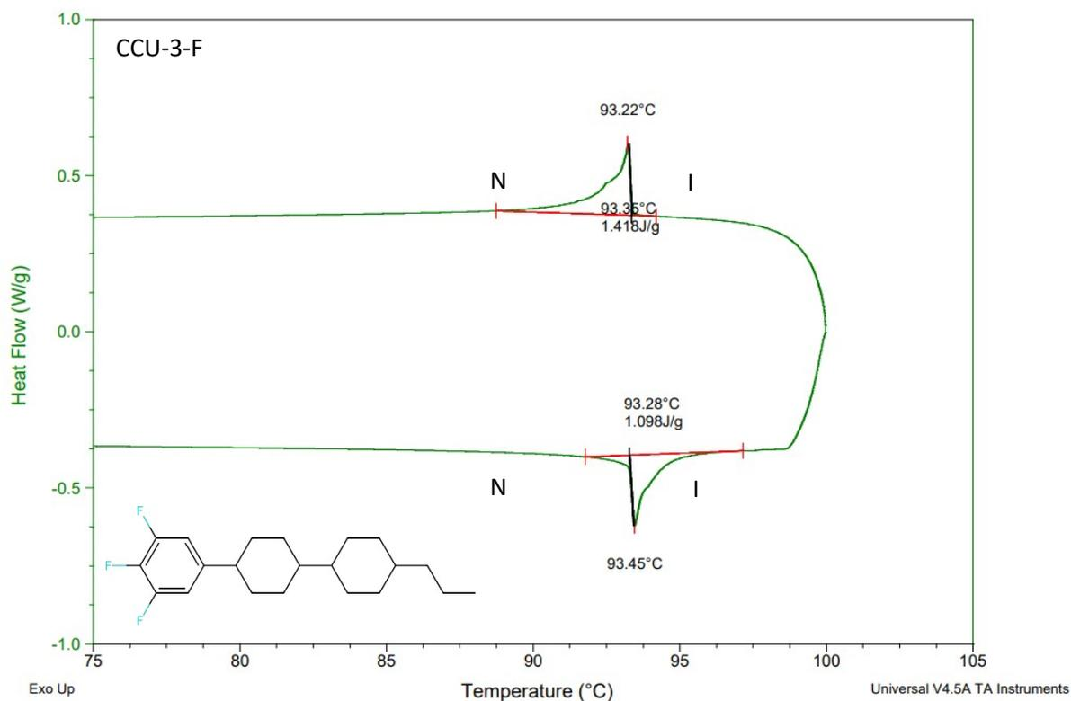
**Figure S4.** DSC Thermogram (endo up, exo down) for CCU-3-F recorded at (10 dC min<sup>-1</sup>). The phase state of liquid crystal through the measurement run is labelled.
