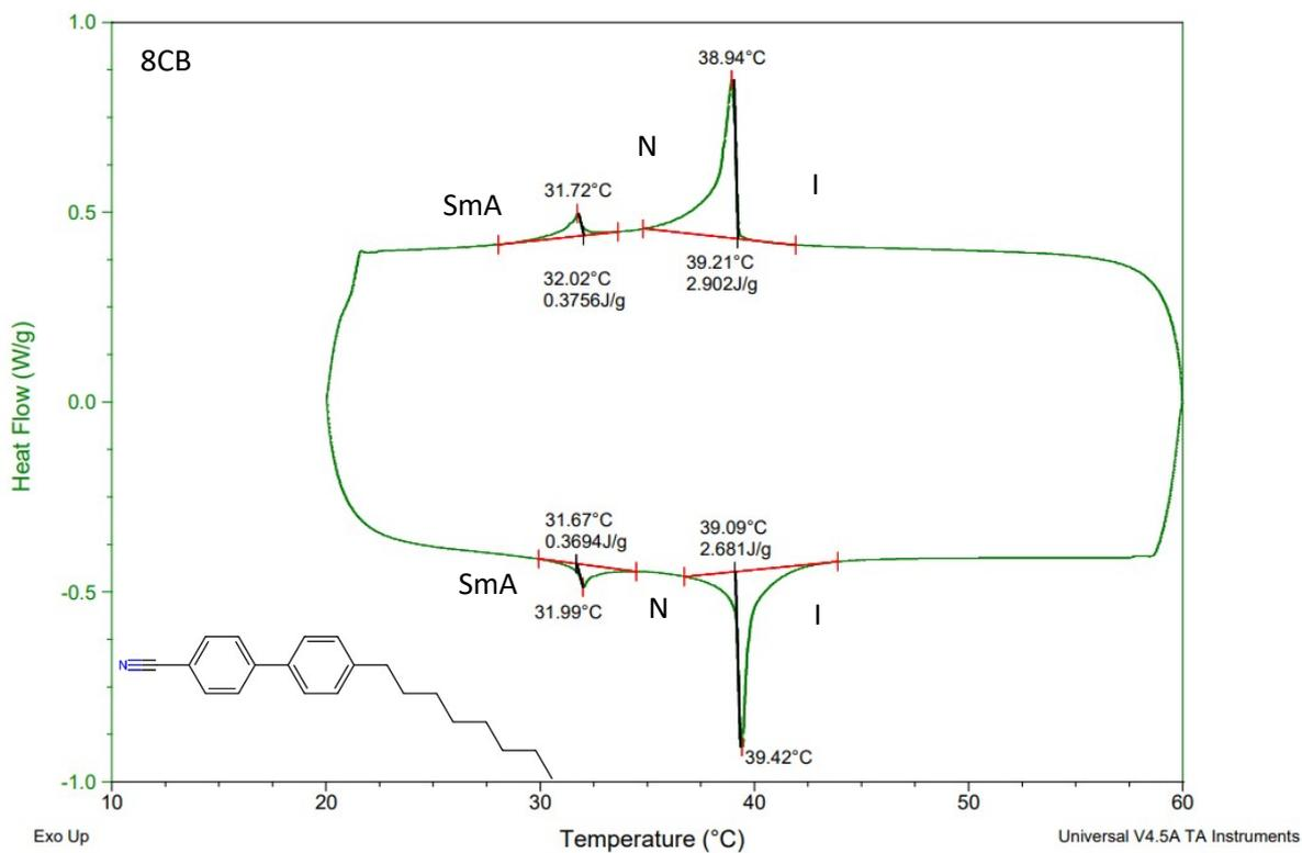
**Figure S2:** DSC Thermogram (endo up, exo down) for 8CB recorded at (10 dC min<sup>-1</sup>). The phase state of liquid crystal through the measurement run is labelled.
