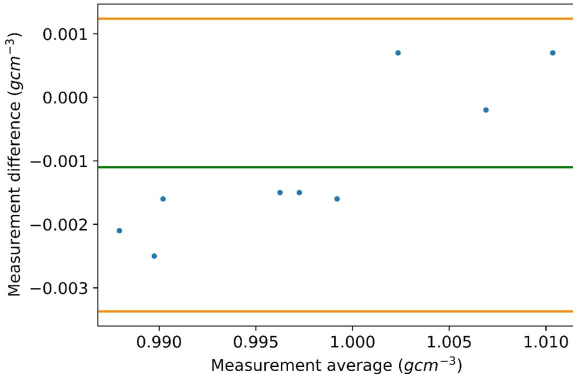
**Figure S17.** The means of the literature value and measured value are plotted against the difference between the two values (blue points). The orange lines denote the upper and lower bounds of two standard deviations. The green line gives the mean difference between literature and measured values.
