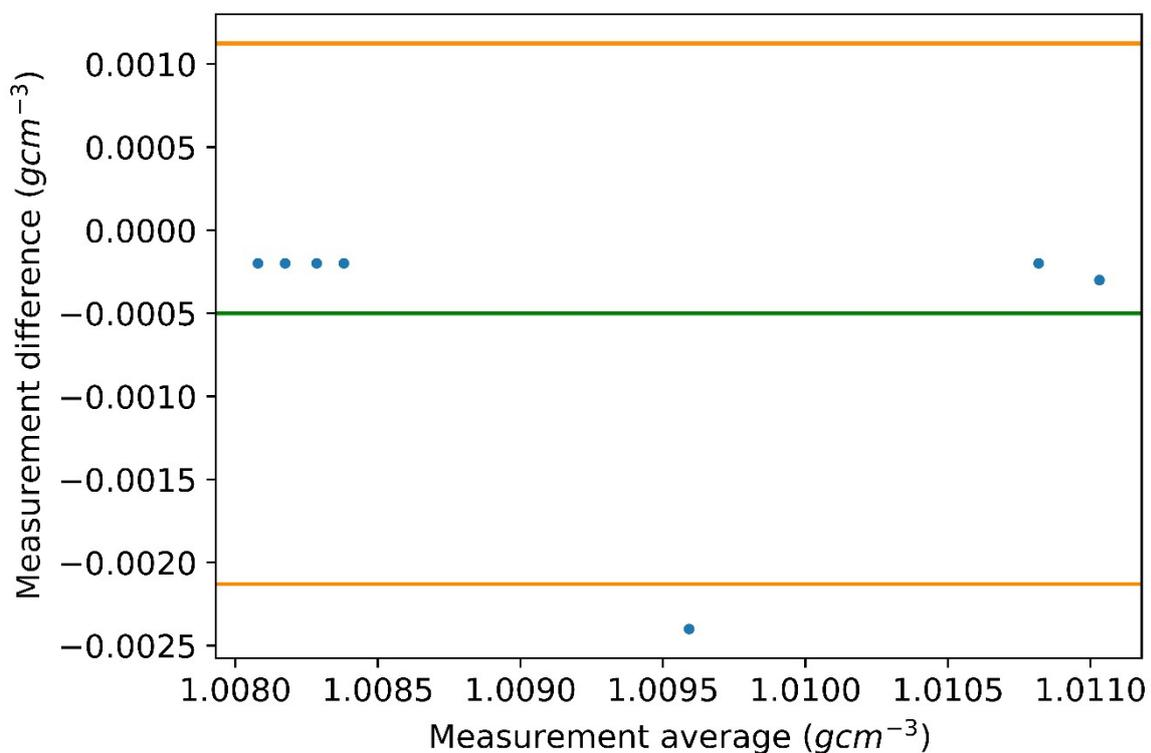
**Figure S9.** The means of the literature value and measured value are plotted against the difference between the two values (blue points). The orange lines denote the upper and lower bounds of two standard deviations. The green line gives the mean difference between literature and measured values.
