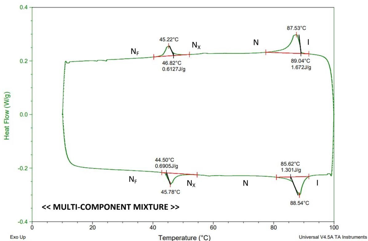
**Figure S5.** DSC Thermogram (endo up, exo down) for M5 recorded at (10 dC min<sup>-1</sup>). The phase state of liquid crystal through the measurement run is labelled.
