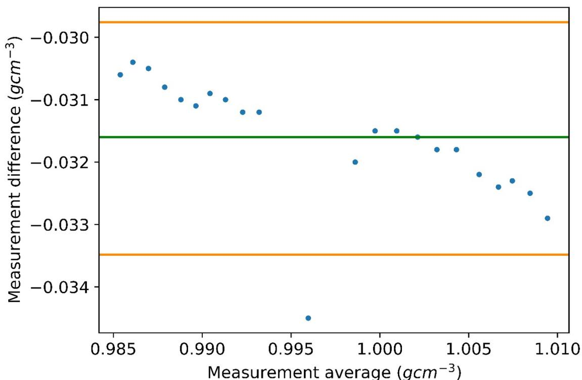
**Figure S16.** The means of the literature value and measured value are plotted against the difference between the two values (blue points). The orange lines denote the upper and lower bounds of two standard deviations. The green line gives the mean difference between literature and measured values.
