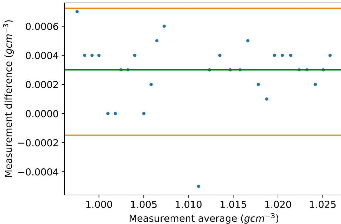
**Figure S11.** The means of the literature value and measured value are plotted against the difference between the two values (blue points). The orange lines denote the upper and lower bounds of two standard deviations. The green line gives the mean difference between literature and measured values.
