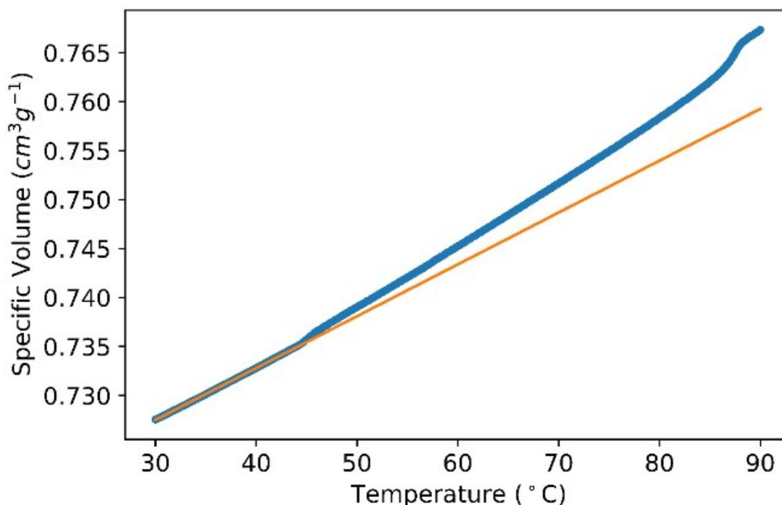
**Figure S18.** The specific volume (1/density) of M5. The orange line represents the linear fit of the density data that is used to calculate a value for the expansion coefficient,  $\alpha$
