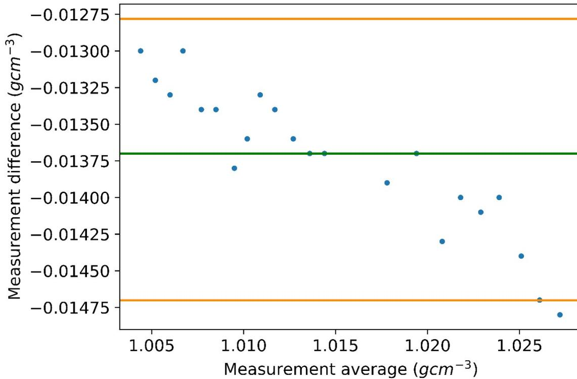
**Figure S12.** The means of the literature value and measured value are plotted against the difference between the two values (blue points). The orange lines denote the upper and lower bounds of two standard deviations. The green line gives the mean difference between literature and measured values.
