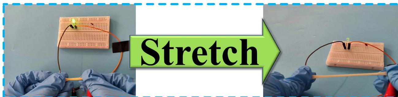
Fig. S1. The brightness change of LED lights follows the stretching
