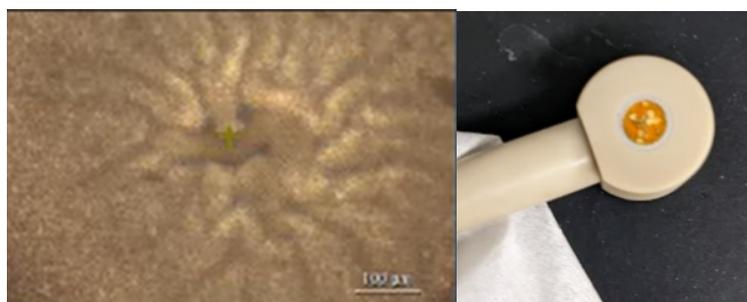
Figure S16. Picture of the electrode surface when a potential is stepped to -2.7 V vs. Ag/Ag<sup>+</sup> (left) showing the formation of solid precipitate that, when exposed to ambient humidity, forms an orange film (right).
