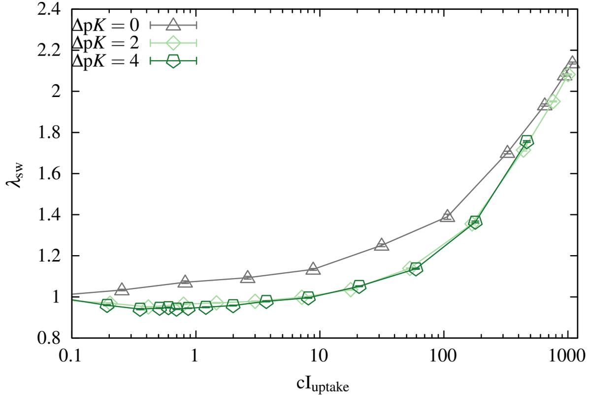
FIG. 3. Degree of swelling as a function of counterions uptake for different  $\Delta pK$ .
