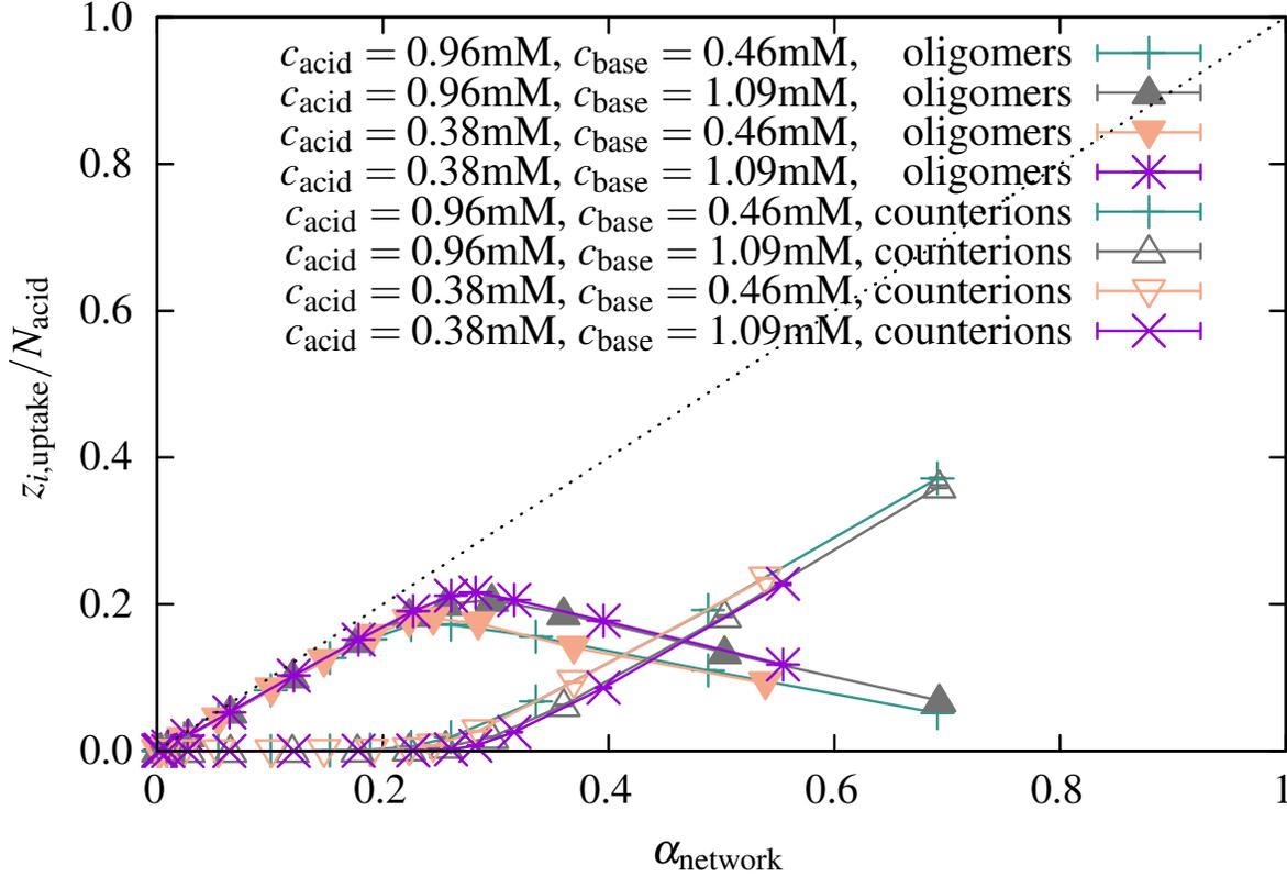
FIG. 9. Number of charges taken up normalized by the total number of acidic beads in the network as the function of the degree of ionization of the network. Oligomers (filled symbols) and counterions of the network (hollow symbols) were investigated separately. The dashed line represents the number of charges taken up equal to the degree of ionization.
