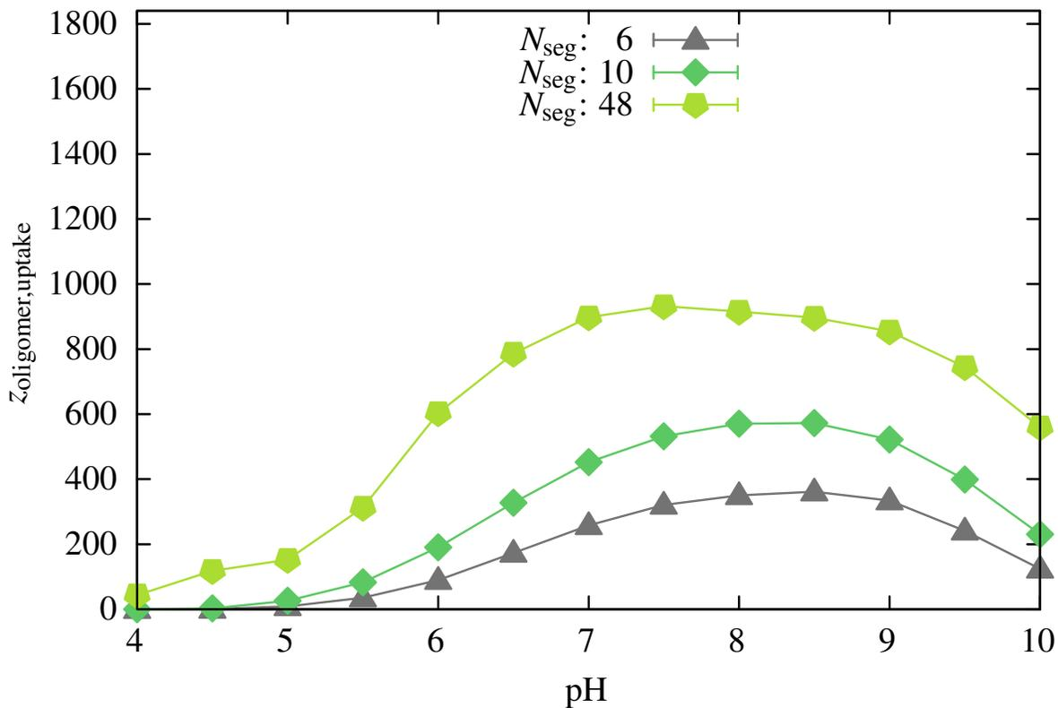
FIG. 6. Number of charges in the oligomers taken up as a function of pH for systems with different oligomer lengths.
