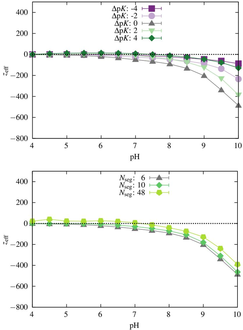
FIG. 2. Effective charge as a function of pH for systems with different oligomer lengths.
