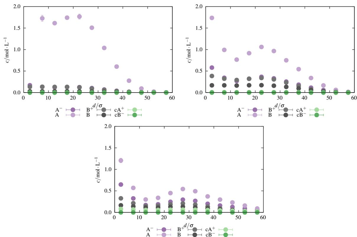
FIG. 8. Concentrations of network monomers, oligomer beads (charged and uncharged), and counterions in the reference system as a function of the distance to the center of mass at a) pH 6, b) pH 8, and c) pH 9
