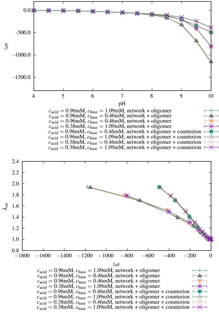
FIG. 10. Effective charge defined as the sum of network charges and oligomer charges taken up (hollow symbols) and counterion included (filled symbols) as a function of pH (top). Degree of swelling as a function of effective charge (down).
