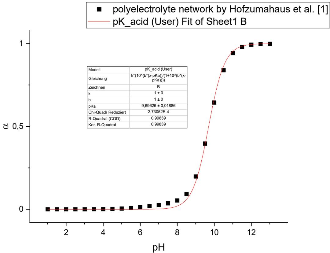
FIG. 1. Degree of ionization of a pure polyelectrolyte network by Hofzumahaus et al.[1] with a fit based on Henderson-Hasselbalch equation.
