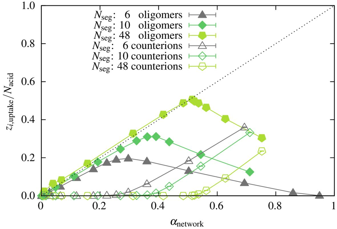
FIG. 7. Number of charges taken up normalized by the total number of acidic beads in the network as the function of the degree of ionization of the network. Oligomers (filled symbols) and counterions of the network (hollow symbols) were investigated separately. The dashed line represents the number of charges taken up equal to the degree of ionization.
