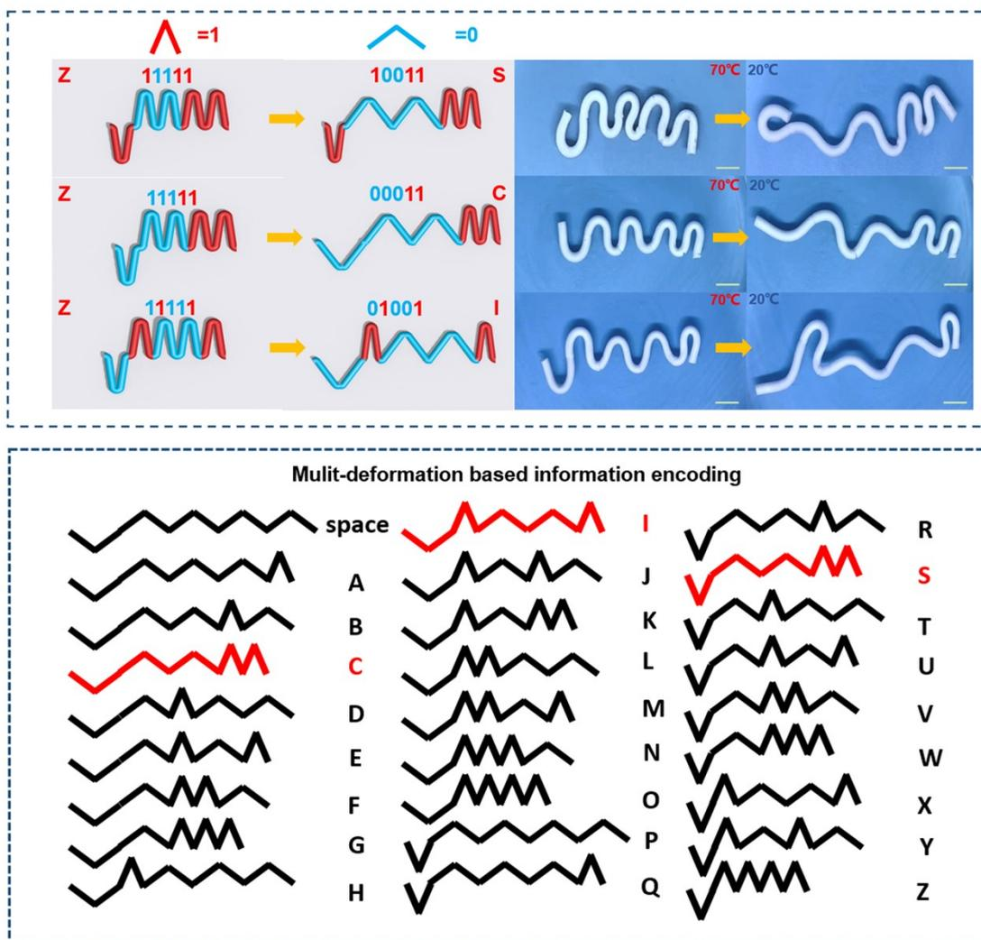
**Fig. S18.** Schematic illustration and photos showing the information encryption and decryption of 2CH-gel based on the editable shape memory function.  $X_{0.42}\text{-Ca}_{0.50}$  and  $X_{0.42}\text{-Ca}_{0.75}$  hydrogel strips were put together in different sequences, then the hydrogel strip was fixed into specific shapes at 70°C, and the hydrogel could display different messages due to the different softening times of each hydrogel pieces. Scale bars = 1.0 cm.
