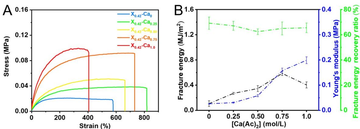
**Fig. S21.** (A) Tensile curves of 2CH-gel after remodeling. (B) The Young's modulus, fracture energy, and fracture energy recovery rate of 2CH-gel after remodeling.
