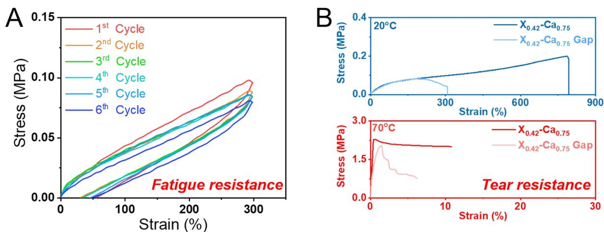
**Fig. S12.** (A) Fatigue resistance of  $X_{0.42}\text{-Ca}_{0.75}$ . (B) Tear resistance of  $X_{0.42}\text{-Ca}_{0.75}$ .
