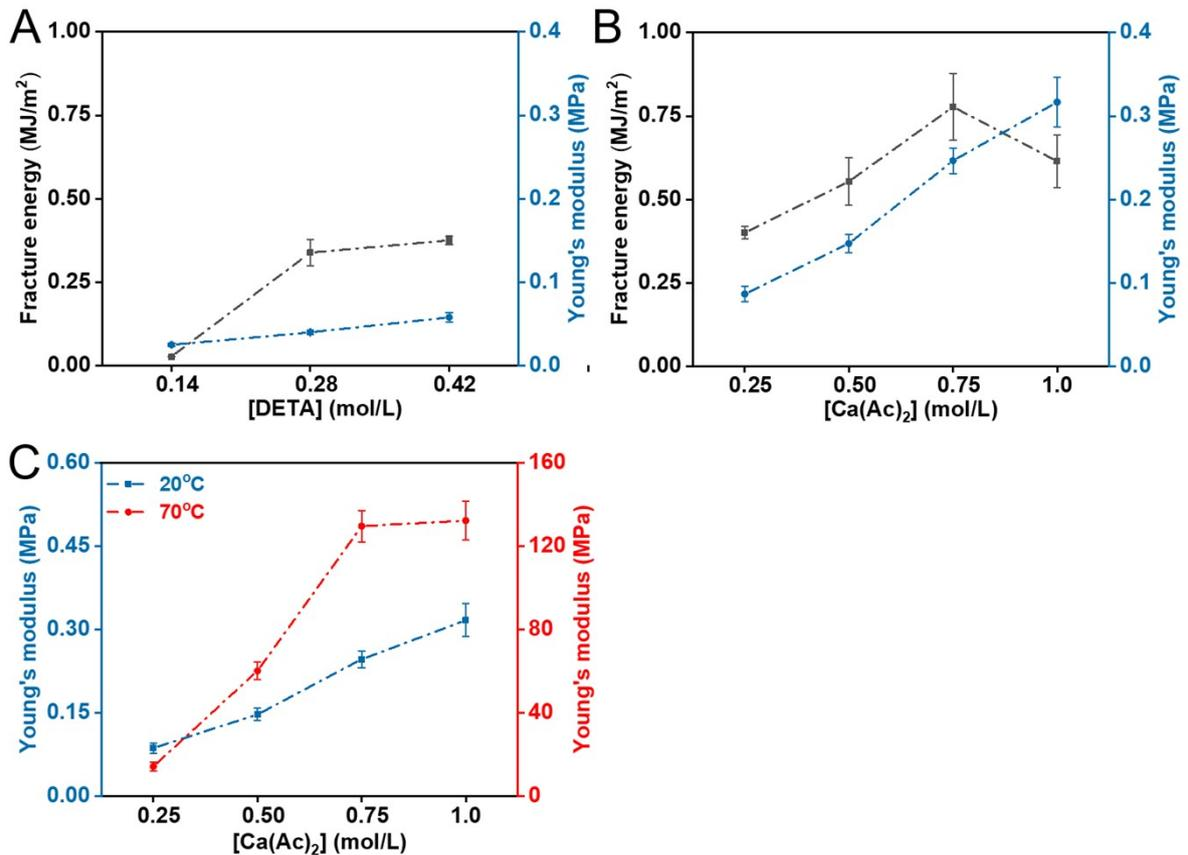
**Fig. S4.** Comparison of mechanical properties of 2CH-gel. (A) Comparison of fracture energy and modulus of PAA/DETA at different DETA concentrations at 20°C. (B) Comparison of fracture energy and modulus of PAA/DETA at different calcium acetate concentrations at 20°C. The concentration of DETA concentration is 0.42 M. (C) Comparison of the modulus of PAA/DETA at 20°C and 70°C with different calcium acetate concentrations. The concentration of DETA is 0.42 M.
