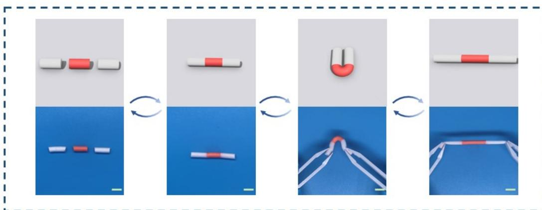
**Fig. S7.** Photos showing the self-healing performance of 2CH-gel. The 2CH-gel is broken into 3 sections by external force, and the 3 sections are placed together in a humid environment and can repair themselves with only 10 seconds of gentle pressure, the middle hydrogel is stained with eosin to make the display effect more obvious. Scale bars = 1.0 cm.
