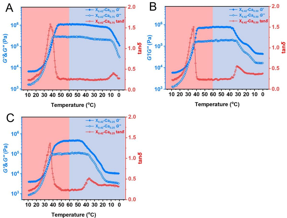
**Fig. S14.** Storage modulus ( $G'$ ) and loss modulus ( $G''$ ) of 2CH-gel as a function of temperature. (A) Storage modulus ( $G'$ ) and loss modulus ( $G''$ ) of  $X_{0.42}\text{-Ca}_{0.75}$  as a function of temperature. (B) Storage modulus ( $G'$ ) and loss modulus ( $G''$ ) of  $X_{0.42}\text{-Ca}_{0.50}$  as a function of temperature. (C) Storage modulus ( $G'$ ) and loss modulus ( $G''$ ) of  $X_{0.42}\text{-Ca}_{0.25}$  as a function of temperature.
