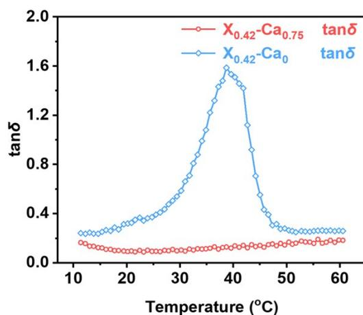
**Fig. S8.** Loss tangent as function of temperature of 2CH-gel with and without  $\text{Ca}(\text{Ac})_2$ .
