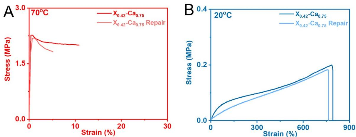
**Fig. S11.** Stress-strain curves of  $X_{0.42}\text{-Ca}_0$  and  $X_{0.42}\text{-Ca}_{0.75}$  before and after self-healing at 20 °C and 70 °C.
