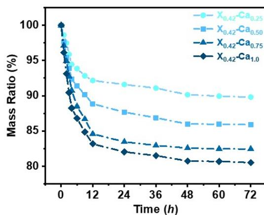
**Fig. S2.** Mass change curve of PAA/DETA hydrogels during immersing in calcium acetate solution over 72 h. Calcium acetate solutions (0.25 M, 0.5 M, 0.75 M, 1 M) were used.
