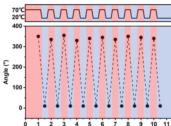
**Fig. S22.** Cyclic testing indicates the reversible phase separation behavior exhibited by 2CH-gel after remodeling.
