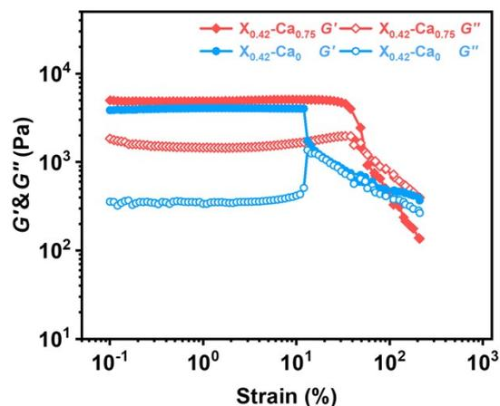
**Fig. S6.** Oscillatory amplitude sweep of 2CH-gel with and without  $\text{Ca}(\text{Ac})_2$ .
