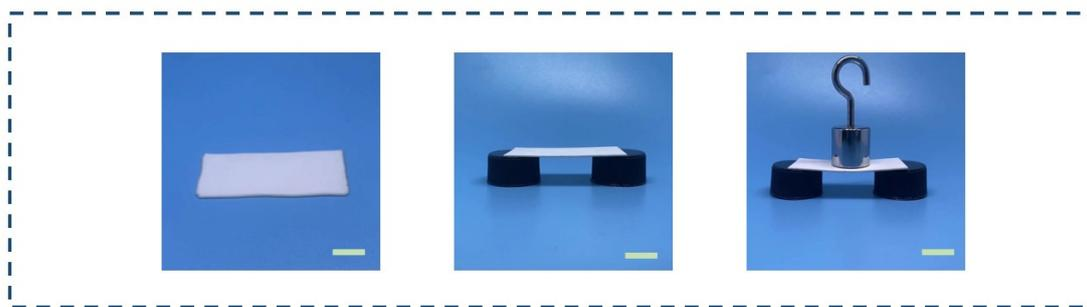
**Fig. S10.** Photos showing the thermal stiffening effect of 2CH-gel. A piece of 2CH-gel was heated in hot water at 70°C for 10 s, and then it could support a 100 g weight without deformation. (Sample size: ~20 mm × 60 mm × 1 mm). Scale bars = 1.0 cm.
