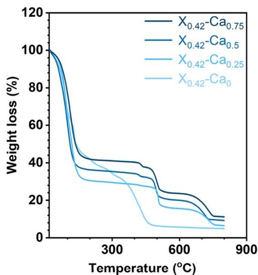
**Fig. S3.** TGA thermograms of 2CH-gel with 0.42 M of DETA and with different  $\text{Ca}(\text{Ac})_2$  concentration.
