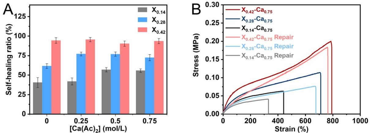
**Fig. S5.** Self-healing properties of 2CH-gel. (A) The self-healing efficiency of 2CH-gel with different concentration of DETA and Ca(Ac)<sub>2</sub>. (B) tensile curves of 2CH-gel before and after self-healing.
