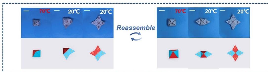
**Fig. S17.** 3D message encryption display of 2CH-gel.  $X_{0.42}\text{-Ca}_{0.50}$  and  $X_{0.42}\text{-Ca}_{0.75}$  hydrogels are assembled into a star-shape, letters are printed on each corner and the star-shaped hydrogel are fixed into a tetrahedron by heating at  $70^\circ\text{C}$ . Each corner has a different opening speed to display information (left), while the star-shaped hydrogel can be re-assembled to display different information (right). Scale bars = 1.0 cm.
