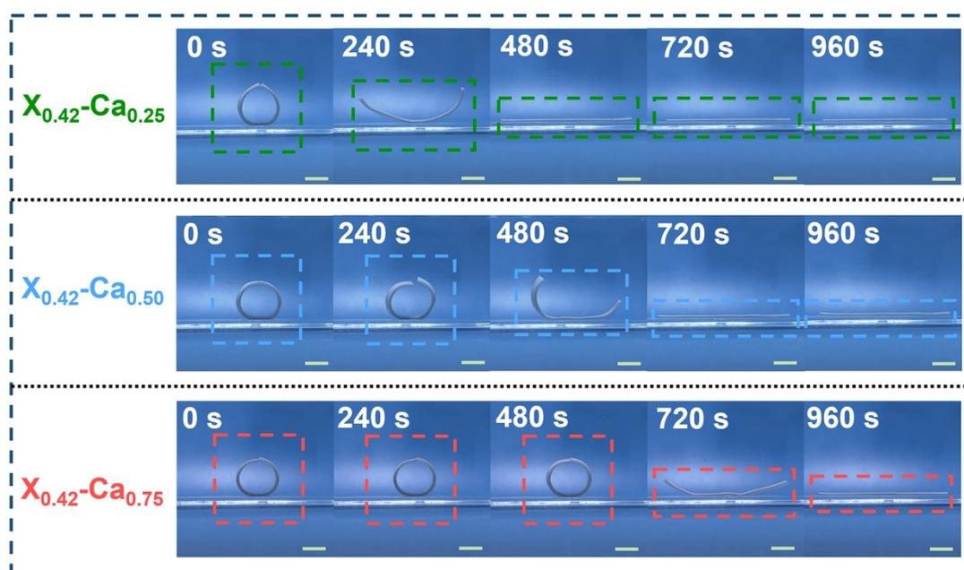
**Fig. S16.** Photos showing the shape recovery of  $X_{0.42}\text{-Ca}_{0.25}$ ,  $X_{0.42}\text{-Ca}_{0.50}$ , and  $X_{0.42}\text{-Ca}_{0.75}$  after shape fixation in  $70^\circ\text{C}$  water for 10 s.
