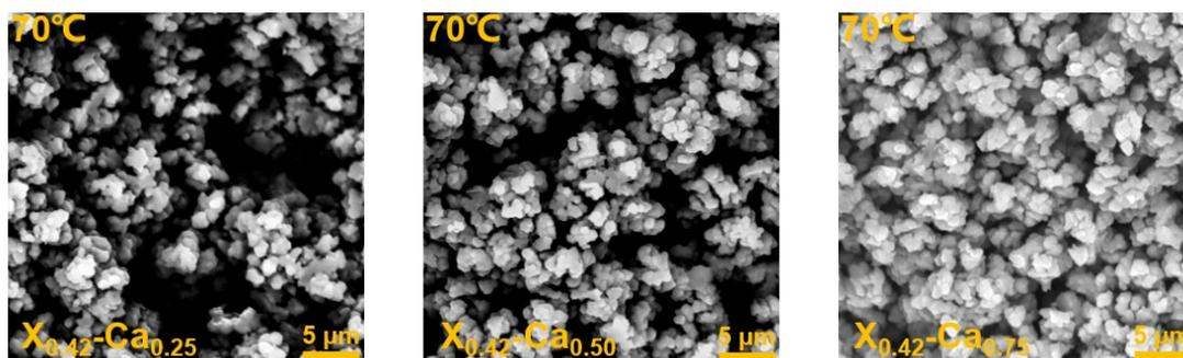
**Fig. S15.** Scanning electron micrographs of  $X_{0.42}\text{-Ca}_{0.25}$ ,  $X_{0.42}\text{-Ca}_{0.50}$  and  $X_{0.42}\text{-Ca}_{0.75}$  at  $70^\circ\text{C}$ .
