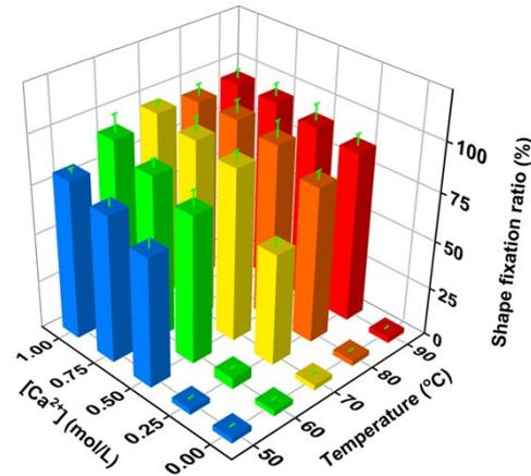
**Fig. S13.** The influences of the temperature and concentration of  $\text{Ca}(\text{Ac})_2$  aqueous solution on the shape fixity ratio of 2CH-gel.
