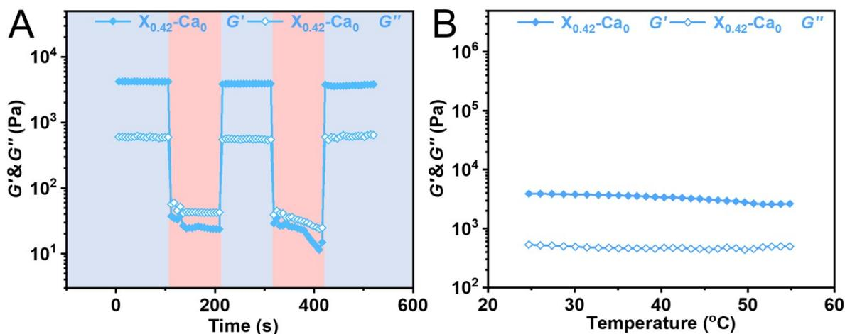
**Fig. S20.** (A) Alternating strain rheology curves (high strain (250%) and low strain (1.0%)) of 2CH-gel without  $Ca(Ac)_2$  after being remodeled. (B) Temperature scanning rheology curves of 2CH-gel without  $Ca(Ac)_2$  after being remodeled.
