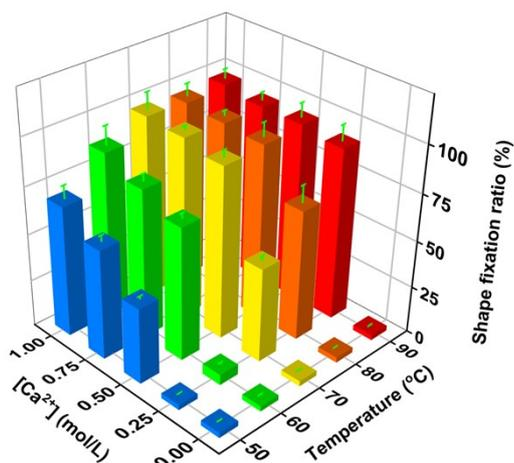
**Fig. S23.** The influences of the temperature and concentration of  $\text{Ca}(\text{Ac})_2$  aqueous solution on the shape fixity ratio of 2CH-gel after remodeling.
