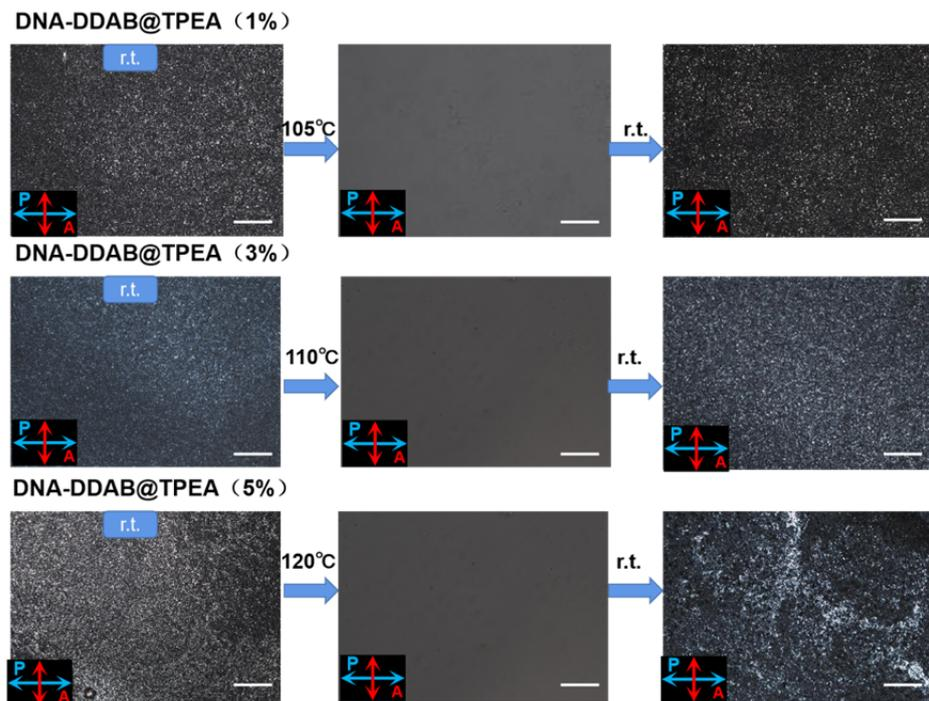
**Figure S8.** Temperature-dependent POM analyses on the phase changes of DNA-DDAB@TPEA LCs. Scale bar: 20  $\mu\text{m}$ .
