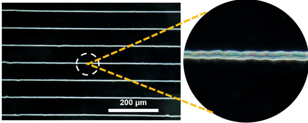
**Fig. S6** The dark field image of bending PEDOT:PSS arrays with small angle indicated the freezing assembly strategy can achieve fine control on the micro-morphology of PEDOT:PSS fibers.
