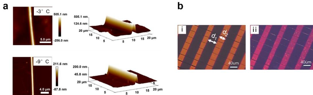
**Fig. S9** Morphological characterization of PEDOT:PSS nanowires. **(a)** AFM image of PEDOT:PSS nanowires assembled at  $-3^{\circ}\text{C}$  and  $-9^{\circ}\text{C}$ , respectively. **(b)** Optical microscopy image of PEDOT:PSS pattern arrays coated with Au electrode (i) ( $d_1$  was the distance between two adjacent Au electrodes;  $d_2$  was width of Au electrode) and in situ polarized optical microscopy image of PEDOT:PSS pattern arrays (ii).
