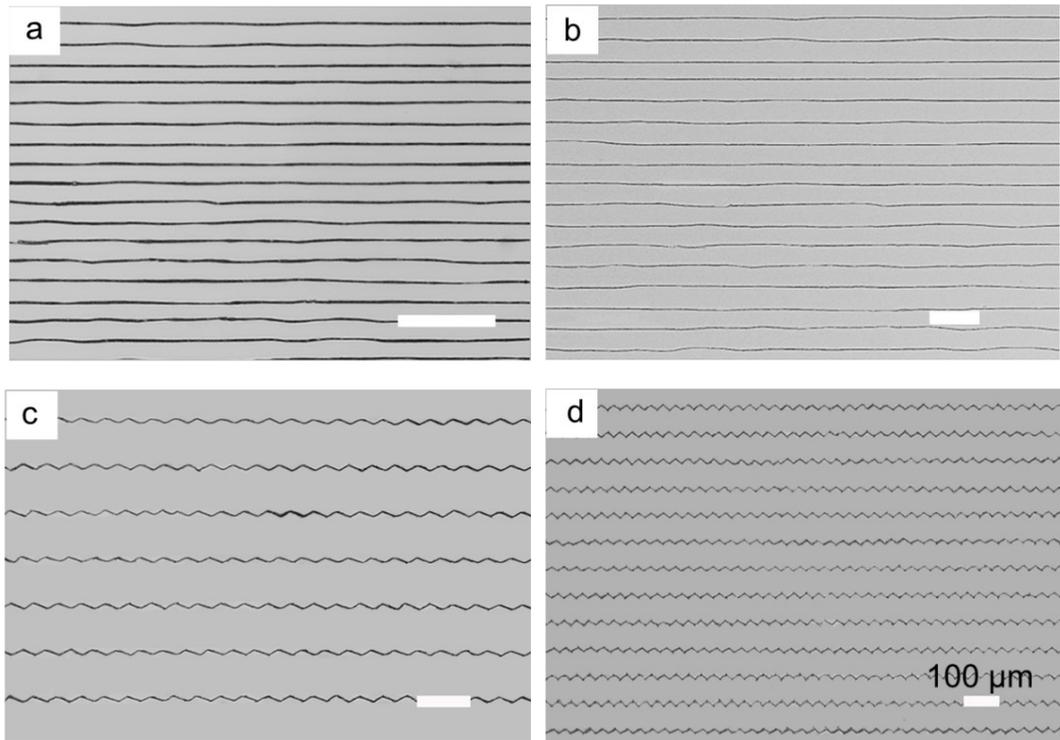
**Fig. S2** Large-area PEDOT:PSS fibers array. **(a-b)** Linear nanofibers array ( $L = 20 \mu\text{m}$  and  $50 \mu\text{m}$ ). **(c-d)** Bending arrays ( $\theta = 120^\circ$ ,  $L = 90 \mu\text{m}$ ,  $120 \mu\text{m}$ ); ( $\theta = 90^\circ$ ,  $L = 80 \mu\text{m}$ ,  $110 \mu\text{m}$ ). All scale bars were  $100 \mu\text{m}$ .
