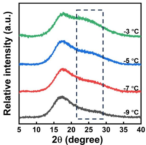
**Fig. S7** XRD diffraction pattern of PEDOT:PSS assembled at different temperature (-3 °C, -5 °C, -7 °C, -9 °C) annealing for 48h. The higher assembly temperature results in stronger intensity at  $2\theta = 25.6^\circ$ .
