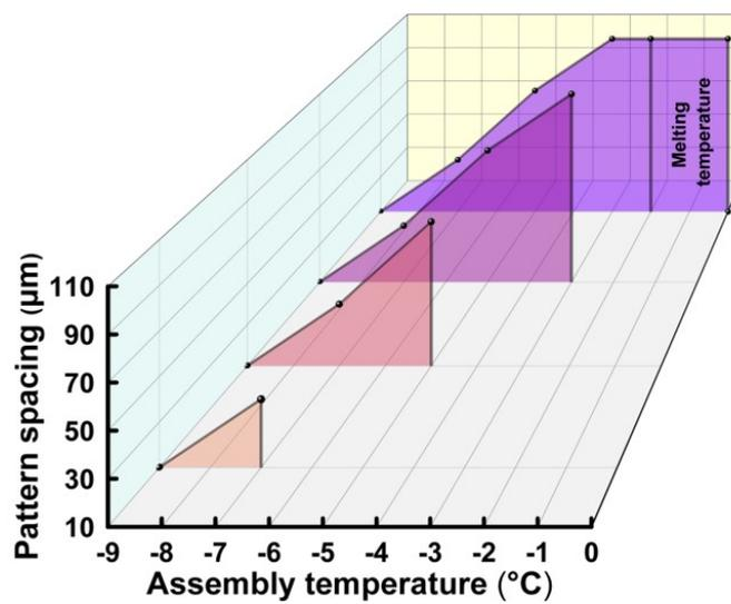
**Fig. S4** The phase diagram shows the correlation of assembly temperature with pattern spacing.
