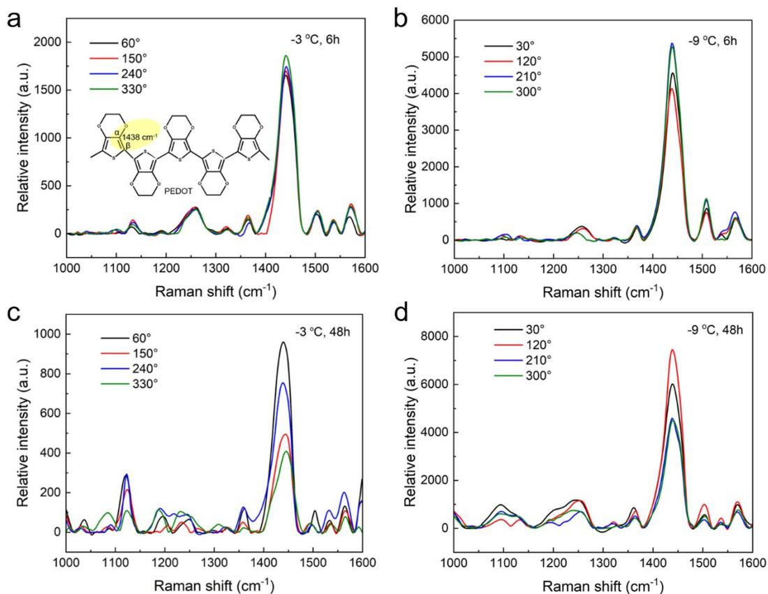
**Fig. S8** (a-b) Raman spectra of PEDOT:PSS nanofibers assembled at -3 °C and -9 °C for 6 h in different polarized degrees. The peak of 1438 cm<sup>-1</sup> was attributed to double-bond stretching vibration of C<sub>α</sub>=C<sub>β</sub>(-O). (c-d) Raman spectra of PEDOT:PSS annealed at -3 °C and -9 °C for 48 h at diverse polarized degrees.
