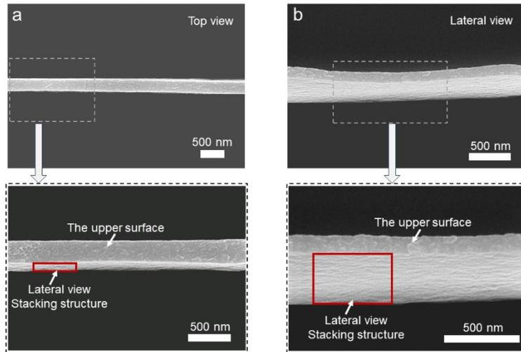
**Fig. S3** SEM image of PEDOT:PSS nanowire microstructure. **(a)** The PEDOT:PSS nanowire was rotated 30° clockwise. **(b)** The PEDOT:PSS nanowire was rotated 60° clockwise. The lateral view indicate that the interior of the nanowire was layer-by-layer stacked structure.
