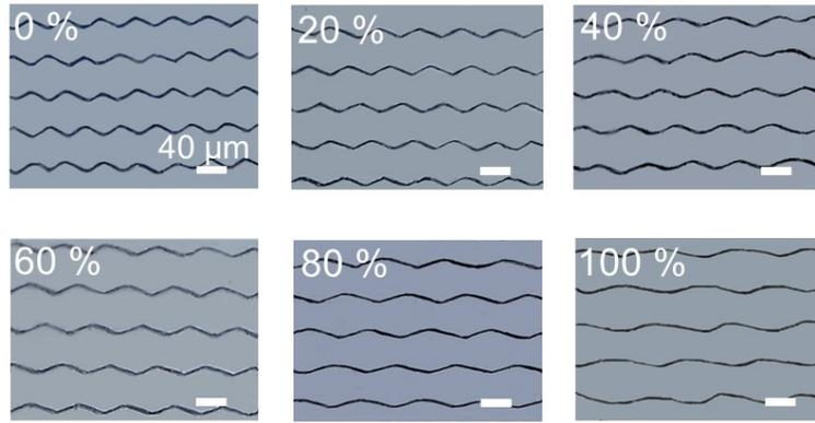
**Fig. S10** PDMS film with PEDOT:PSS bend pattern in different strain (0%, 20%, 40%, 60%, 80%,100%). All scale bars were 40  $\mu\text{m}$ .
