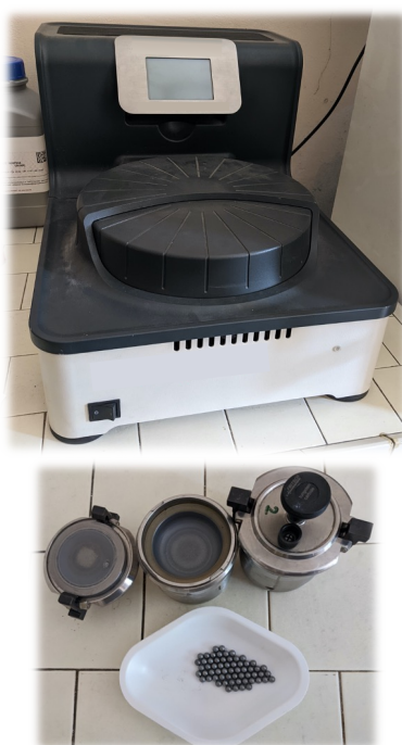
Figure S2. Ball-milling system used.
