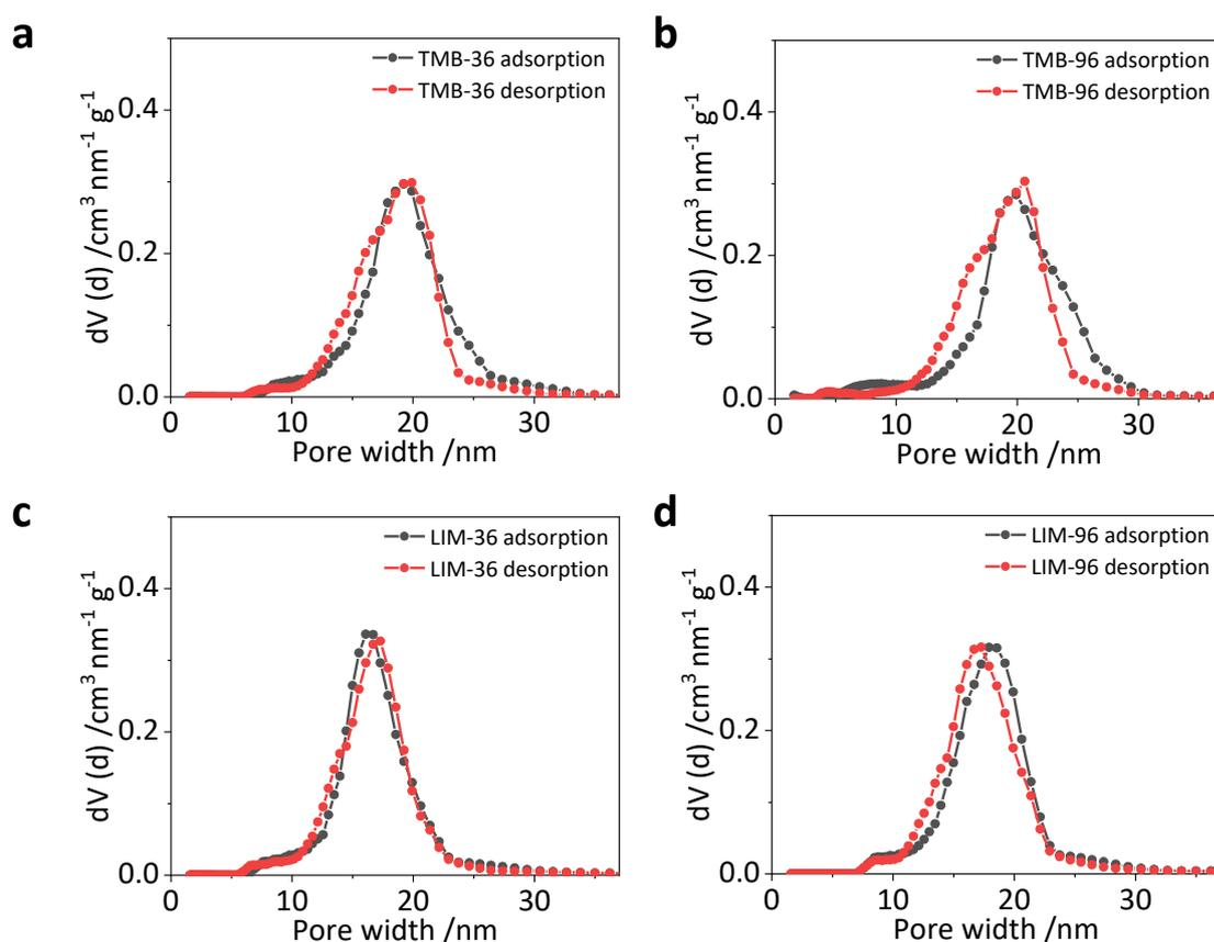
**Figure S2.** Pore size distributions from nitrogen physisorption for samples synthesised with low (36) and high (96) expander/P123 molar ratio using TMB (top row) and limonene (LIM, bottom row). The comparison of pore size distributions calculated from the adsorption and desorption branches of the isotherms shows very similar mode pore diameters. This indicates that the majority of the pores are not restricted by narrower pore openings and are freely accessible.
