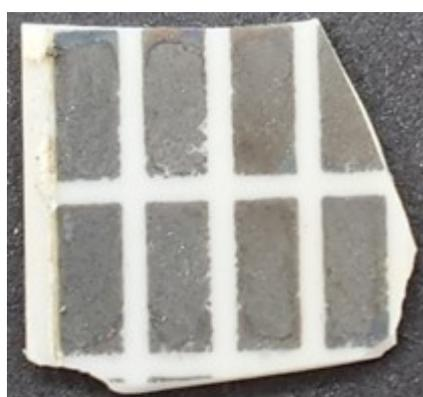
**Figure S7.** Photograph of a ceramic plate after Cu removal (after repeated contacts with  $0.1 \text{ mol}\cdot\text{dm}^{-3}$  Cu(II) chloride in a ChCl brine containing  $1.0 \text{ mol}\cdot\text{kg}^{-1}$  chloride), revealing the grey W layer.
