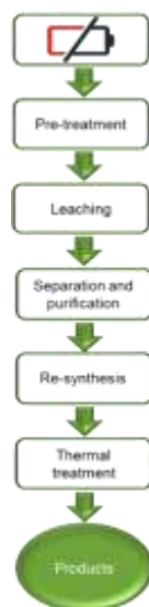
Supplementary Figure S5 GEM Ltd. recycling process [3].
