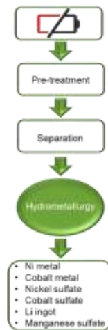
Supplementary Figure S9 SungEel HiTech LIB recycling process [3].
