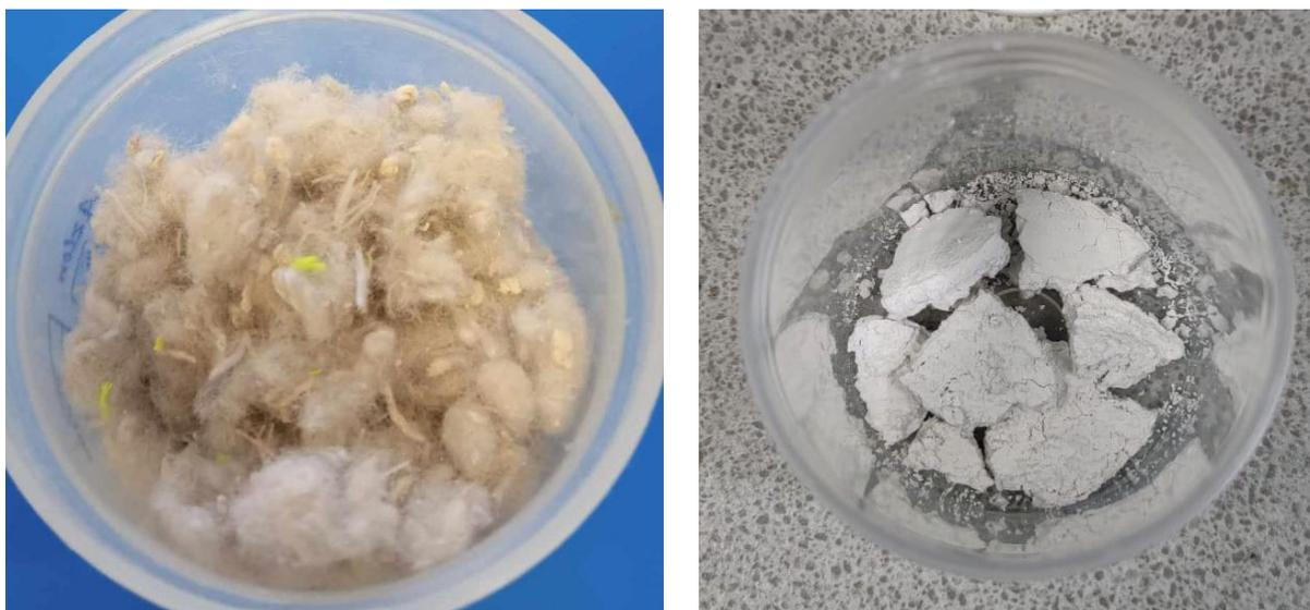
**Figure S3:** Images of (left) nonwoven carpet yarn prior to dissolution and (right) recycled PP.
