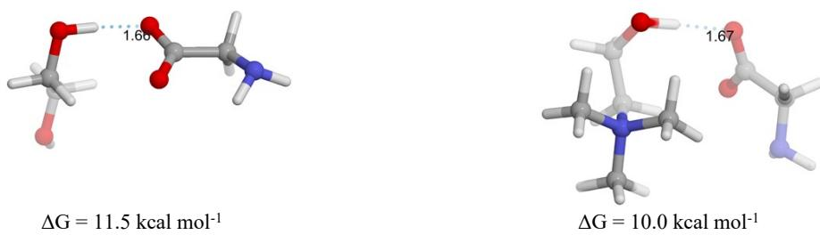
**Fig. S6.** Competition in deprotonation of glycol (left) *versus* choline (right) by glycinate in TS<sub>addition</sub> in isolated calculations.
