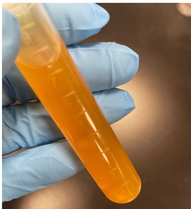
Figure S5. Optical image of Fe 2+ color in aqueous solution.
