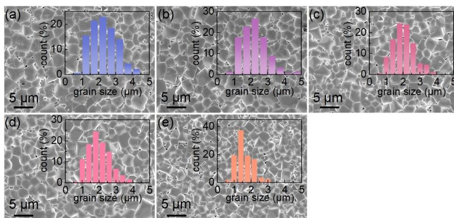
Fig. S3 SEM morphologies of BNT-BSZS ceramics and corresponding grain size distribution: (a)  $x = 0$ , (b)  $x = 0.10$ , (c)  $x = 0.15$ , (d)  $x = 0.20$ , (e)  $x = 0.25$ .
