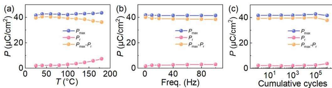
Fig. S6 Evolution of  $P_{\max}$ ,  $P_r$  and  $P_{\max} - P_r$  of  $x = 0.2$  under different temperatures, frequencies and cycling numbers.
