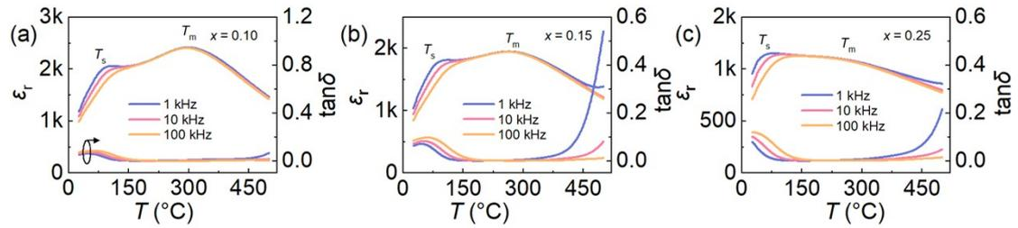
Fig. S2 Temperature-dependent permittivity ( $\epsilon_r$ ) and loss ( $\tan\delta$ ) of (a)  $x = 0.10$ , (b)  $x = 0.15$ , (c)  $x = 0.25$ .
