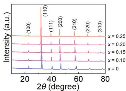
Fig. S1 XRD patterns of  $(1-x)\text{BNT}-x\text{BSZS}$  ceramics.
