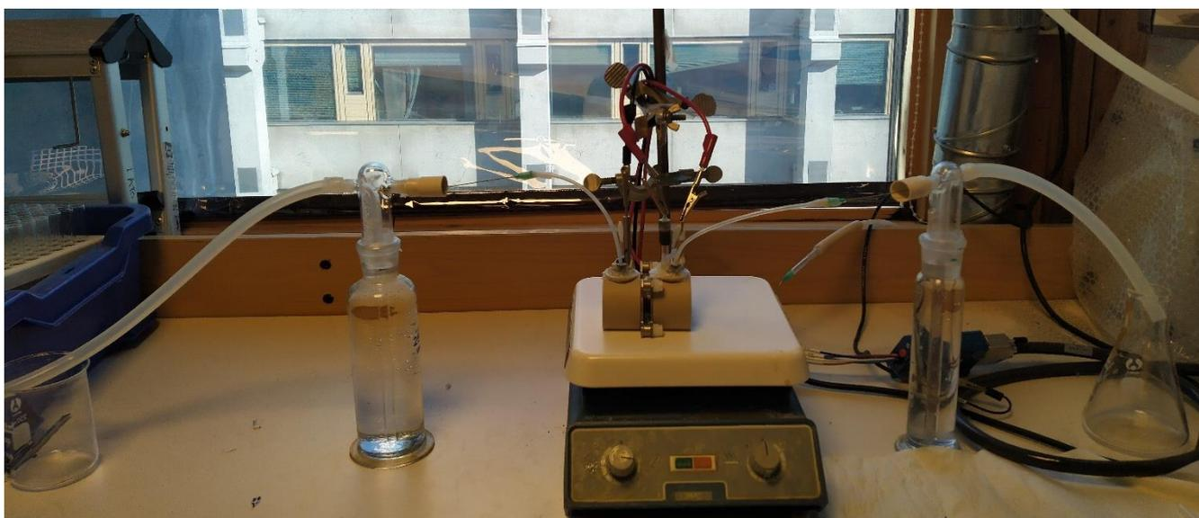
**Figure S15.** A graphic illustration of the home-made electrolysis set-up for the overall water electrolysis at pH 7 and quantitative gas detections from the anode ( $O_2$ ) and cathode ( $H_2$ ) compartments using an H-cell (purchased from redox.me). The anode and cathode compartments were separated by a Nafion-117 membrane.
