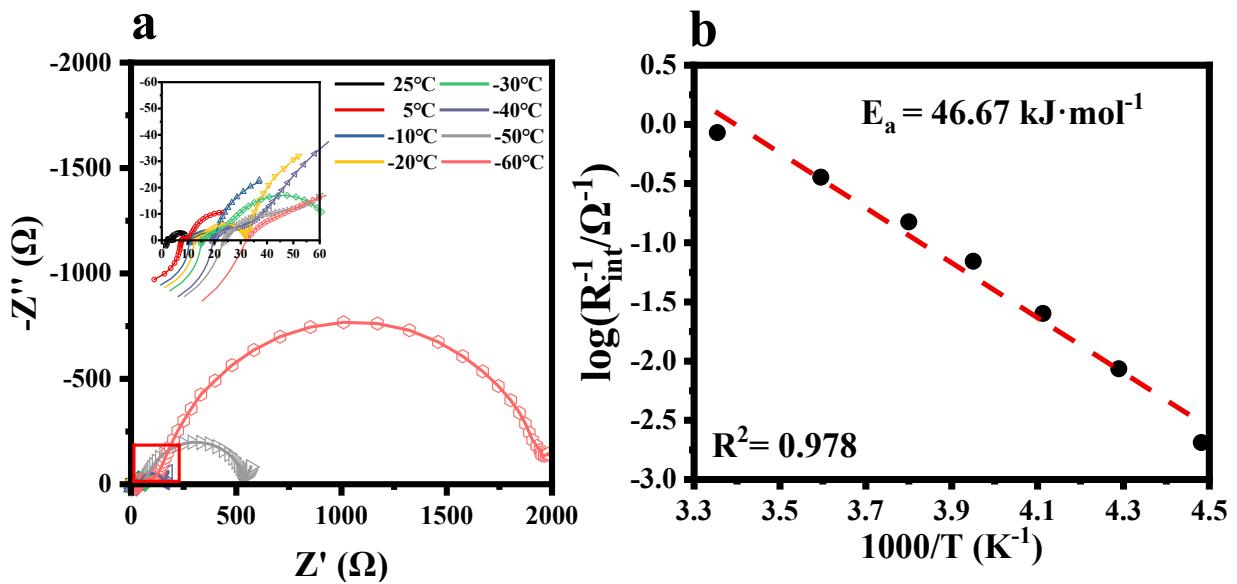
**Fig. S17** (a) The Nyquist plots of the Li-Li symmetric cell at different temperatures. The inset: the enlarged view of the part marked by the red square. (b) The interfacial resistance  $R_{int}$  fitted by the Arrhenius equation to obtain the activation energy  $E_a$ .
