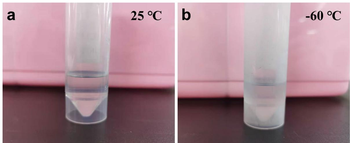
**Fig. S3** Digital photos of the 1 M LiTFSI-DOL/DME electrolyte at (a) 25 °C and (b) -60 °C.
