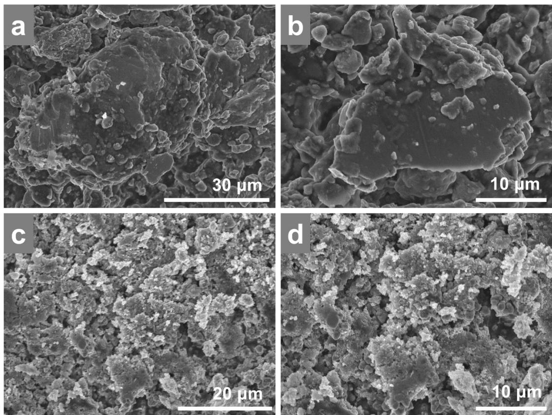
**Fig. S11** SEM images of (a, b) pristine Cu<sub>2</sub>S electrode (with Cu foil as the current collector) and (c, d) the one after the 20<sup>th</sup> delithiation at 0.3 C.
