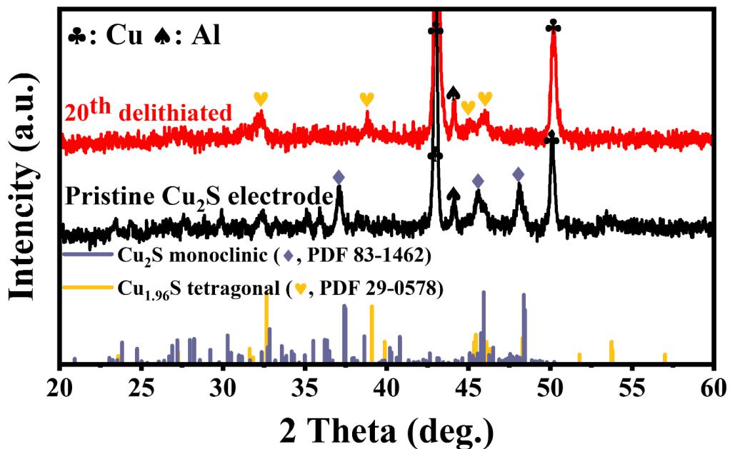
**Fig. S10** XRD patterns of pristine  $\text{Cu}_2\text{S}$  electrode (with Cu foil as the current collector) (black line) and the one after the 20<sup>th</sup> delithiation at 0.3 C (red line) with the standard diffraction patterns of monoclinic  $\text{Cu}_2\text{S}$  (JCPDF No. 83-1462) and tetragonal  $\text{Cu}_{1.96}\text{S}$  (JCPDF No. 29-0578) also presented. Note: the Al signals originate from the aluminium XRD sample holder.
