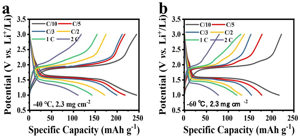
**Fig. S6** The galvanostatic charge-discharge curves from 0.1 C (33 mA g<sup>-1</sup>) to 2 C (674 mA g<sup>-1</sup>) for the Li-Cu<sub>2</sub>S half-cells (with Cu<sub>2</sub>S loading of 2.3 mg cm<sup>-2</sup>) at (a) -40 °C and (b) -60 °C.
