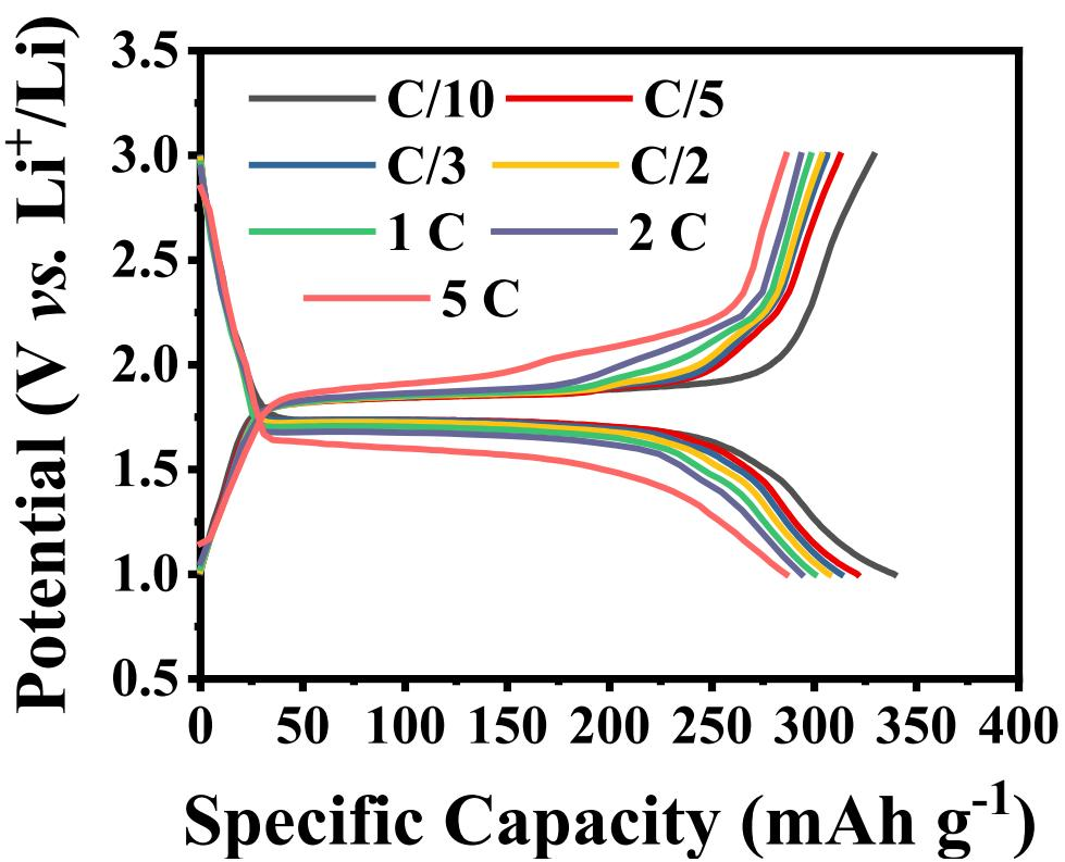
**Fig. S4** The galvanostatic charge-discharge curves from 0.1 C to 5 C for the Li-Cu<sub>2</sub>S half-cell (with Cu<sub>2</sub>S loading of 2.3 mg cm<sup>-2</sup>) under 25 °C.
