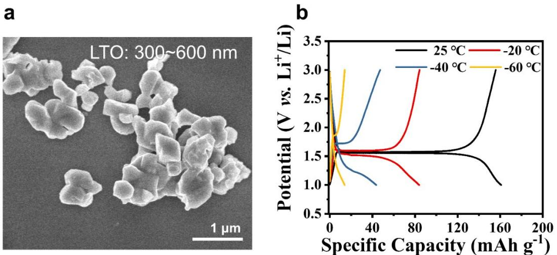
**Fig. S5** (a) The SEM image of commercial LTO powder and (b) the galvanostatic charge-discharge potential profiles of LTO coated on Cu foil current collector at 25 °C, -20 °C, -40 °C, and -60 °C. The charge-discharge current rate and mass loading of LTO in (b) is 0.2 C (32 mA g<sup>-1</sup>) and 2.1 mg cm<sup>-2</sup>.
