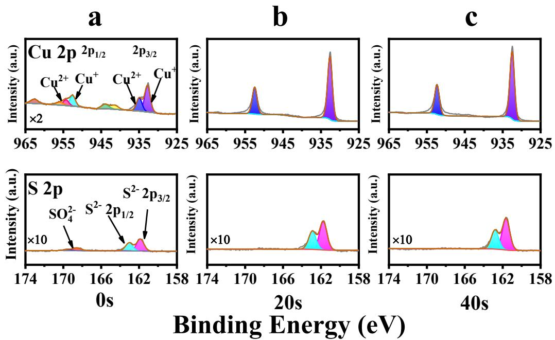
**Fig. S1** X-ray photoelectron spectroscopy (XPS) depth-profiling analysis of pristine Cu<sub>2</sub>S sample. The Cu 2p (top row) and S 2p (bottom row) spectra after argon ion sputtering for (a) 0 s, (b) 20 s, and (c) 40 s, respectively.
