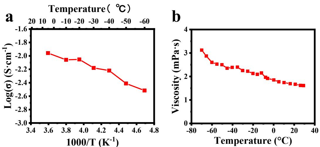
**Fig. S2** Physical properties of the 1 M LiTFSI-DOL/DME electrolyte. Temperature dependence of the (a) ionic conductivity and (b) viscosity of the electrolyte.
