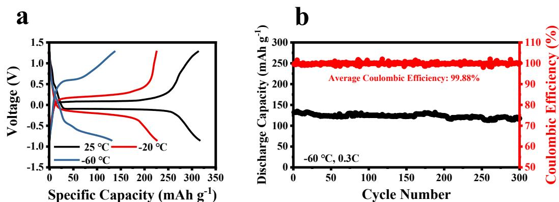
**Fig. S8** (a) The galvanostatic charge-discharge curves of the Cu<sub>2</sub>S-Cu<sub>2</sub>S symmetrical cell tested at 0.3 C (100 mA g<sup>-1</sup>) under 25, -20, and -60 °C. (b) Cycling performance of the Cu<sub>2</sub>S-Cu<sub>2</sub>S symmetrical cell tested at 0.3 C (100 mA g<sup>-1</sup>) under -60 °C.
