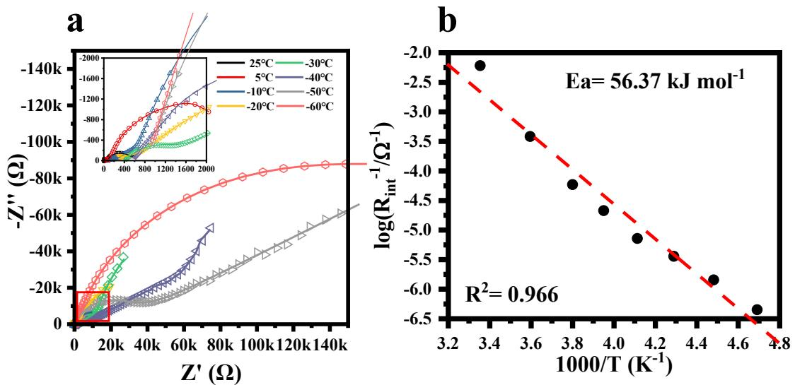
**Fig. S22** (a)The Nyquist plots of the NCM-NCM symmetric cell at different temperatures. The inset: the enlarged view of the part marked by the red square. (b) The interfacial resistance  $R_{int}$  fitted by the Arrhenius equation to obtain the activation energy  $E_a$ .
