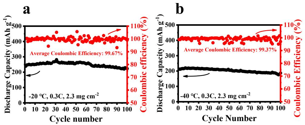
**Fig. S7** Cycling performance of the Li-Cu<sub>2</sub>S half-cells (with Cu<sub>2</sub>S loading of 2.3 mg cm<sup>-2</sup>) at 0.3 C (100 mA g<sup>-1</sup>) under (a) -20 °C and (b) -40 °C.
