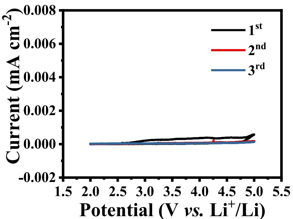
**Fig. S20** Cyclic voltammograms of the 1 M LiTFSI-DOL/DME electrolyte between 2.0 and 5.0 V (vs.  $\text{Li}^+/\text{Li}$ ), which are obtained with Al foil as the working electrode and lithium metal as the counter and reference electrode. The scan rate is  $0.1 \text{ mV s}^{-1}$ .
