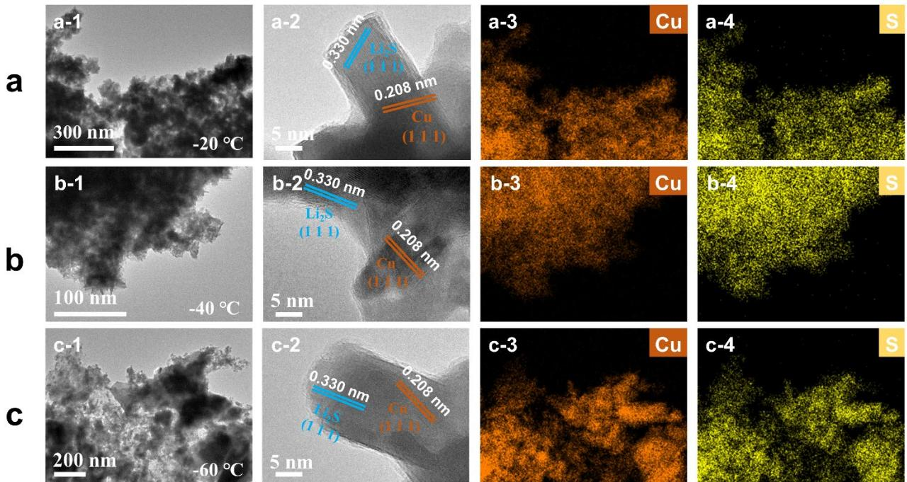
**Fig. S13** (a-1, b-1, c-1) TEM and (a-2, b-2, c-2) HRTEM images (with the *d*-spacings of crystal planes of Li<sub>2</sub>S and Cu marked) of the Cu<sub>2</sub>S electrode after the 10<sup>th</sup> lithiation at 0.3 C under (a) -20, (b) -40, and (c) -60 °C. The corresponding Cu (a-3, b-3, c-3) and S (a-4, b-4, c-4) elemental mapping results of the lithiated samples.
