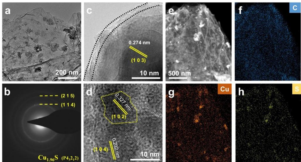
**Fig. S12** Post-mortem TEM characterizations of the  $\text{Cu}_2\text{S}$  after the 20<sup>th</sup> delithiation at 0.3 C. (a) The TEM image, (b) SAED pattern, (c-d) HRTEM images (with the *d*-spacings of crystal planes of  $\text{Cu}_{1.96}\text{S}$  marked), and (e-h) elements mapping results ((f) C, (g) Cu, and (h) S) of the sample.
