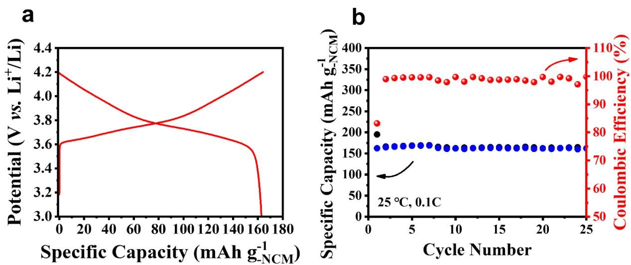
**Fig. S21** (a) The galvanostatic charge-discharge potential profiles and (b) cycling performance of the Li-NCM half-cell under a current rate of 0.1 C ( $1\text{C} = 160 \text{ mA g}^{-1}$ ) and  $25^\circ\text{C}$ .
