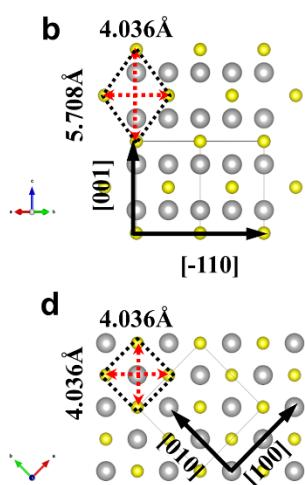
**Fig. S19** Structure of tetragonal Cu<sub>1.96</sub>S along the (a) [100] and (c) [001] directions versus cubic Li<sub>2</sub>S along the (b) [110] and (d) [001] directions. Rhombic and square shapes mark the networks formed by sulfur atoms.
