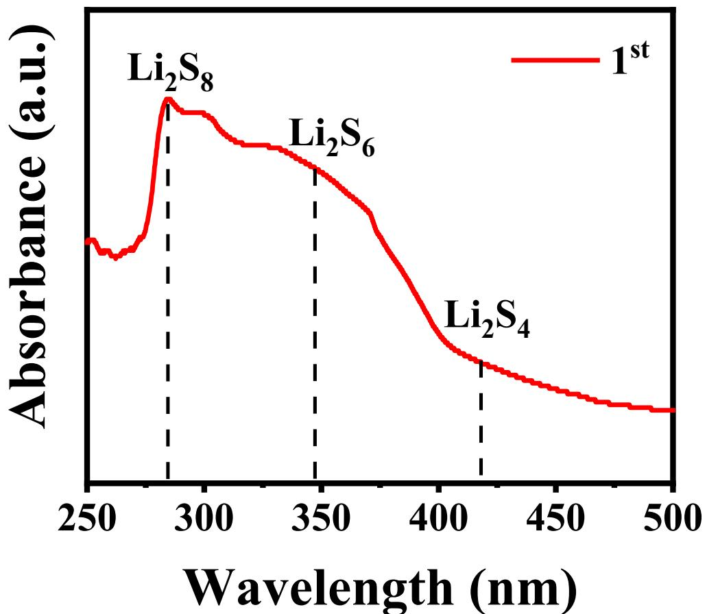
**Fig. S14** UV-vis absorbance spectra (red line) of the electrolyte which was retrieved from the Li-Cu<sub>2</sub>S cells after the first lithiation-delithiation cycle. The characteristic signals (dashed lines) of Li<sub>2</sub>S<sub>8</sub>, Li<sub>2</sub>S<sub>6</sub>, and Li<sub>2</sub>S<sub>4</sub> are also marked.
