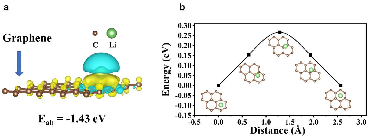
**Fig. S18** (a) The calculated charge density difference and adsorption energy of Li-ion adsorbed on the graphene surface (yellow: charge increase, blue: charge decrease). (b) The calculated energy barrier for the Li-ion diffusion on the surface of graphene (the insets show the configurations of the Li-ion at various states during the diffusion process).
