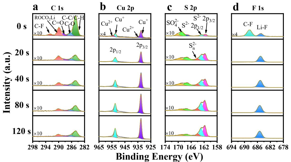
**Fig. S16** XPS depth-profiling analysis of the delithiated Cu<sub>2</sub>S electrode after 50 cycles at 0.3 C. The (a) C 1s, (b) Cu 2p, (c) S 2p, and (d) F 1s spectra after argon ion sputtering for 0 s, 20 s, 40 s, 80 s, and 120 s, respectively.
