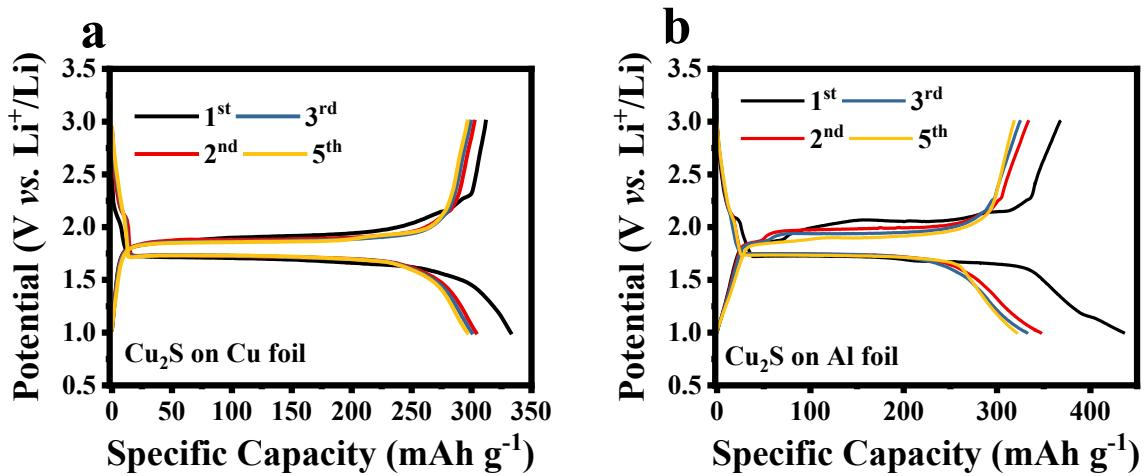
**Fig. S15** The galvanostatic charge-discharge potential profiles of the Li-Cu<sub>2</sub>S half-cells with Cu<sub>2</sub>S coated on the (a) Cu and (b) Al foil, respectively. The results clearly show the absence of the 2.28 V delithiation plateau.
