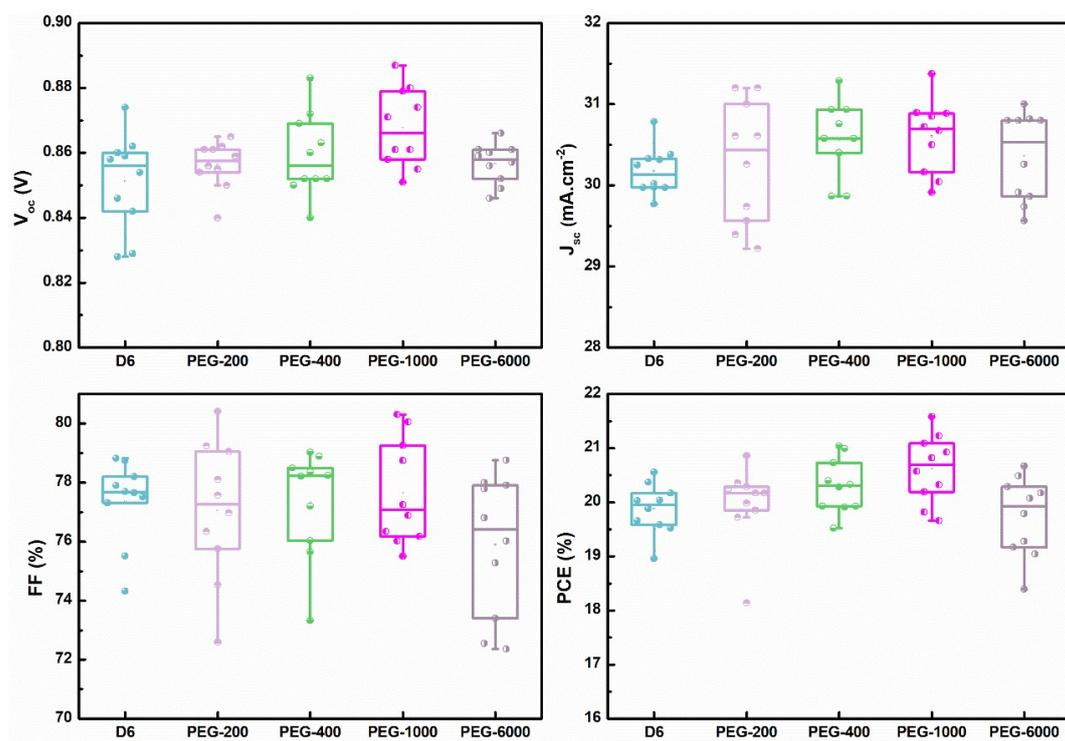
**Figure S12** Statistical results of devices based on 0.75 mg·mL<sup>-1</sup> PEG with different molecular weights using solvent etching process. The best device is the one with PEG molecular weight of 1000.
