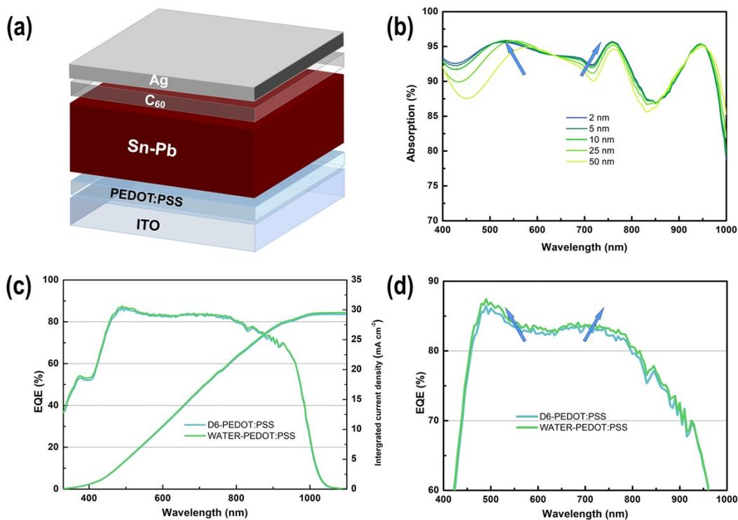
**Figure S14** (a) The device structure and materials used in the simulation. (b) The absorption of devices with different thicknesses of PEDOT:PSS is calculated by simulation. (c) EQE spectra of the devices using D6-PEDOT:PSS and WATER-PEDOT:PSS HTLs. The integrated photocurrents calculated from the EQE spectra are also shown. (d) Partial enlargements of (c). The actual value has the same trend as absorption of simulation, which indeed indicates the thinning HTL after solvent etching process.
