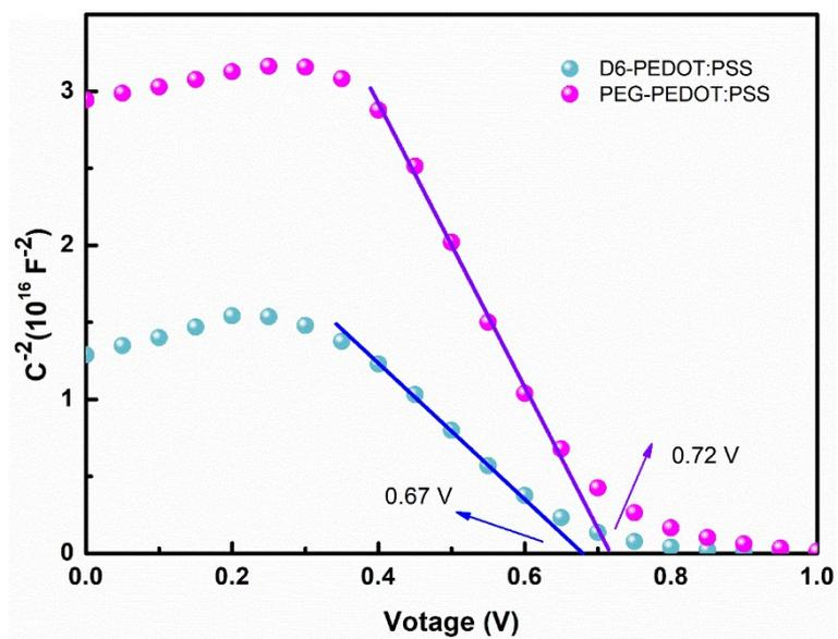
**Figure S11** C-V measurements of D6-PEDOT:PSS and PEG-PEDOT:PSS devices. The built-in voltage increases from 0.67 V of the reference to 0.72 V of the device using PEG-PEDOT:PSS.
