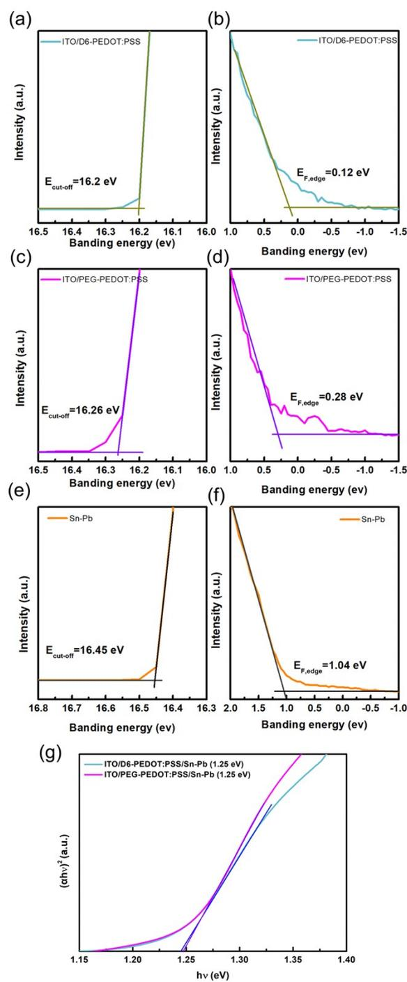
**Figure S10** The UPS spectra of (a) and (b) D6-PEDOT:PSS film; (c) and (d) PEG-PEDOT:PSS film; (e) and (f) Sn-Pb perovskite film. (g) Optical band gap of perovskite grown on different films.
