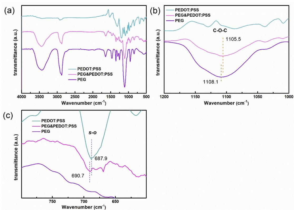
**Figure S2** (a) FTIR spectra of PEDOT:PSS, PEG and PEG&PEDOT:PSS mixture. (b) and (c) partial enlargements of (a). The peak shift demonstrates the interaction of PEG with PSS sulfonic acid groups.
