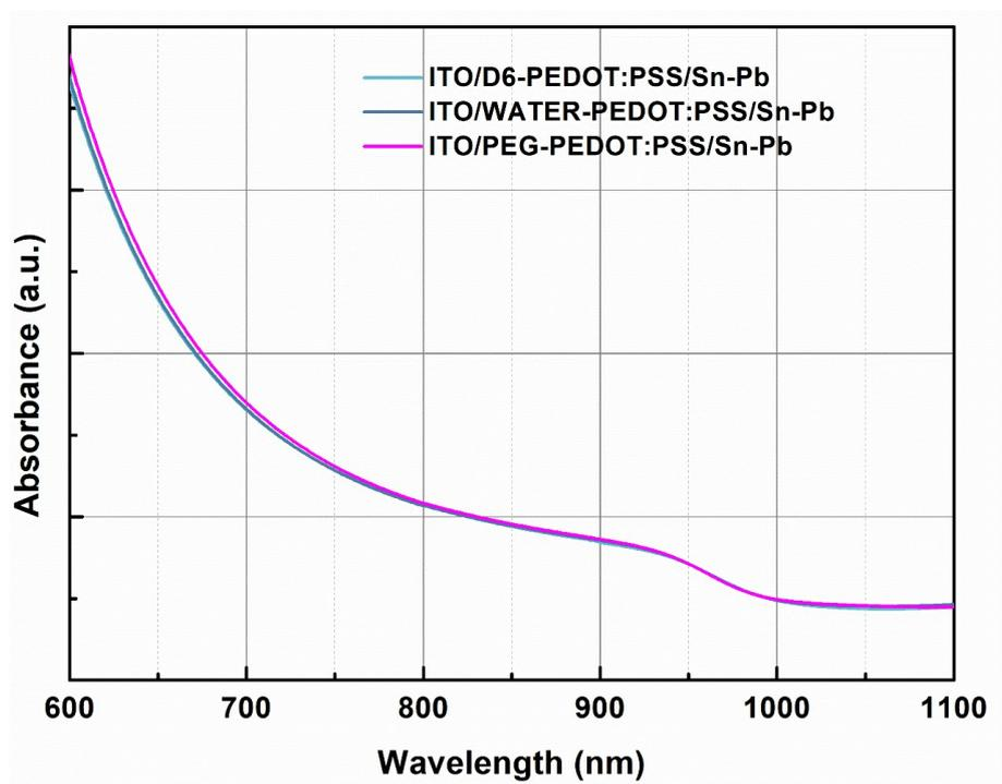
**Figure S9** Absorbance of perovskites grown on D6-PEDOT:PSS, WATER-PEDOT:PSS and PEG-PEDOT:PSS films.
