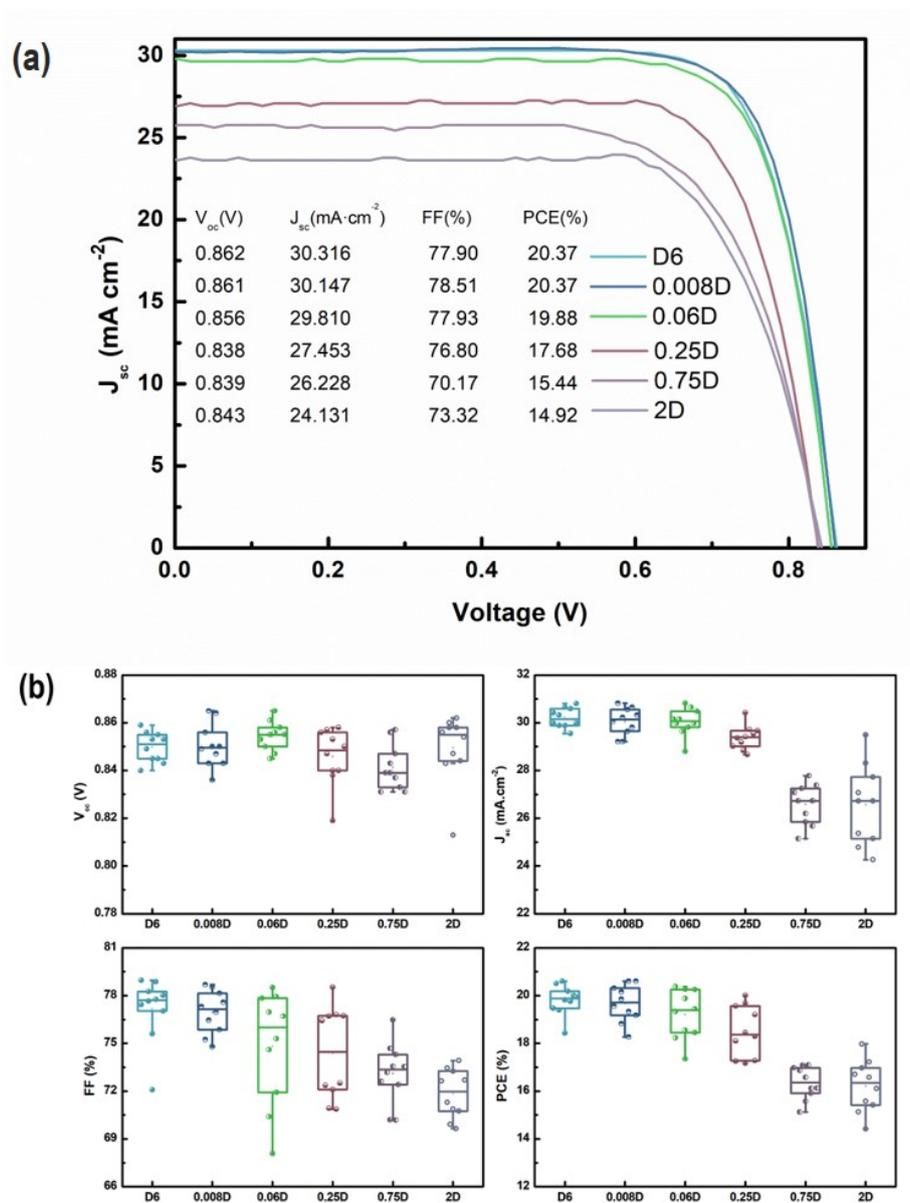
**Figure S13** (a) J-V curve parameters of devices doped with different concentrations of PEG. (b)  $V_{oc}$ ,  $J_{sc}$ , FF and PCE photovoltaic parameters statistics box of PEG doped devices with different concentrations. 0.008D, 0.06D, 0.25D, 0.75D, 2D correspond to 0.008, 0.06, 0.25, 0.75, and 2  $\text{mg}\cdot\text{mL}^{-1}$  PEG doped into the perovskite precursor. The trace PEG doping has little effect on the performance of device.
