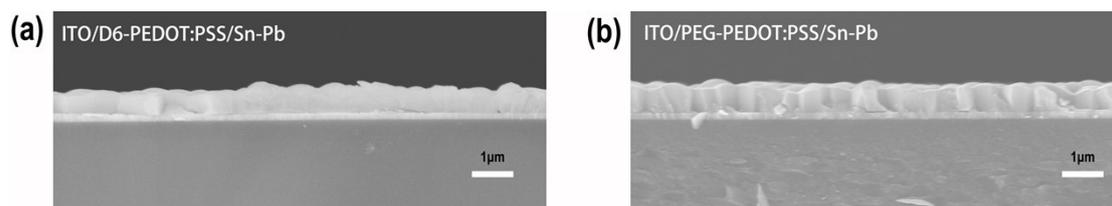
**Figure S7** Cross-sectional view of perovskite grown on different substrates. (a) D6-PEDOT:PSS, (b) PEG-PEDOT:PSS.
