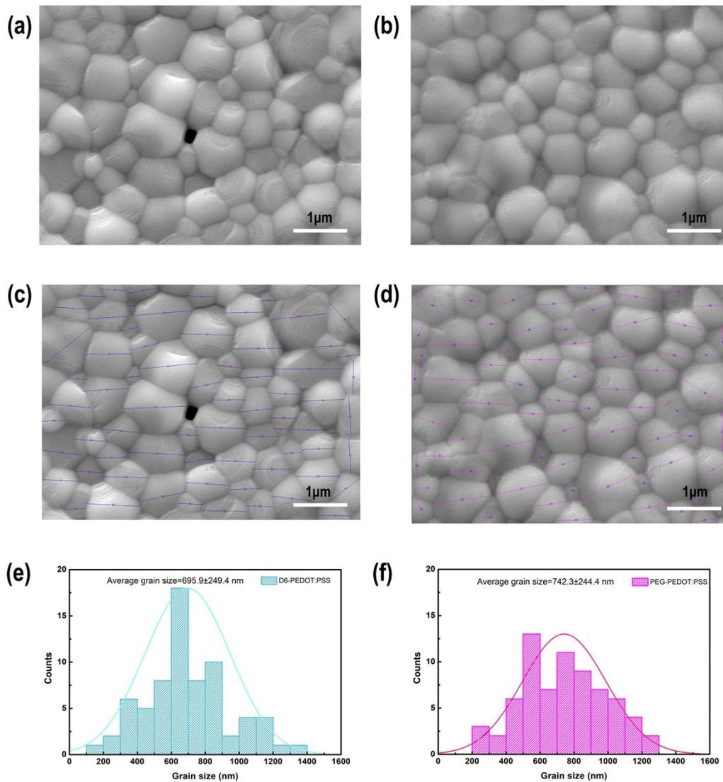
**Figure S6** FESEM and grain size statistics of perovskite grown on different films. (a), (c) and (e) D6-PEDOT:PSS; (b), (d) and (f) PEG-PEDOT:PSS.
