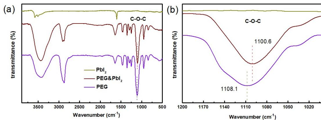
**Figure S5** (a) FTIR spectra of  $\text{PbI}_2$ , PEG and  $\text{PEG\&PbI}_2$  mixture. (b) Partial enlargements of (a), which reveal interaction between PEG and  $\text{PbI}_2$ .
