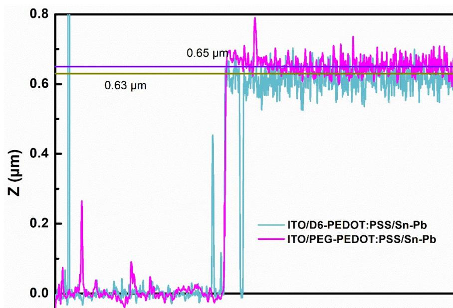
**Figure S8** The thicknesses of perovskite layers grown on D6-PEDOT:PSS and PEG-PEDOT:PSS films measured by step profiler.
