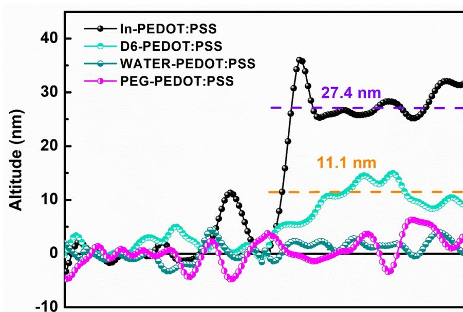
**Figure S3** AFM contour lines of different PEDOT:PSS layers profile for estimating film thickness. In-PEDOT:PSS was obtained by spin-coating commercial PEDOT:PSS solution. The thickness of the WATER-PEDOT:PSS and PEG-PEDOT:PSS films cannot be distinguished because its thickness is lower than the roughness of the substrate.
