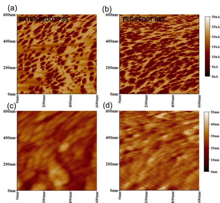
**Figure S4** C-AFM micro-zone conductivity (bias voltage of 0.1 V) images of (a) WATER-PEDOT:PSS and (b) PEG-PEDOT:PSS films. AFM images of (c) WATER-PEDOT:PSS and (d) PEG-PEDOT:PSS films.
