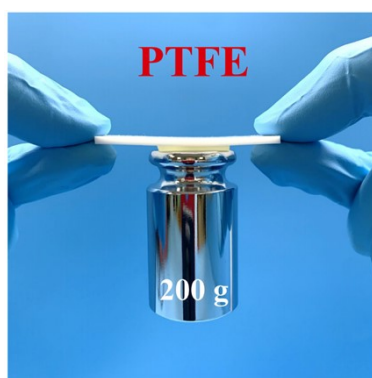
Figure S19. Adhesion behavior of \text{IG}_{0.825}\text{-AL}_{0.26\%}\text{-Zn}_{18\%} on PTFE.
