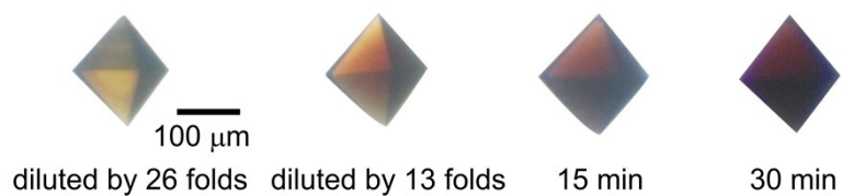
Fig. S34. Photographs of the UiO-68-SMe-Pt crystals after immersed in the transformer oil with different \text{C}_2\text{H}_2 concentration and varying periods.
