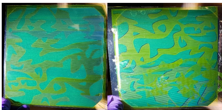
Figure S3. Prototypes demonstrating the versatile graphic design opportunities on solar cells with LDS materials (2 cm x 2 cm Si solar cells).
