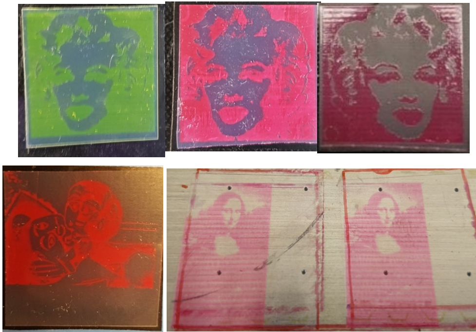
Figure S7 Photographs demonstrating the different artistic design opportunities with an inkjet printer on ETFE film using LDS materials
