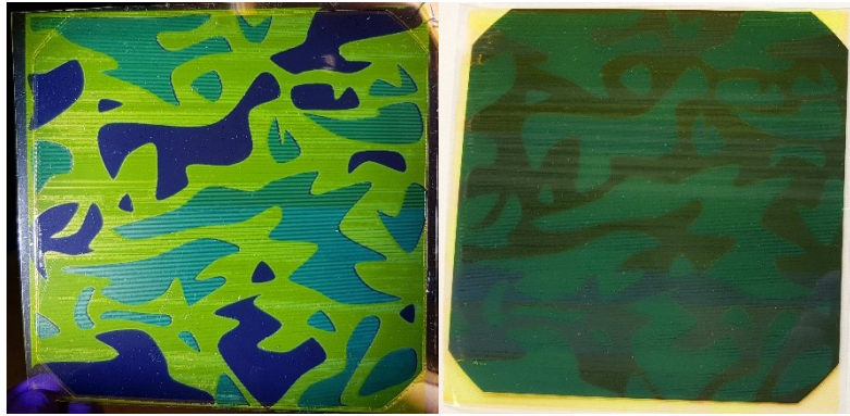
Figure S4. Prototypes demonstrating the versatile graphic design opportunities on solar cells with LDS materials (12.5 cm x 12.5 cm Sun power solar cells).
