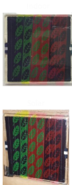
Figure S5. CIS solar cells laminated with graphically printed ETFE foil with LDS materials under the sun (top) and UV-light illumination (bottom) and comparison of the efficiency of the bare cell and after lamination with luminescent coating. The efficiency of the cell with the luminescent coating is only 2% lower than a bare cell.
