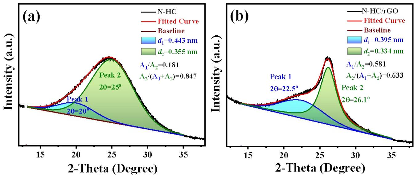
Figure S2. Fitting of XRD (002) peak of (a) N-HC and (b) N-HC/rGO.
