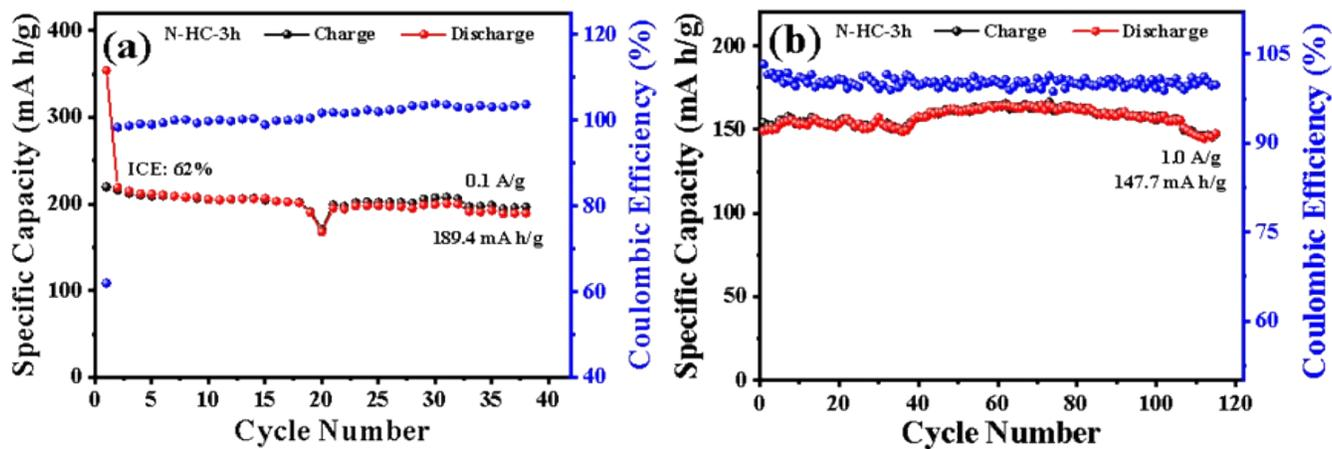
Figure S9. Cycling performance of N-HC-3h electrode at (a) 0.1 and (b) 1.0 A g<sup>-1</sup>.
