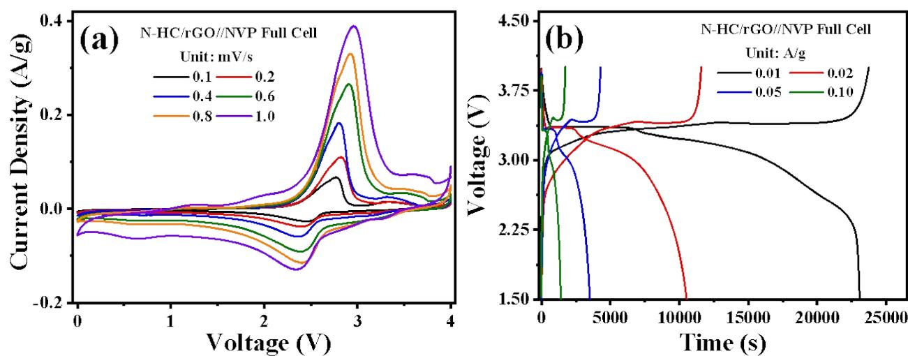
Figure S12. Electrochemical performance of N-HC/rGO//NVP full cell. (a) CV curves at various sweep rates from 0.1 to 1.0 mV s<sup>-1</sup>; (b) Rate capability at various current densities from 0.01 to 0.1 A g<sup>-1</sup>.
