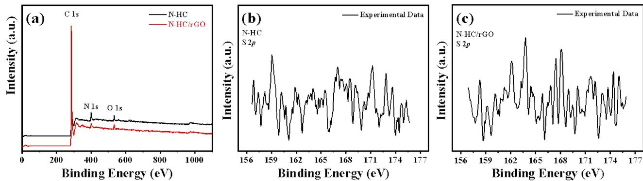
Figure S4. (a) XPS survey spectra of N-HC and N-HC/rGO. XPS spectra of S 2p of (b) N-HC and (c) N-HC/rGO.
