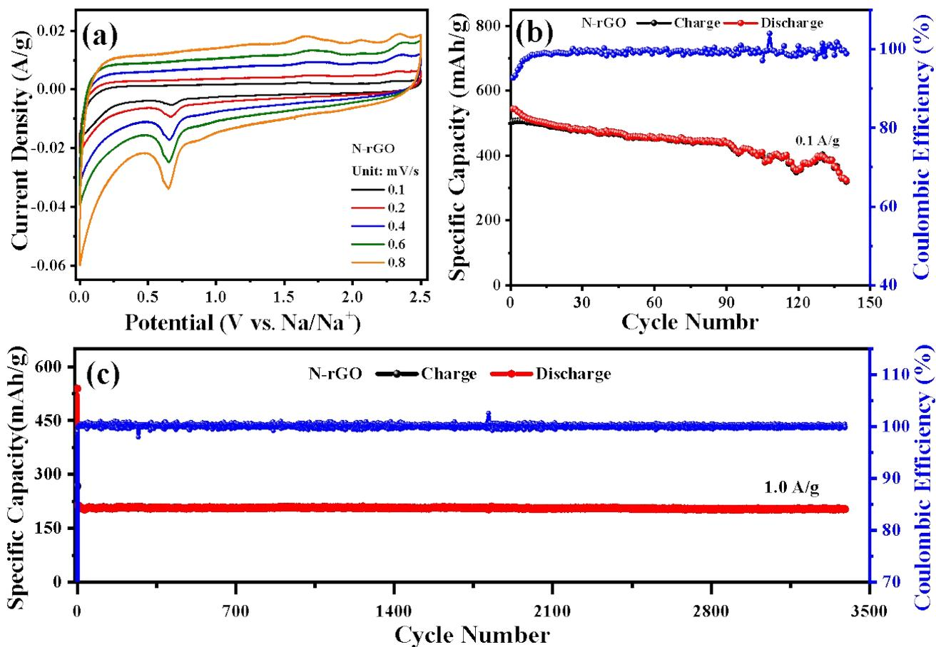
Figure S7. Electrochemical performance of N-rGO electrode. (a) CV curves at different scan rates; Cycling test of N-rGO electrode at (b) 0.1 and (c) 1.0 A g<sup>-1</sup>.
