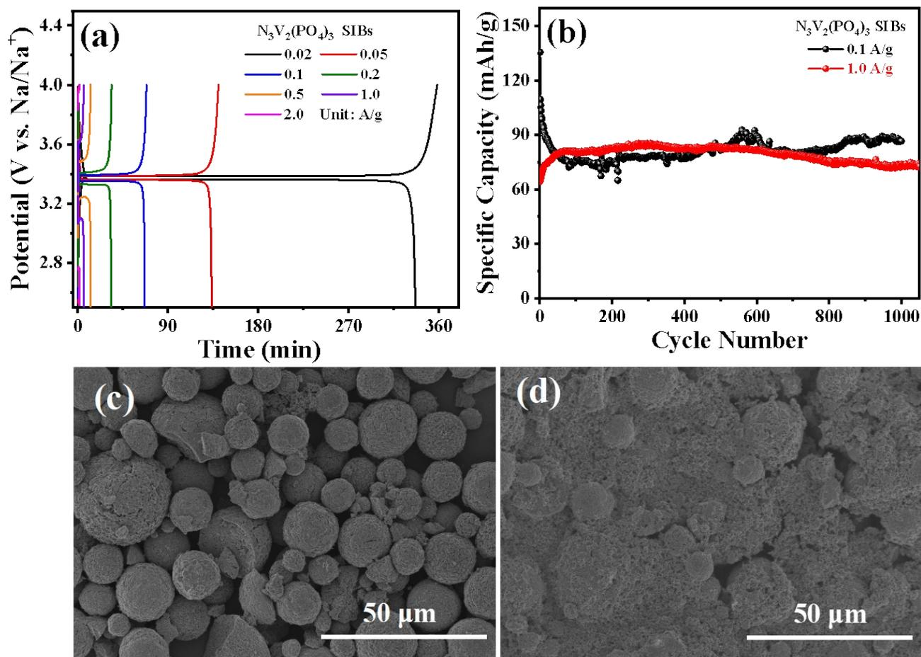
Figure S11. Electrochemical performance of NVP electrode. (a) Rate capability at various current densities from 0.02 to 2.0 A g<sup>-1</sup>; (b) Cycling performances at 0.1 and 1.0 A g<sup>-1</sup>; SEM images of NVP (c) before cycling and (d) after cycling at 0.1 A g<sup>-1</sup> after 50 cycles.
