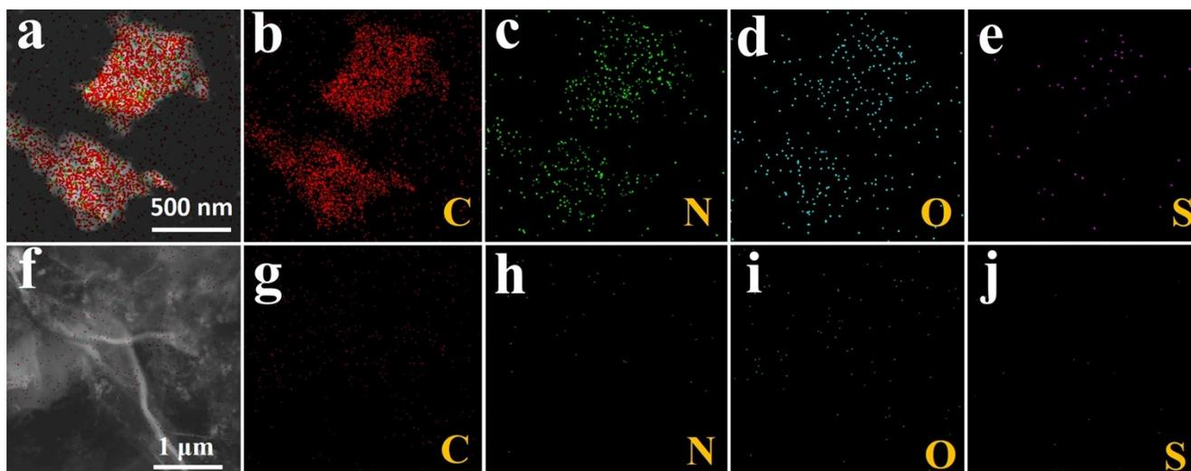
Figure S3. EDS elemental mappings of (a–e) N-HC and (f–j) N-HC/rGO.
