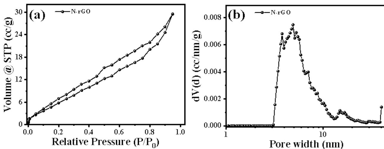
Figure S6. (a)  $N_2$  adsorption/desorption and (b) corresponding pore size distribution by NLDFT calculation of N-rGO.
