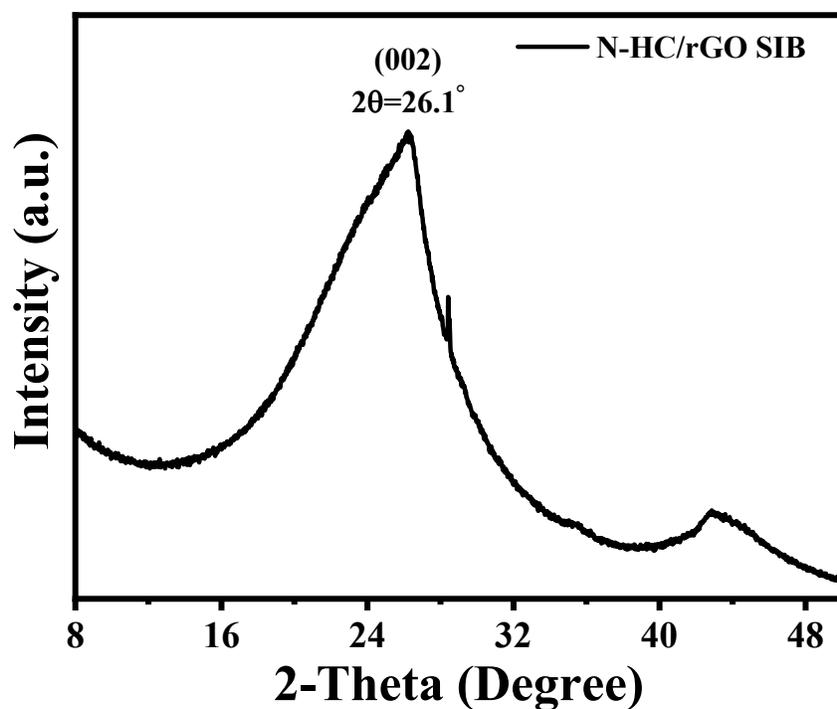
Figure S10. In-situ XRD result of N-HC/rGO electrode when discharged at 0.1 A g<sup>-1</sup>.
