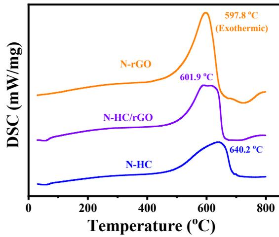
Figure S1. DSC results of N-HC, N-rGO and N-HC/rGO.
