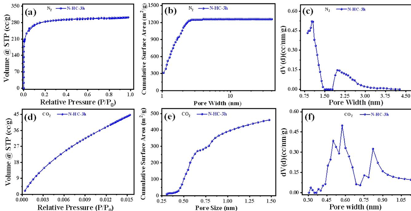
Figure S5. (a)  $N_2$  adsorption/desorption and (d)  $CO_2$  adsorption measurements of N-HC-3h sample; SSA and pore size distribution determined by NLDFT calculation of (b)  $N_2$  adsorption/desorption and (e)  $CO_2$  adsorption measurements; Pore size distribution determined by NLDFT calculation for (c)  $N_2$  adsorption/desorption and (f)  $CO_2$  adsorption measurements.
