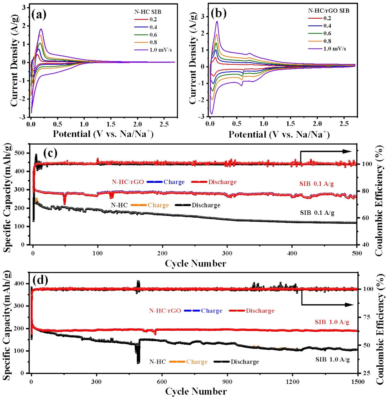
Figure S8. CV curves of (a) N-HC and (b) N-HC/rGO; Cycling test at (c) 0.1 A g<sup>-1</sup> and (d) 1.0 A g<sup>-1</sup> of N-HC and N-HC/rGO, respectively.
