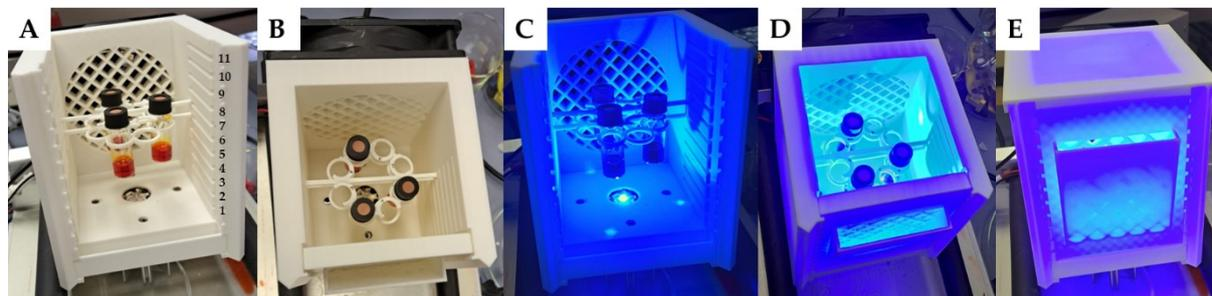
Figure S1: Photoreactor used for hydrogen evolution experiments with 1 mL of aqueous methyl orange solution in three 4 mL LABSOLUTE 7613421 clear glass screw neck vials. (A) Side view of reactor including slot position indication. (B): Top view of reactor including side shielding. (C): Side view of reactor under LED irradiation. (D): Top view of reactor under LED irradiation. (E): Photoreactor including top- and side shielding under operation.
