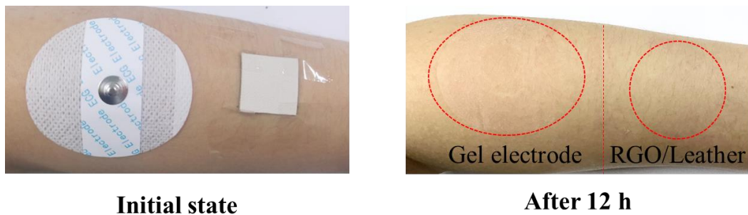
Fig. S11. The gel electrode and leather electrode were covered on the arm for 12 h and then removed from the arm. The skin under the gel electrode became greasy, while the skin under the leather electrode is changed.
