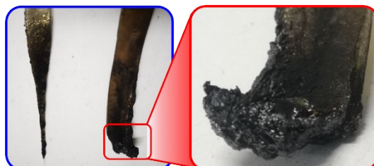
Figure S15. Digital photographs of char residue after strip sample testing for BPA-PC and PP-BPT.
