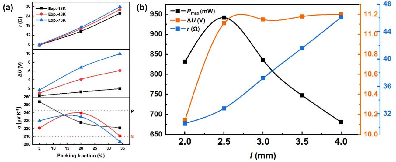
**Fig. S4** (a) Packing fraction dependence of  $r$ ,  $\Delta U$  and average Seebeck coefficient values of 50-Tcs ( $f=5\%$ ), 200-Tcs ( $f=20\%$ ) and 338-Tcs ( $f=34\%$ ) TEGs at different  $\Delta T$ . (b) The leg height ( $l$ ) dependence of  $P_{\text{max}}$ ,  $\Delta U$  and  $r$  of 338-Tcs TEG between 293K and 366K.
