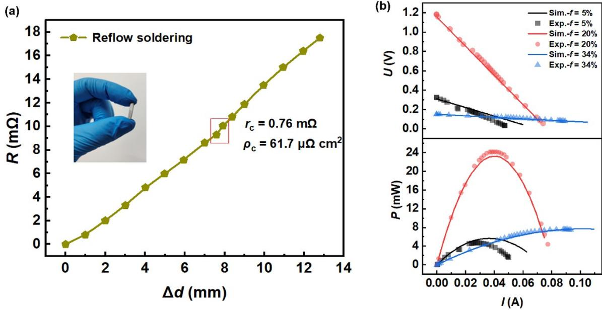
**Fig. S3** (a) The electrical contact resistance ( $r_c$ ) of typical reflow soldering sample, and (b) the simulation and experimental value of TEGs ( $f$ : 5%, 20% and 34%).
