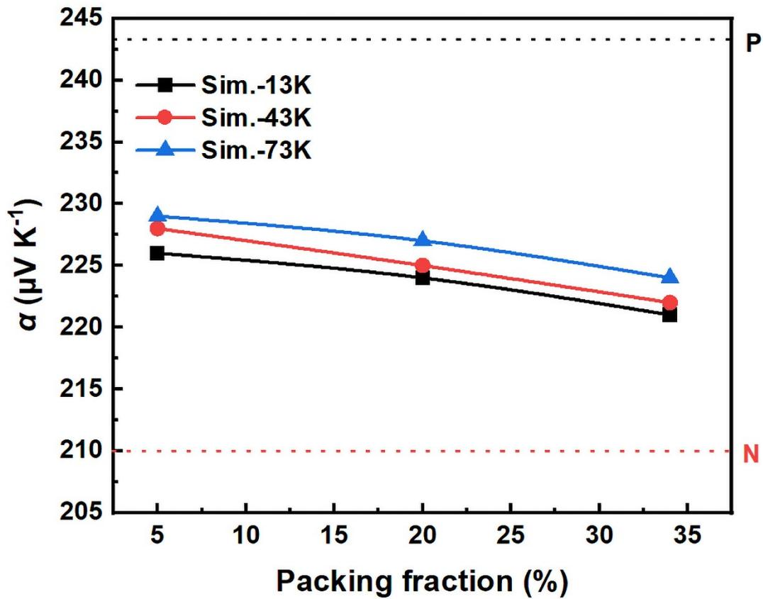
**Fig. S2** Packing fraction dependence of average Seebeck coefficient values of 200-Tcs ( $f = 20\%$ ), 50-Tcs ( $f = 5\%$ ) and 50-Tcs ( $f = 34\%$ ) TEGs at different  $\Delta T$ .
