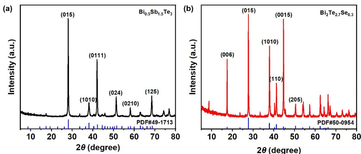
**Fig. S1** Phase characterization diagram of commercial  $\text{Bi}_2\text{Te}_3$ -based thermoelectric materials. The X-ray diffraction patterns of (a) p-type and (b) n-type materials.
