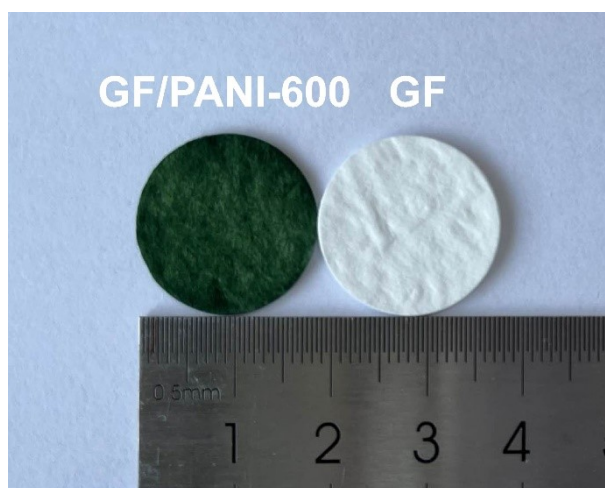
Fig. S2 Digital photographs of the GF/PANI-600 (left) and the pristine GF (right) separator.
