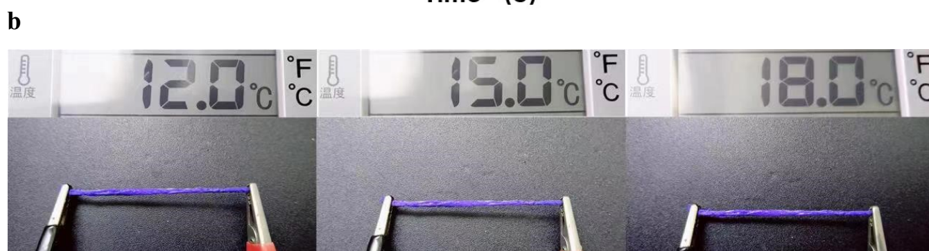
Fig. S15. Temperature of the composite Ti@Ecoflex/CB fiber sensors with 7.5 wt.% of CB NPs with 5% cyclic strain applied at an ambient temperature of 16 °C and 3000 cycles ( a ), and 50% stretching exhibits the same color at different ambient temperatures ( b ).
