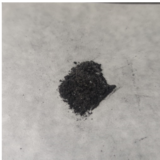
Fig. S5. Digital image of the decomposed LATP powder obtained from the surface of the reacted LATP pellets.
