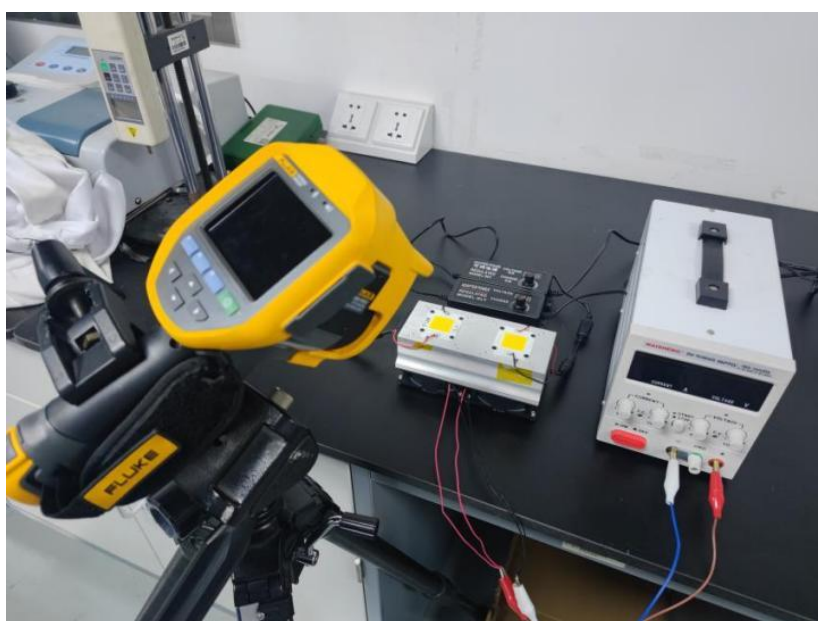
Figure S9. Photography of TIM performance test system.
