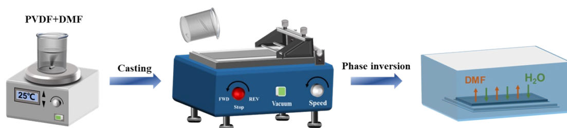
Fig. S1 Schematic illustration for the fabrication process of the Negative-Charge Separator (NCS).
