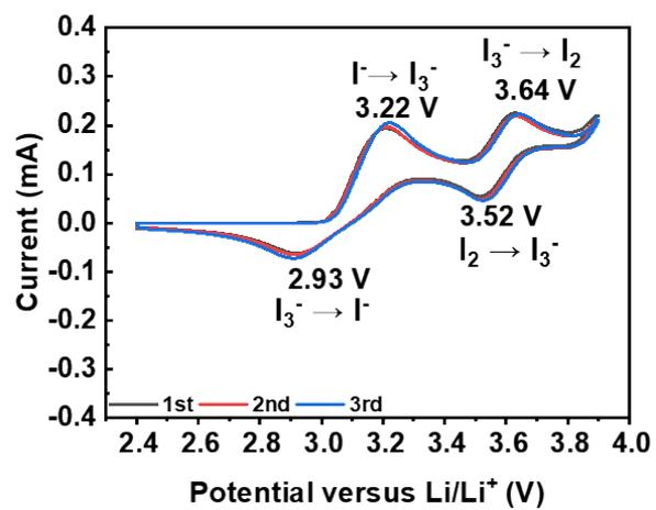
**Fig. S7** Three-electrode CV curves for an electrolyte composed of 0.2 M LiI + 1 M LiNO<sub>3</sub>/N,N-dimethylacetamide.
