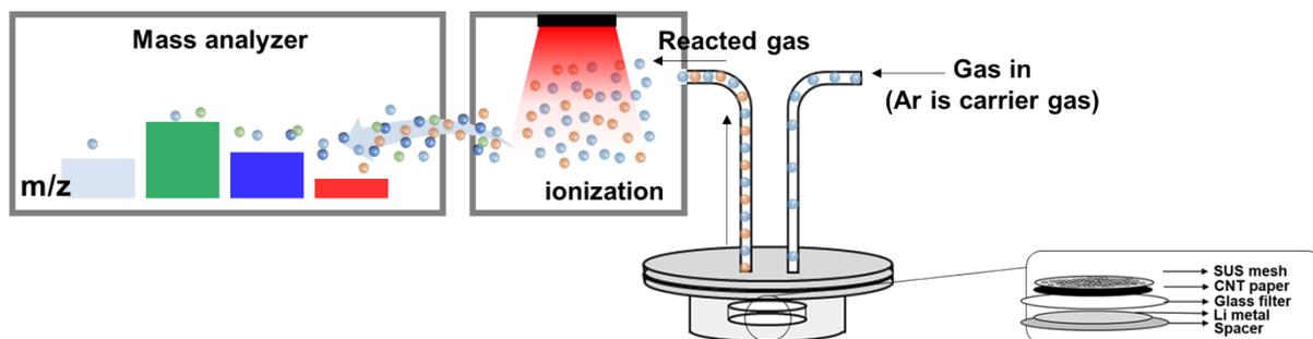
**Fig. S1.** A schematic illustration representing the setup of the DEMS and the structure of a custom designed HS air type cell.
