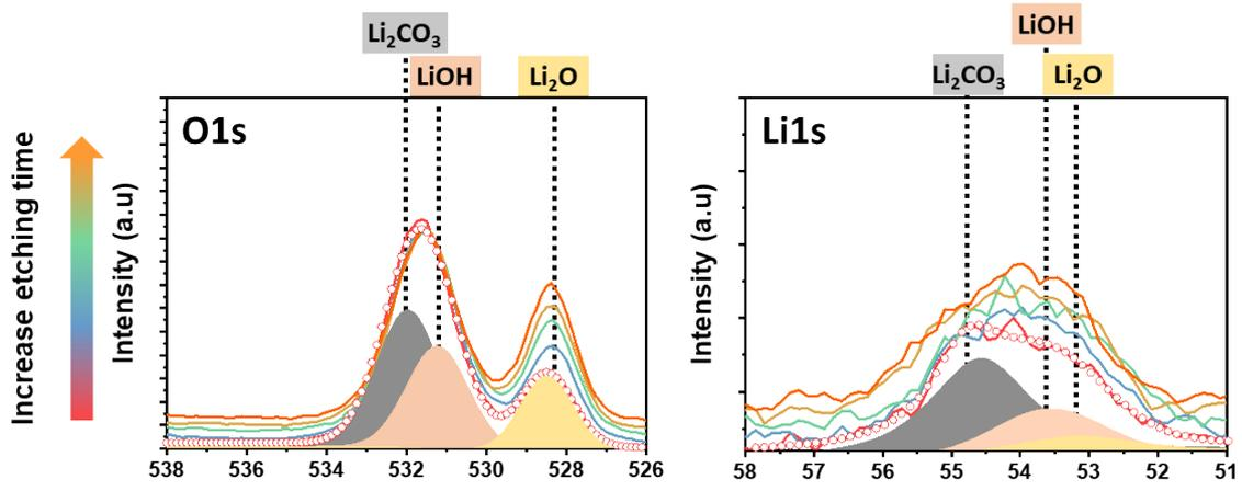
**Fig. S3** XPS depth profiles of Li metal after 25 cycles in an Li-O<sub>2</sub> cell using 1 M LiNO<sub>3</sub>/N,N-dimethylacetamide electrolyte.
