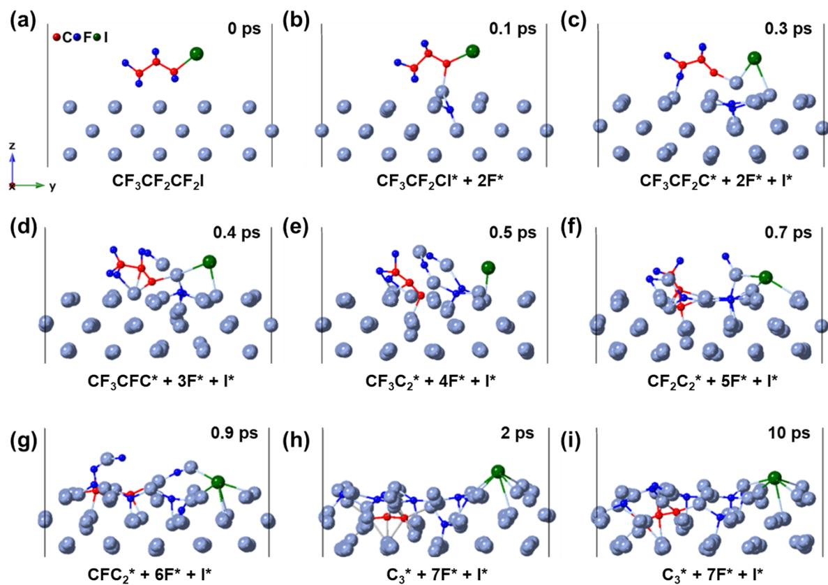
**Fig. S5** *Ab initio* molecular dynamics calculations at 300 K of the dissociation of  $\text{CF}_3(\text{CF}_2)_2\text{I}$  on the Li(100) surface.
