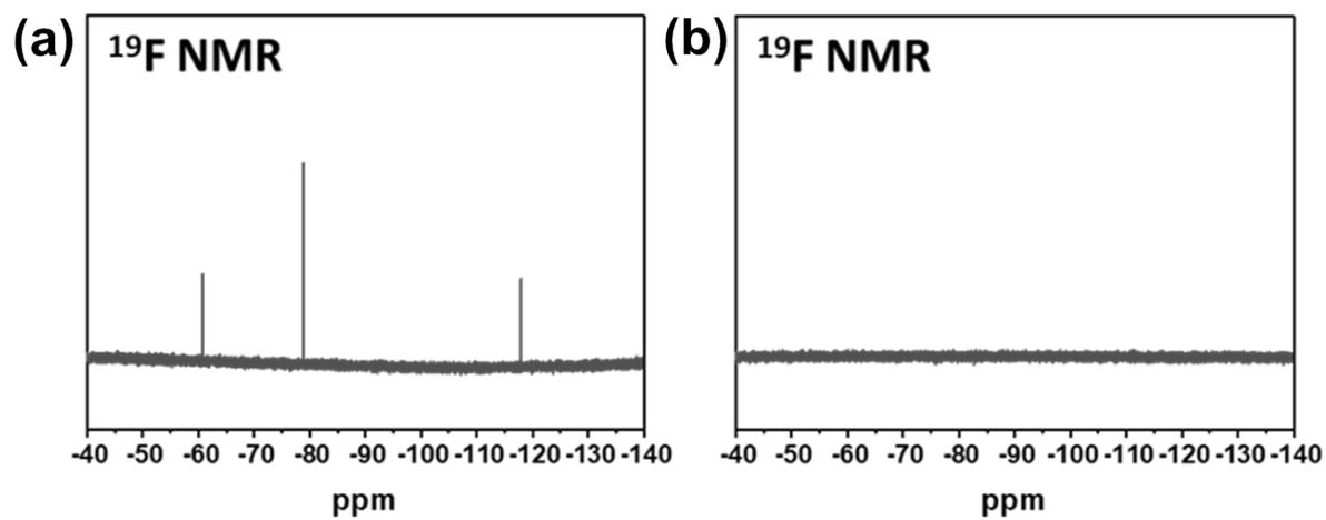
**Fig. S8.** The  $^{19}\text{F}$  NMR spectrum of 0.2 M  $\text{CF}_3(\text{CF}_2)_2\text{I}$  + 1 M  $\text{LiNO}_3/\text{DMA}$  (a) before and (b) after reaction with Li metal.
