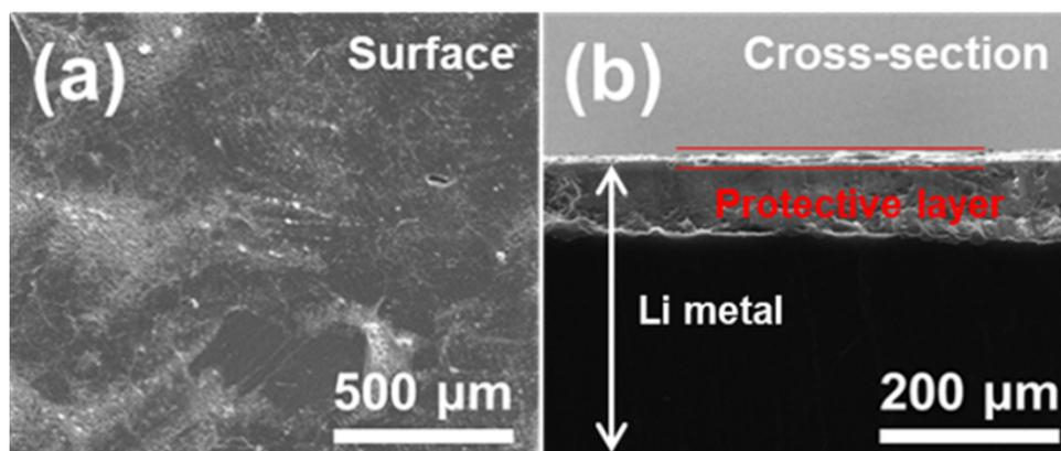
**Fig. S15.** SEM images of (a) surface and (b) a cross-section of Li metal after discharging to a capacity of  $5 \text{ mA h cm}^{-2}$  using  $0.2 \text{ M CF}_3(\text{CF}_2)_2\text{I} + 1 \text{ M LiNO}_3/\text{N,N-dimethylacetamide}$  electrolyte.
