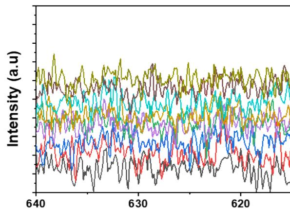
**Fig. S6** XPS depth profiles of I 3d spectra of Li metal after storage in  $\text{CF}_3(\text{CF}_2)_2\text{I}$ -containing electrolyte.
