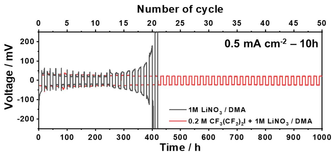
**Fig. S10.** Voltage profiles of a symmetric Li/Li cell cycled in 1 M LiNO<sub>3</sub>/N,N-dimethylacetamide (DMA) (black) and 0.2 M CF<sub>3</sub>(CF<sub>2</sub>)<sub>2</sub>I + 1 M LiNO<sub>3</sub>/DMA (red) at a current density of 0.5 mA cm<sup>-2</sup> under O<sub>2</sub>.
