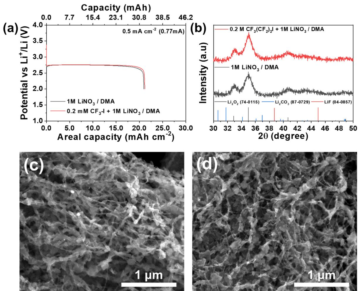
**Fig. S9.** (a) Discharge–charge curves of Li–O<sub>2</sub> cell using 1 M LiNO<sub>3</sub>/N,N-dimethylacetamide (DMA) (black) and 0.2 M CF<sub>3</sub>(CF<sub>2</sub>)<sub>2</sub>I + 1 M LiNO<sub>3</sub> in DMA (red) at a current density of 0.5 mA cm<sup>-2</sup> until 2.0 V. (b) XRD patterns of the discharged cathode in 1 M LiNO<sub>3</sub>/DMA and 0.2 M CF<sub>3</sub>(CF<sub>2</sub>)<sub>2</sub>I + 1 M LiNO<sub>3</sub>/DMA and (c), (d) the respective SEM images.
