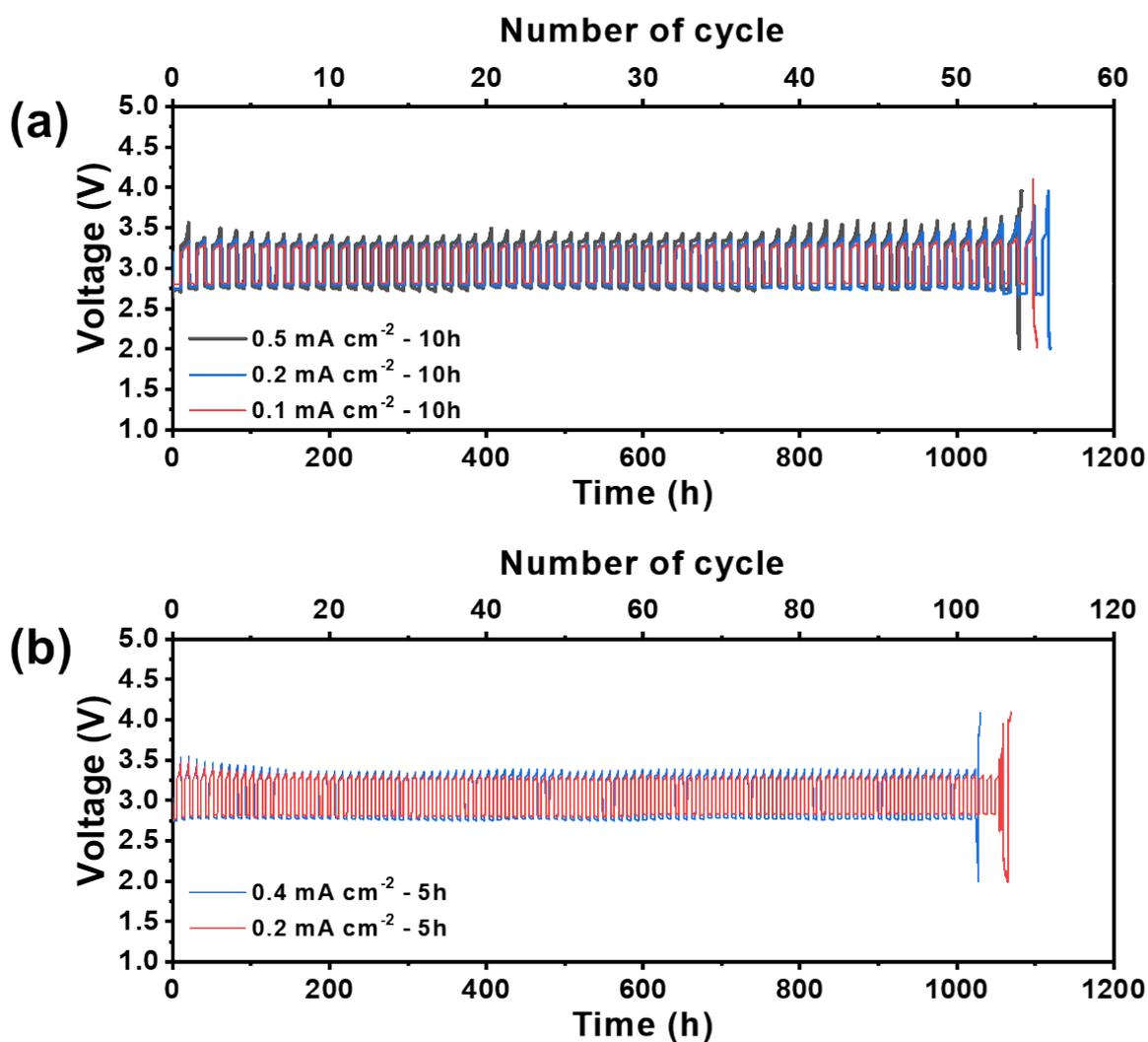
**Fig. S11.** Time–voltage profile of Li–O<sub>2</sub> cell using 0.2 M CF<sub>3</sub>(CF<sub>2</sub>)<sub>2</sub>I + 1 M LiNO<sub>3</sub>/N,N-dimethylacetamide under various current densities with a time limit of (a) 10 h and (b) 5 h.
