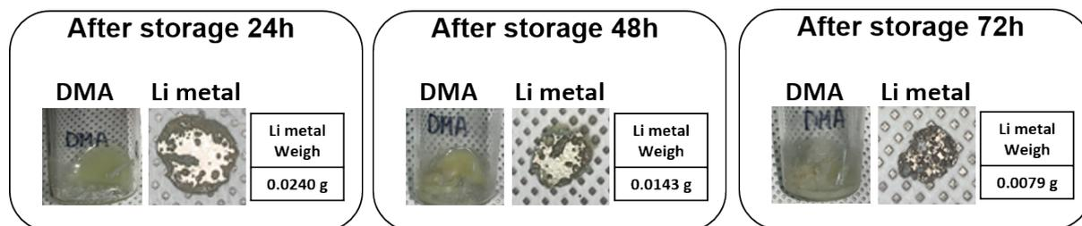
**Fig. S4** Digital photos of N,N-dimethylacetamide (DMA) and Li and the obtained Li metal weight after storage of Li metal in DMA for different time.
