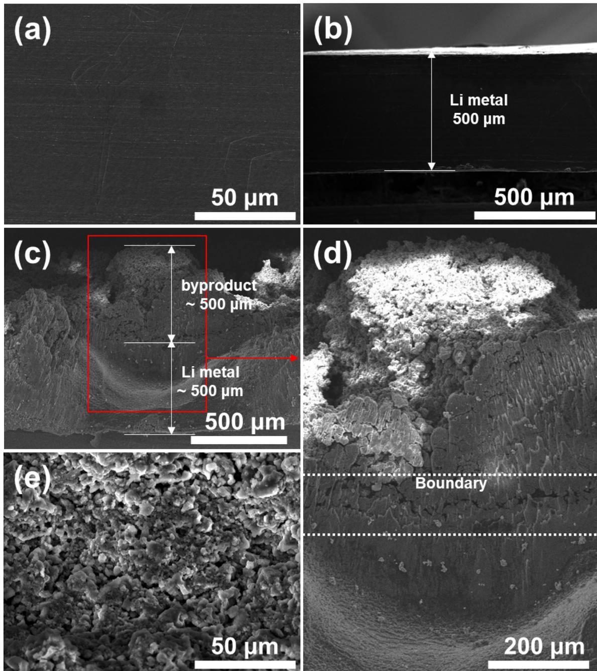
**Fig. S14.** SEM images of (a) surface and (b) a cross-section of pristine Li metal. SEM images of (c) a cross-section and (e) surface of the Li metal after 25 cycles in an Li–O<sub>2</sub> cell using 1 M LiNO<sub>3</sub>/N,N-dimethylacetamide electrolyte. (d) High-magnification SEM image of (c).
