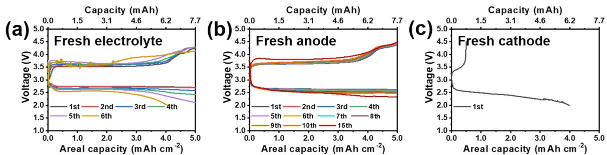
**Fig. S2.** Discharge-charge curves of rebuild Li-O<sub>2</sub> cells using (a) fresh electrolyte, (b) fresh anode, and (c) fresh cathode.
