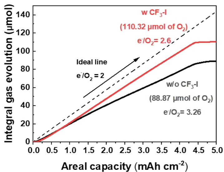
**Fig. S13.** Integral gas evolution for O<sub>2</sub> determined by in situ differential electrochemical mass spectroscopy measurements using 1 M LiNO<sub>3</sub>/N,N-dimethylacetamide (DMA) (black) and 0.2 M CF<sub>3</sub>(CF<sub>2</sub>)<sub>2</sub>I + 1 M LiNO<sub>3</sub>/DMA (red) during the charging process. The dashed line indicates the ideal oxidation of Li<sub>2</sub>O<sub>2</sub> with an e<sup>-</sup>/O<sub>2</sub> value of 2.
