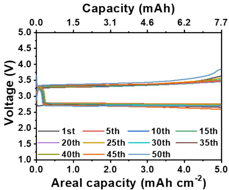
**Fig. S12.** Discharge-charge curves of Li-O<sub>2</sub> cell rebuild using fresh 0.2 M CF<sub>3</sub>(CF<sub>2</sub>)<sub>2</sub>I + 1 M LiNO<sub>3</sub>/N,N-dimethylacetamide electrolyte.
