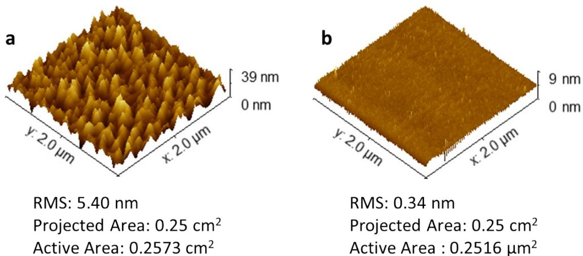
**Fig. S1.** Tribological analysis of the (a) PdSiAu+Si/SiO<sub>2</sub> and (b) MLGR+PdSiAu+Si/SiO<sub>2</sub> using atomic force microscopy. The room mean square (RMS) roughness, projected and active areas are provided below the corresponding images.
