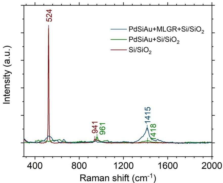
**Fig S2.** Raman spectroscopy of MLGR+PdSiAu+Si/SiO<sub>2</sub>, PdSiAu+Si/SiO<sub>2</sub> and Si/SiO<sub>2</sub> showing the full spectra.
