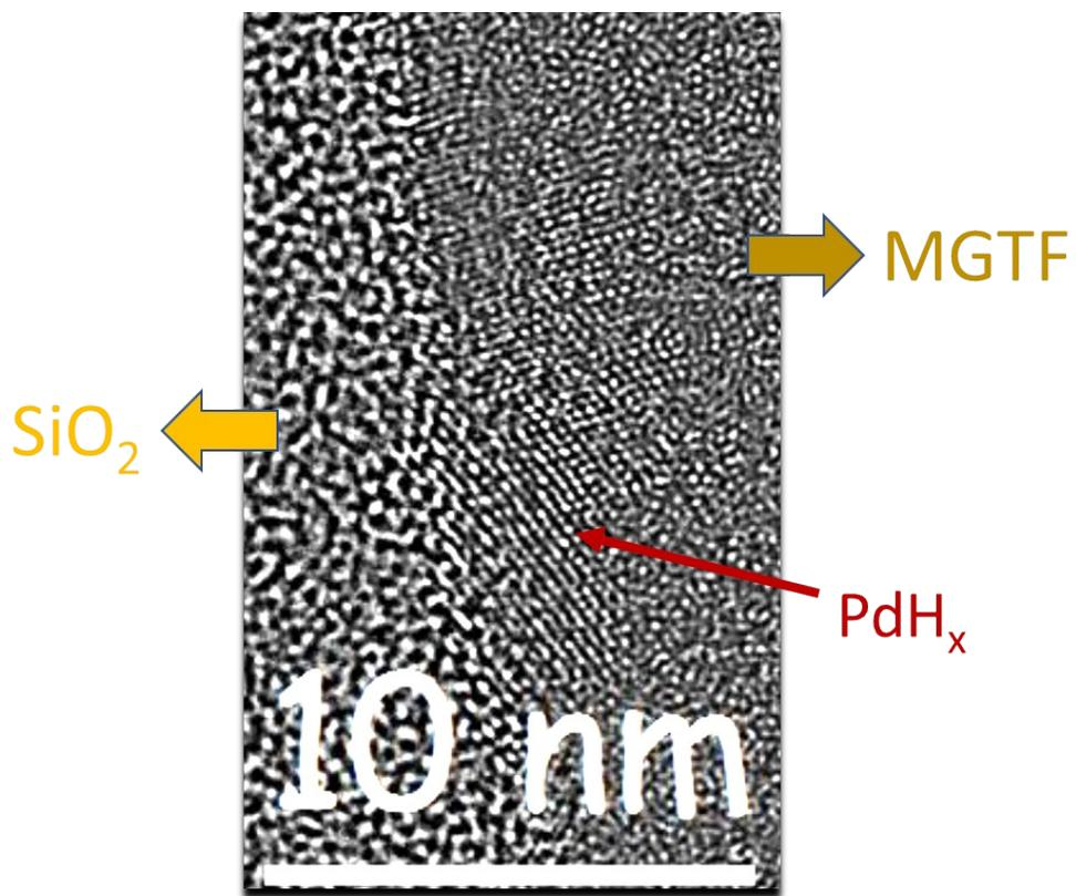
**Fig. S6.** Close-up HRTEM image of the MGTF - Si/SiO<sub>2</sub> interface showing PdH<sub>x</sub> nanocrystals.
