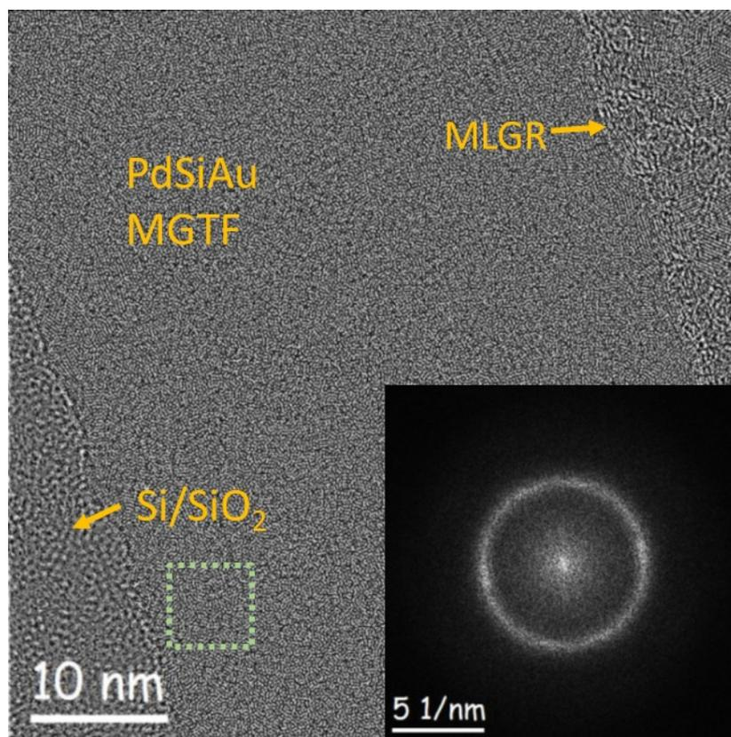
**Fig. S7.** HRTEM imaging of the entire layer of the as-sputter deposited MLGR+PdSiAu layers on Si/SiO<sub>2</sub> substrate and FFT pattern of the region indicated by the light green square.
