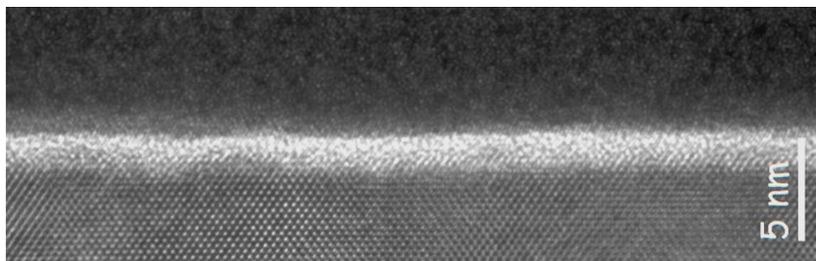
**Fig. S8.** HRTEM imaging of the PdSiAu MGTF and Si/SiO<sub>2</sub> interface
