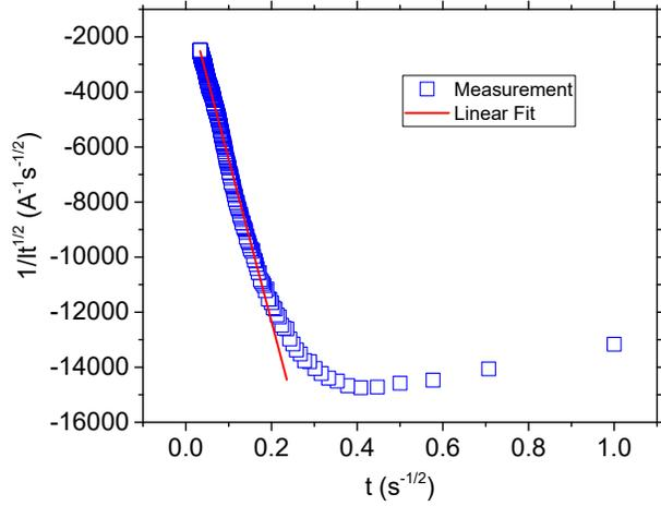
**Fig. S3.** Plot of  $1/I t^{1/2}$  vs.  $t$  for MLGR+PdSiAu+Si/SiO<sub>2</sub>. The open blue squares and the red line depict measured data and the best linear fit. The slope and y-intercept of the linear fit correspond,
