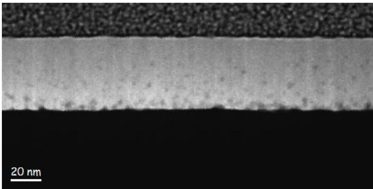
**Fig. S9.** HAADF imaging after hydrogenation of MLGR+PdSiAu+Si/SiO<sub>2</sub>; scattered black regions correspond to nanovoids formed during hydrogen-metal interactions.
