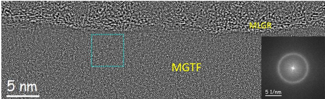
**Fig. S5.** HRTEM imaging of the as-sputter deposited MLGR+PdSiAu layers and FFT pattern of the region indicated by the cyan square.
