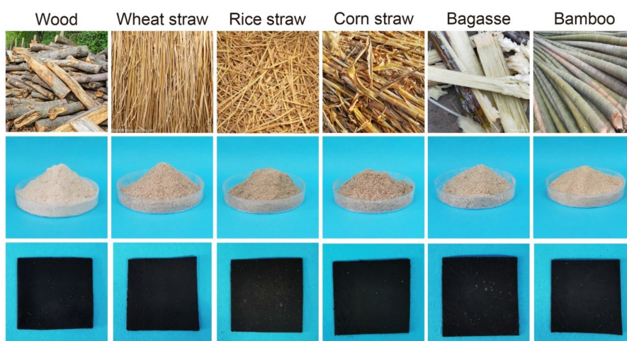
Fig. S9 The universality of the LB preparation method. The LB can be made from various biomass feedstocks, including wood, wheat straw, rice straw, corn straw, bagasse, and bamboo, demonstrating the strong universality of this approach ( 2 \times 2 \times 0.05 \text{ cm}^3 ).
