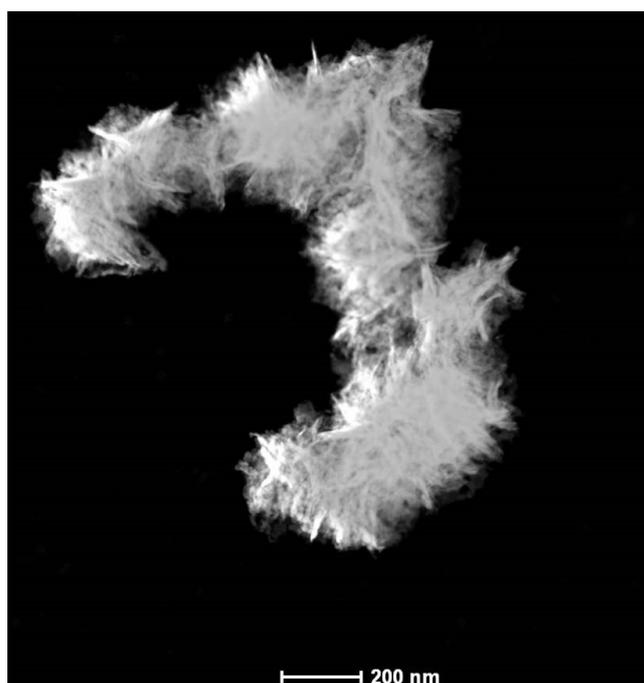
**Fig.S3** STEM image of the metallene-like PdRu-RuO<sub>2</sub> nanostructure.
