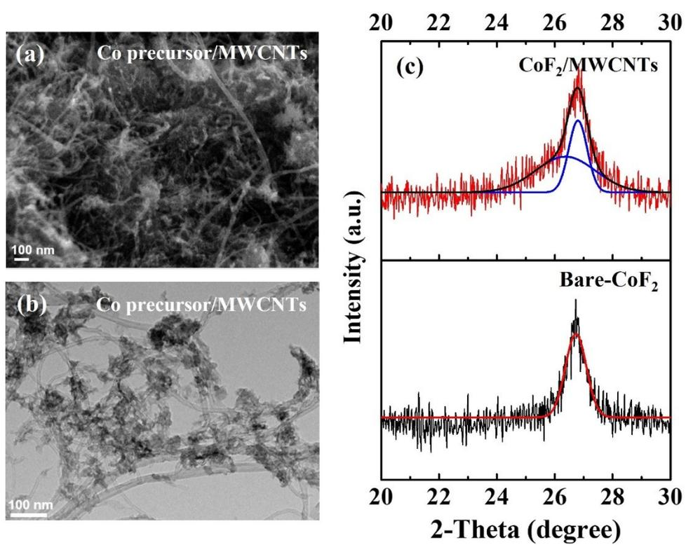
**Fig. S2** (a) SEM and (b) TEM image of Co precursor/MWCNTs. (c) A partial magnification of XRD patterns of CoF<sub>2</sub>/MWCNTs and bare-CoF<sub>2</sub>.
