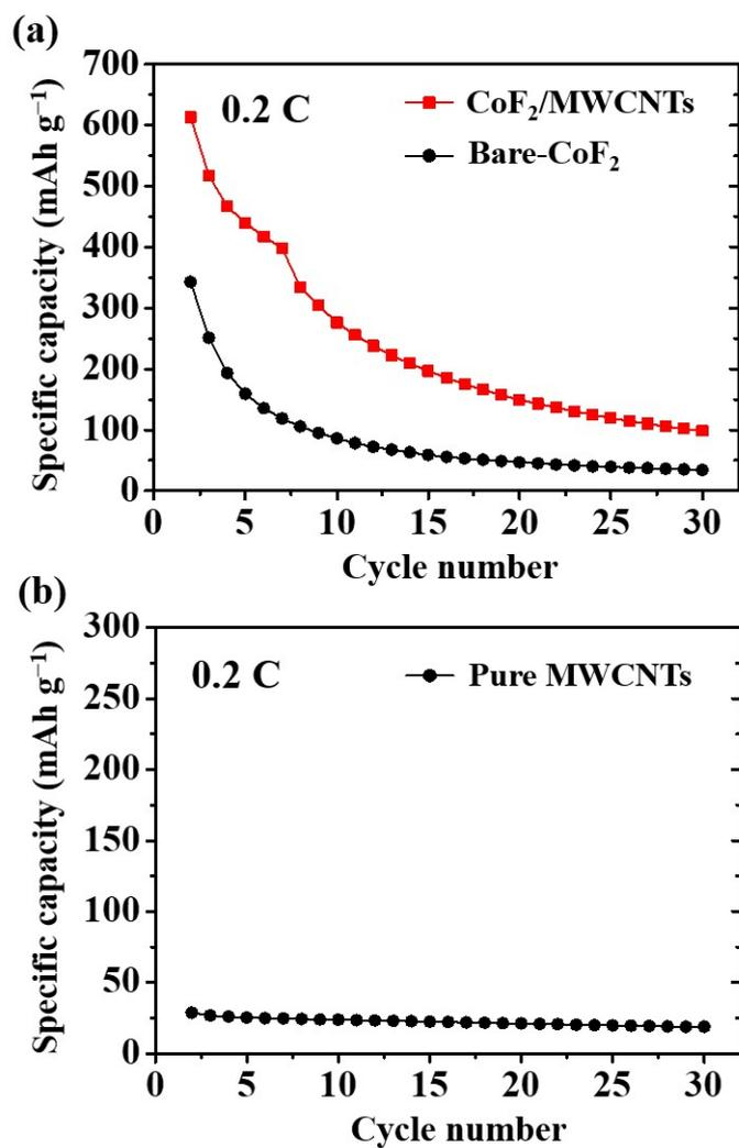
**Fig. S5** Cycle properties of (a) CoF<sub>2</sub>/MWCNTs and bare-CoF<sub>2</sub> and (b) pure MWCNTs. The specific capacities of pure MWCNTs are calculated based on the target mass of MWCNTs (30 wt%).
