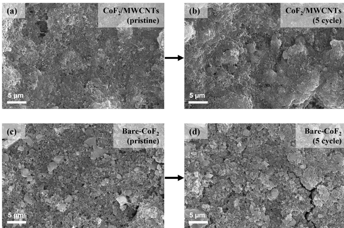
**Fig. S6** SEM images of (a, b) CoF<sub>2</sub>/MWCNTs and (c, d) bare-CoF<sub>2</sub> electrodes: (a, c) Before cycling (pristine) and (b, d) after the 5<sup>th</sup> cycle at 0.5 C.
