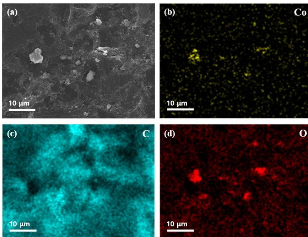
**Fig. S10** Post-mortem analysis of clogged parts of the separator after the 100<sup>th</sup> cycle (electrode: CoF<sub>2</sub>/MWCNTs) in FEC/EMC electrolyte: (a) SEM image and EDS elemental mapping of (b) cobalt, (c) carbon, and (d) oxygen.
