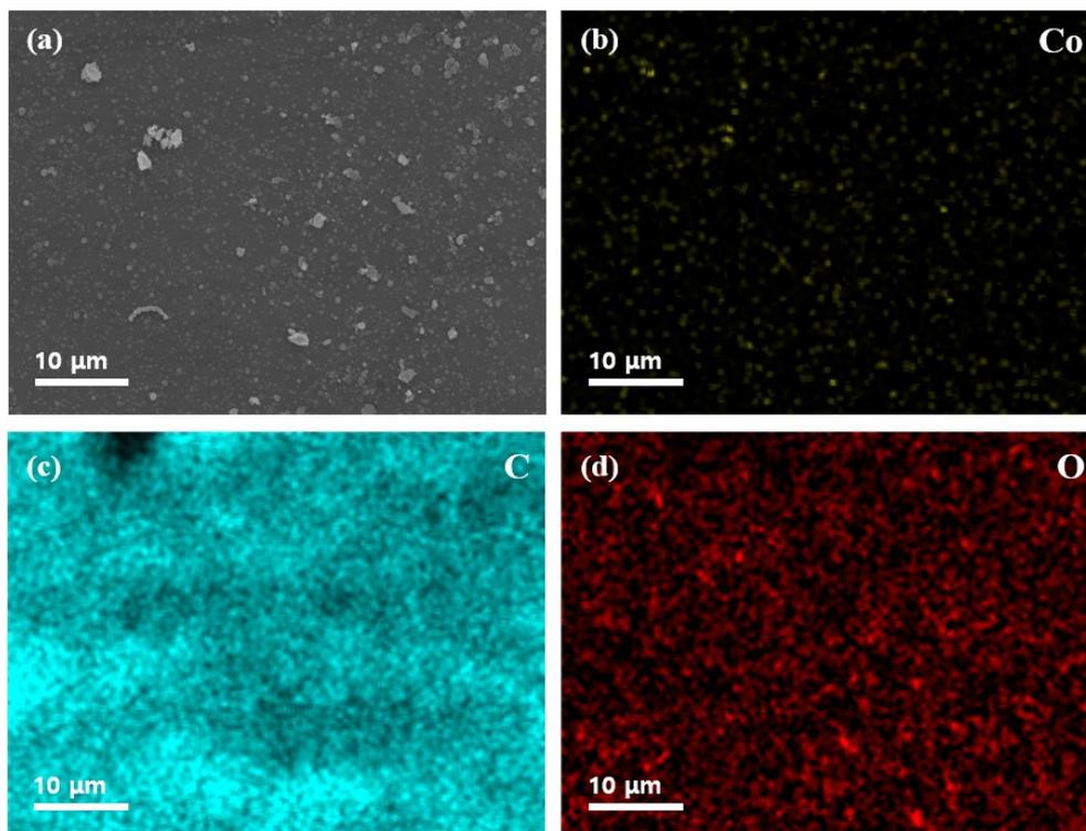
**Fig. S12** Post-mortem analysis of clogged parts of the separator after the 500<sup>th</sup> cycle (electrode: 50A-CoF<sub>2</sub>/MWCNTs) in FEC/EMC electrolyte: (a) SEM image and EDS elemental mapping of (b) cobalt, (c) carbon, and (d) oxygen.
