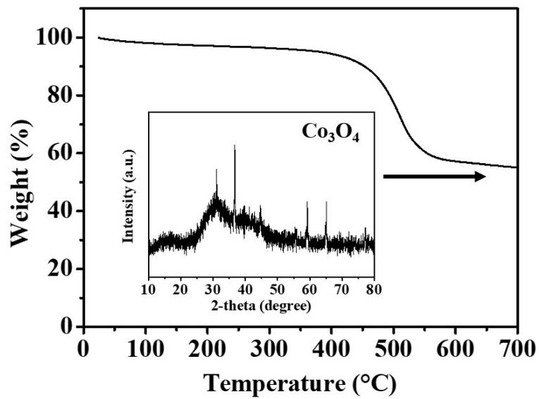
**Fig. S3** TGA curve of  $\text{CoF}_2/\text{MWCNTs}$  nanocomposites.
