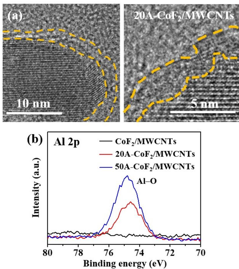
**Fig. S11** (a) HR-TEM images of 20A-CoF<sub>2</sub>/MWCNTs. (b) XPS spectrum of Al 2p of 20A- and 50A-CoF<sub>2</sub>/MWCNTs.
