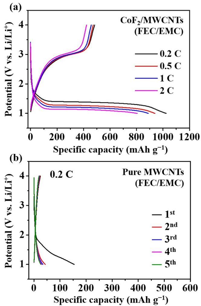
**Fig. S7** Voltage profiles of (a) CoF<sub>2</sub>/MWCNTs with FEC/EMC at the first cycle with various C-rates (0.2, 0.5, 1, and 2 C) and (b) pure MWCNTs. The specific capacities of pure MWCNTs are calculated based on the target mass of MWCNTs (30 wt%).
