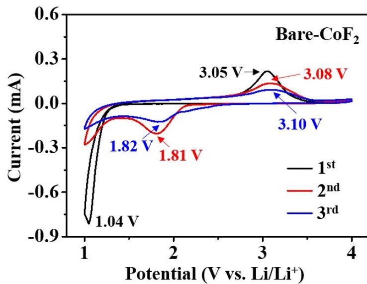
**Fig. S4** CV curves of bare-CoF<sub>2</sub> measured at a scan rate of 0.1 mV s<sup>-1</sup>.
