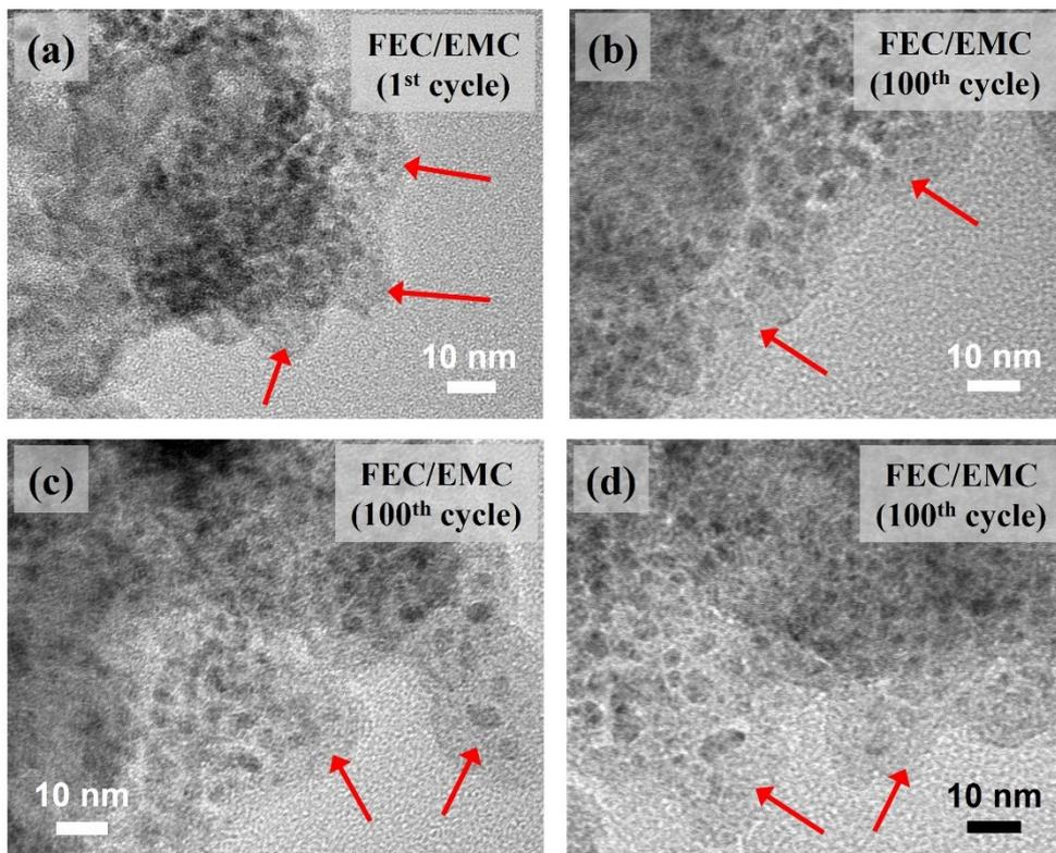
**Fig. S8** TEM images of CoF<sub>2</sub>/MWCNTs cycled in FEC/EMC electrolyte: (a) After the 1<sup>st</sup> cycle and (b–d) after the 100<sup>th</sup> cycle at 0.5 C.
