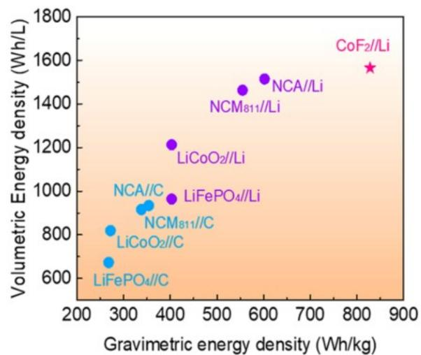
**Fig. S1** Comparison of theoretically achievable energy densities (maximal values) for CoF<sub>2</sub>-Li battery, commercial Li-ion batteries, and Li-metal batteries using commercial cathodes. Reproduced with permission from Ref. 23. Copyright (2021) ACS Nano.
