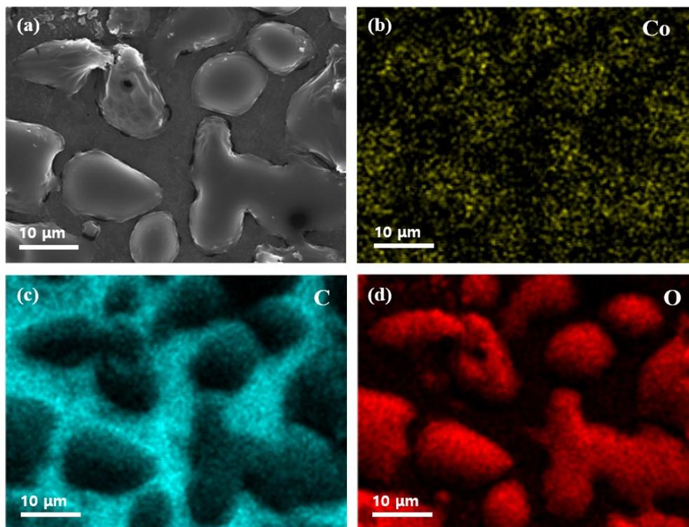
**Fig. S9** Post-mortem analysis of clogged parts of the separator after the 100<sup>th</sup> cycle (electrode: CoF<sub>2</sub>/MWCNTs) in EC/DMC electrolyte: (a) SEM image and EDS elemental mapping of (b) cobalt, (c) carbon, and (d) oxygen.
