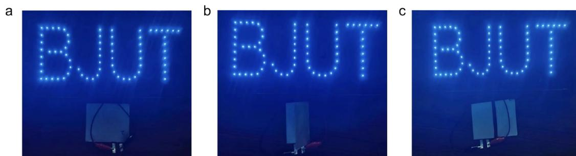
**Fig. S17** The optical photographs for the LLOs/PPS-PE-LB/Li soft package battery that lit up a logo at a, normal, b, wrinkled and c, cutting states.
