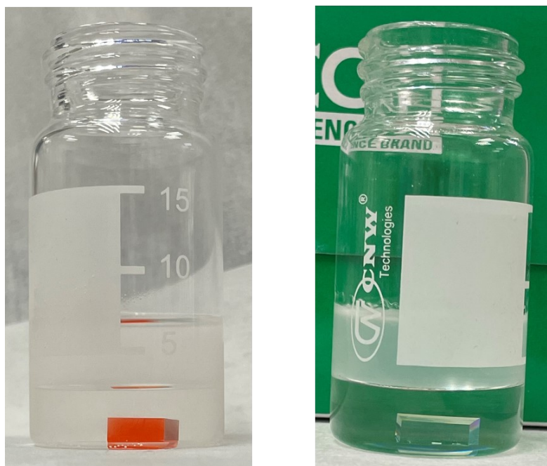
Fig.S1 LT-MAPbBr 3 single crystal in the left bottle and LT-MAPbCl 3 single crystal in the right bottle
