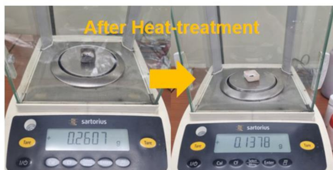
Fig. S12. (a) XRD patterns of PAH/NiFeSe, PGH/NiFeSe, and b-NiFeSe after heat-treatment under the same conditions as those used for TGA and (b) weight change of b-NiFeSe before and after heat-treatment.
