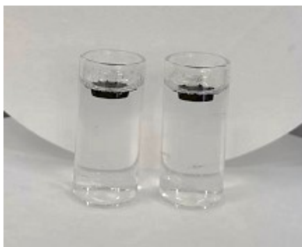
Figure S15 The digital image of rGO hydrogel prepared by hydrothermal method.
